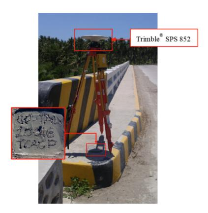
Figure 34. GNSS base set-up, Trimble® SPS 852, at UP-TAL, located at the approach of Talisay Bridge in Brgy. Pagsangahan, Municipality of San Francisco, Quezon
