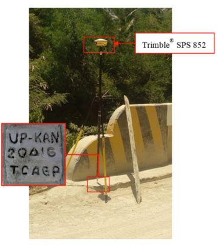
Figure 33. GNSS base set-up, Trimble® SPS 852, at UP-KAN, located at the approach of Kanguinsa Bridge in Brgy. Silongin, Municipality of San Francisco, Quezon
