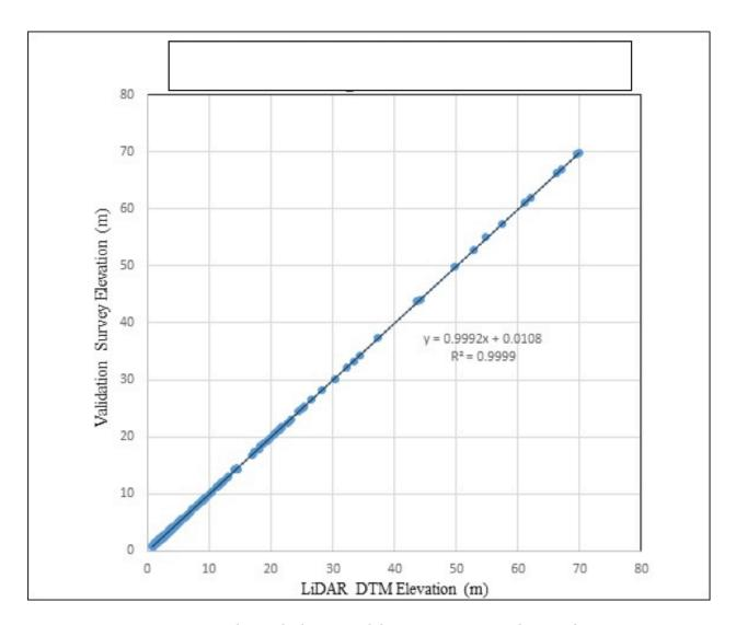
Figure 21. Correlation plot between validation survey points and LiDAR data
