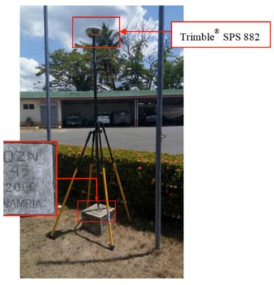
Figure 28. GNSS base set-up, Trimble® SPS 882, at QZN-43, located inside the DPWH compound in Brgy. Matandang Sabang Silangan, Municipality of Catanauan, Quezon
