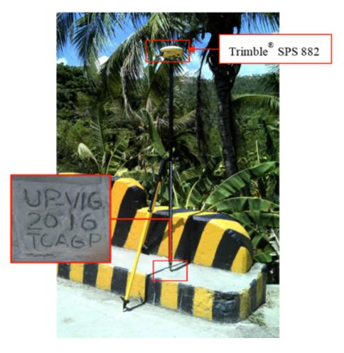
Figure 35. GNSS base set-up, Trimble® SPS 882, at UP-VIG, located at the approach of Vigo Bridge in Brgy. Vigo Central, Municipality of San Francisco, Quezon
