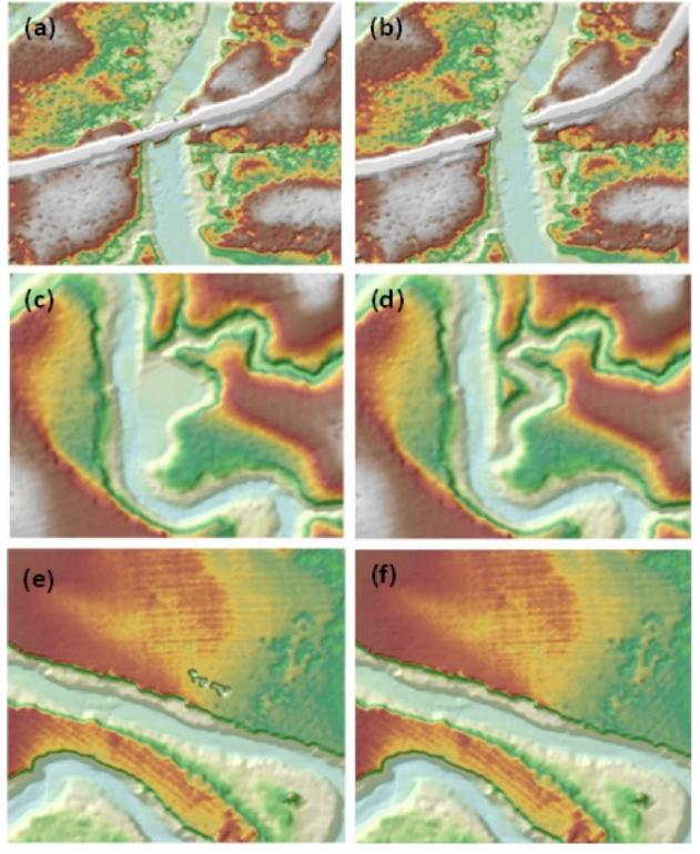
Figure 17. Portions in the DTM of Silongin Floodplain—a bridge before (a) and after (b) manual editing; a point bar before (c) and after (d) data retrieval; and a pit before (e) and after (f) manual editing
