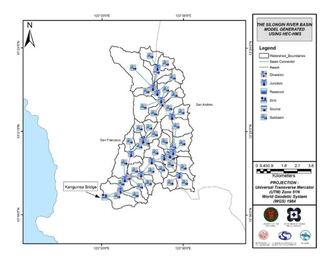
Figure 57. The Silongin River Basin model domain generated by HEC-HMS
