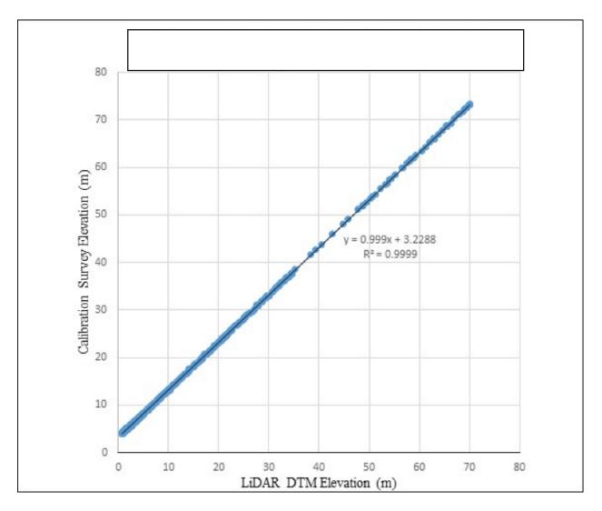
Figure 20. Correlation plot between calibration survey points and LiDAR data
