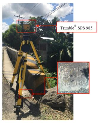
Figure 30. GNSS base set-up, Trimble® SPS 985, at QZ-415, located at the approach of Pansol Bridge in Brgy. Pansol, Municipality of Lopez, Quezon
