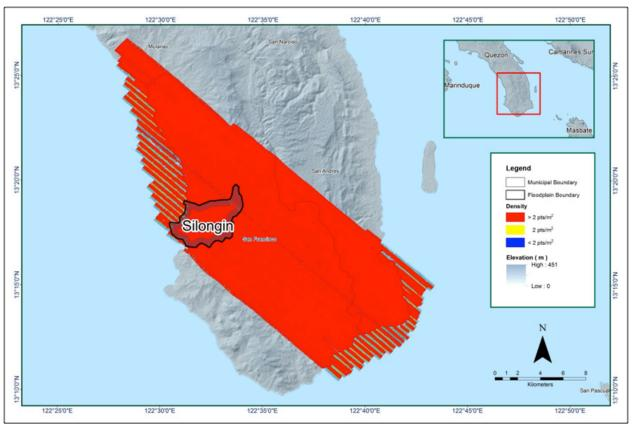
Figure 11. Pulse density map of merged LiDAR data for Silongin Floodplain
