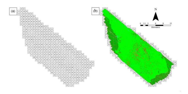
Figure 14. Tiles for Silongin Floodplain (a) and classification results (b) in TerraScan
