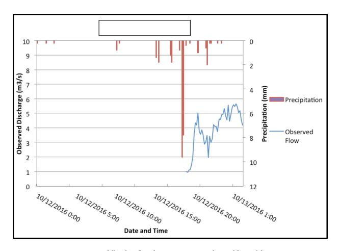
Figure 50. Rainfall and outflow data at Kanguinsa Bridge used for modeling
