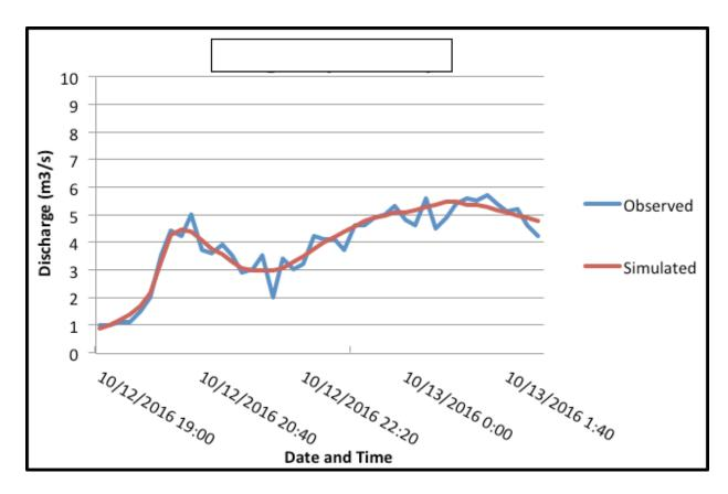
Figure 62. Outflow hydrograph of Silongin produced by the HEC-HMS model compared with observed outflow
