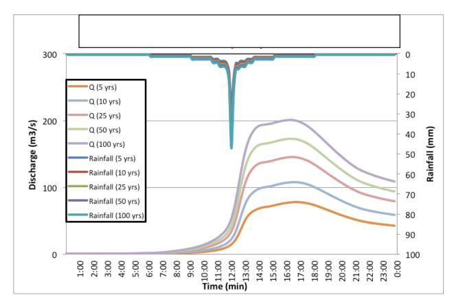
Figure 63. Outflow hydrograph at Silongin Station generated using Romblon RIDF simulated in HEC-HMS
