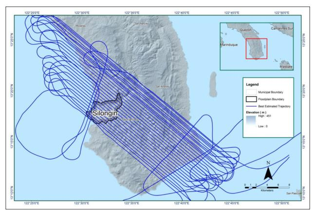
Figure 8. Best estimated trajectory of the LiDAR missions conducted over Silongin Floodplain
