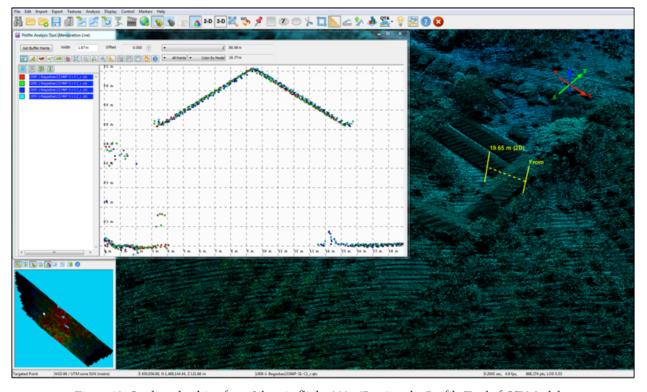
Figure 13. Quality checking for a Silongin flight 23346P using the Profile Tool of QT Modeler
