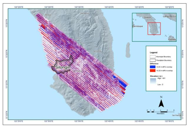
Figure 12. Elevation difference map between flight lines for Silongin Floodplain
