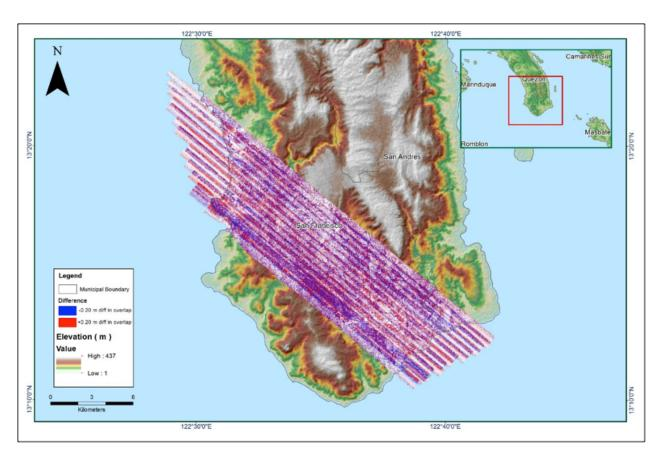
Figure 1.1.7. Elevation difference between flight lines
