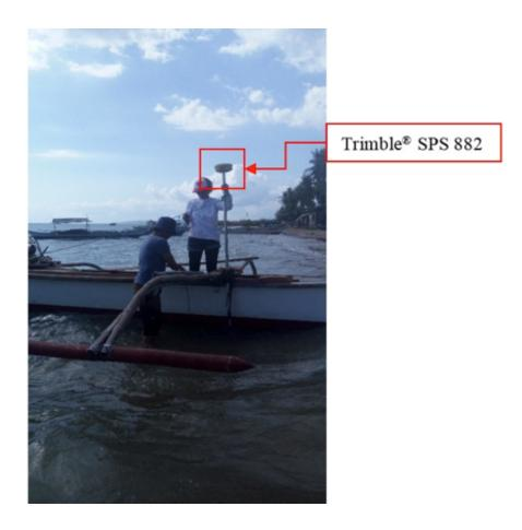
Figure 43. Bathymetry by boat set up for Silongin River survey
