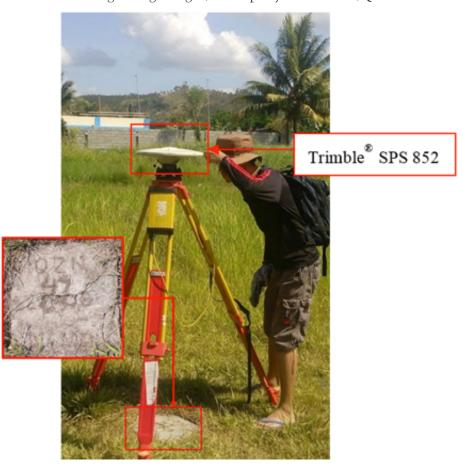
Figure 29. GNSS base set-up, Trimble® SPS 852, at QZN-47, located at the back of the Principal's Office of Mulanay Elementary School in Barangay II, Municipality of Mulanay, Quezon
