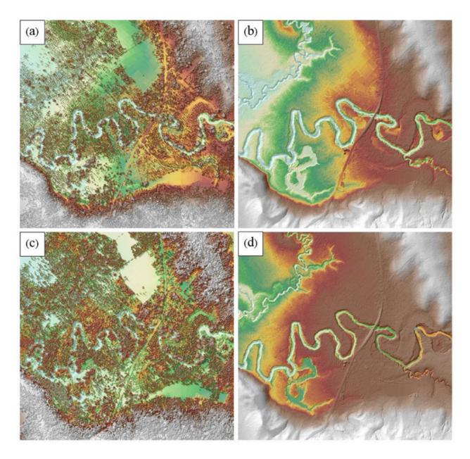
Figure 16. The production of last return DSM (a) and DTM (b); first return DSM (c) and secondary DTM (d) in some portion of Silongin Floodplain.
