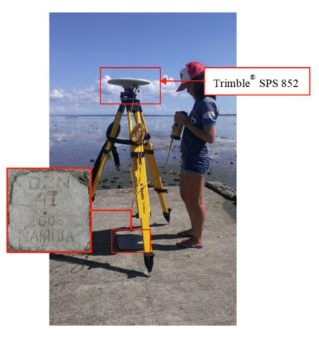
Figure 31. GNSS base set-up, Trimble® SPS 852, at QZN-41, located in front of Brgy. Sabang basketball court found in Calauag Port, Barangay I, Municipality of Calauag, Quezon
