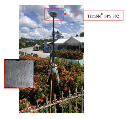
Figure 27. GNSS base set-up, Trimble® SPS 882, at QZN-40, located inside a triangular plant area found at the center of a triangular island in Brgy. San Jose, Municipality of Gen. Luna, Quezon
