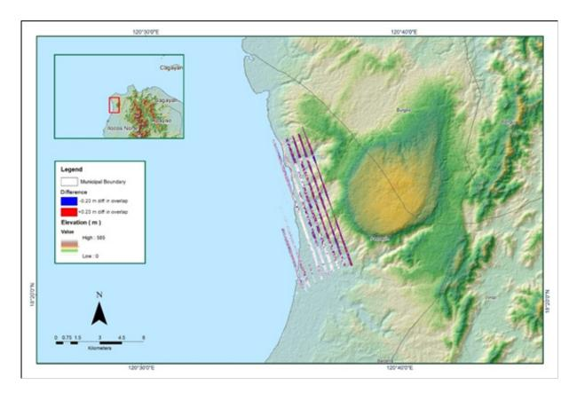
Figure A-8.28 Elevation difference between flight lines
