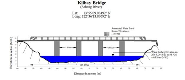
Figure 34. Kilbay Bridge cross-section diagram.
