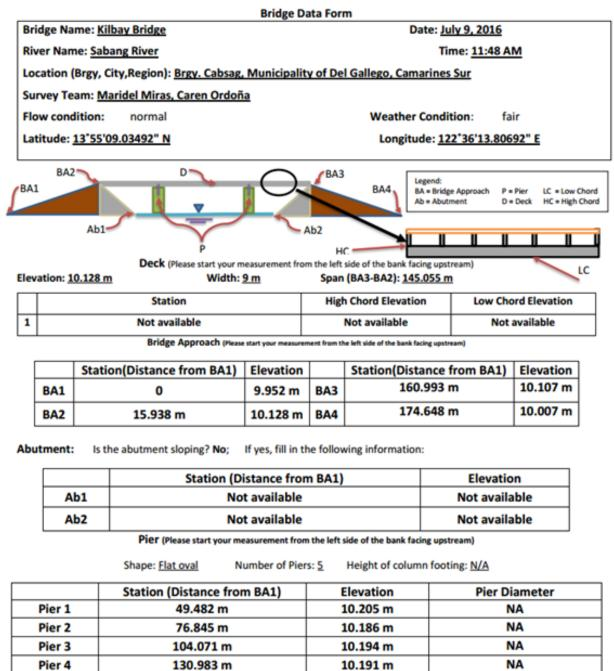
NOTE: Use the center of the pier as reference to its station
