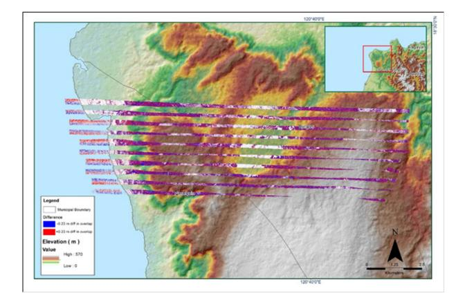
Figure A-8.14 Elevation difference between flight lines
