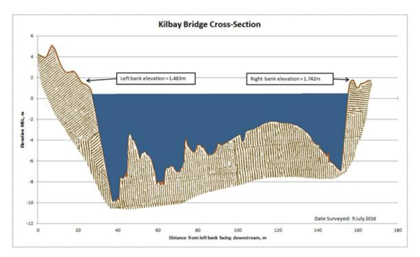
Figure 44. Cross-Section Plot of Kilbay Bridge.
