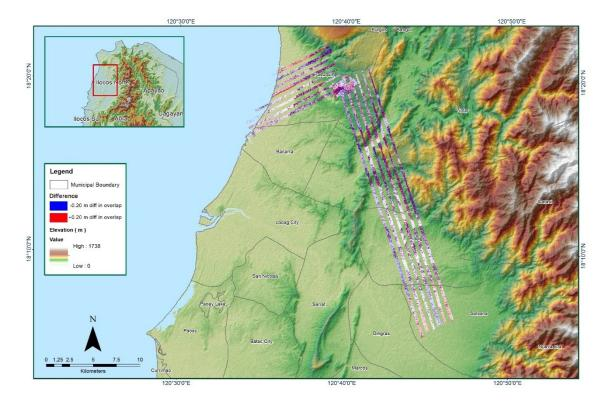
Figure A-8.49 Elevation difference between flight lines
