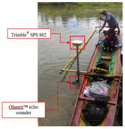
Figure 40. Bathymetric survey using Ohmex<sup>™</sup> single beam echo sounder in Sabang River.
