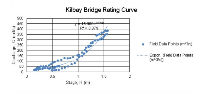
Figure 45. Rating Curve at Kilbay Bridge, Del Gallego, Camarines Sur.
