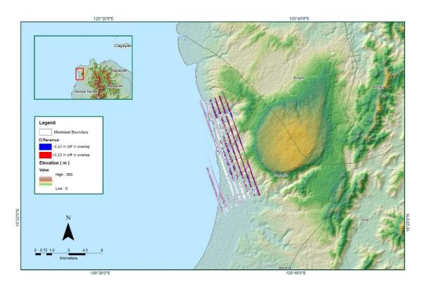
Figure A-8.42 Elevation difference between flight lines
