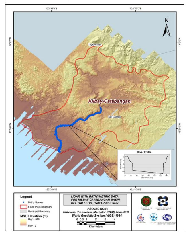
Figure 23. Map of Kilbay-Catabangan Flood Plain with bathymetric survey points shown in blue.
