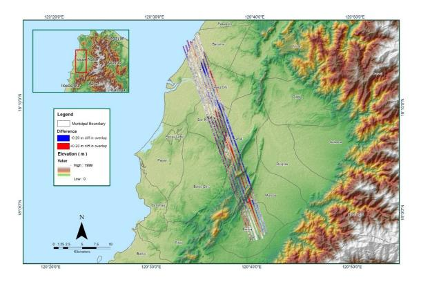
Figure A-8.81 Elevation difference between flight lines
