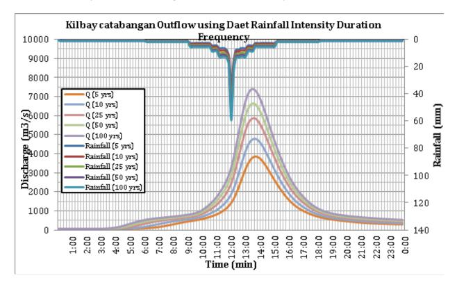
Figure 57. Outflow hydrograph at Kilbay generated using Daet RIDF simulated in HEC-HMS.
