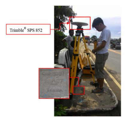
Figure 30. GNSS receiver setup, Trimble<sup>®</sup> SPS 852, at CMN-3087, located at the approach of Labo Bridge in Brgy. Bakiad, Municipality of Labo, Camarines Norte.
