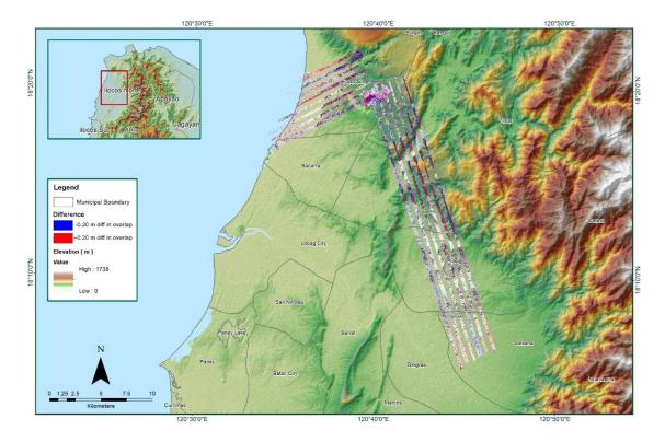
Figure A-8.35 Elevation difference between flight lines
