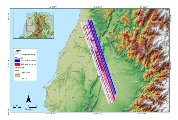
Figure A-8.60 Elevation difference between flight lines
