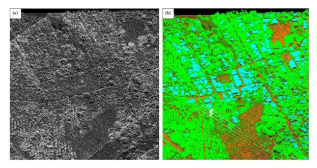
Figure 14. Point cloud before (a) and after (b) classification.
