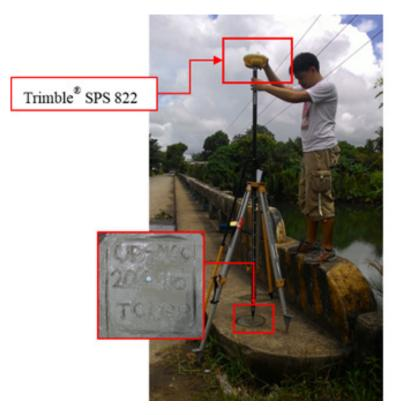
Figure 31. GNSS receiver setup, Trimble<sup>®</sup> SPS 822, at UP-MOC, located at the approach of Mocong Bridge in Brgy. Mocong, Municipality of Basud, Camarines Norte.
