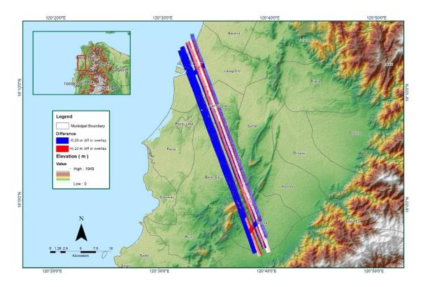
Figure A-8.88 Elevation difference between flight lines
