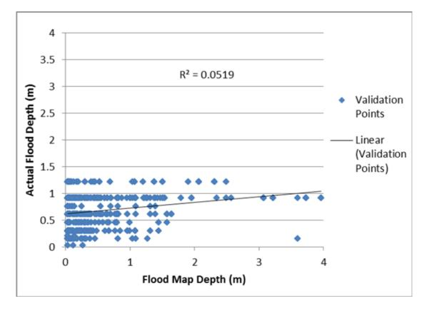
Figure 102. Flood Map depth versus Actual Flood Depth.
