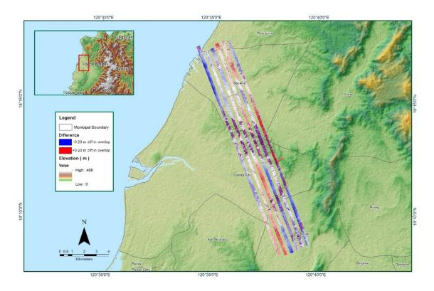
Figure A-8.67 Elevation difference between flight lines
