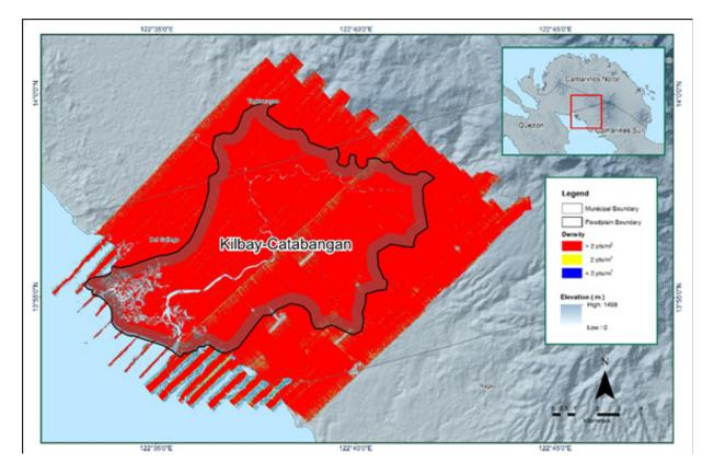
Figure 10. Density map of merged LiDAR data for Kilbay-Catabangan floodplain.
