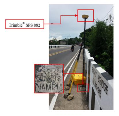
Figure 29. GNSS receiver setup, Trimble® SPS 882, at CS-398, located at the approach of Ragay Bridge in Brgy. Pangitayan, Municipality of Ragay, Camarines Sur. Hazard Mapping of the Philippines Using LIDAR (Phil-LIDAR 1)
