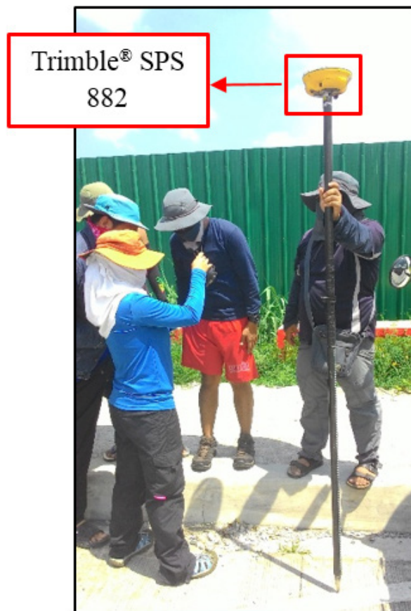
Figure 37. Bridge As-Built Survey using PPK Technique.
