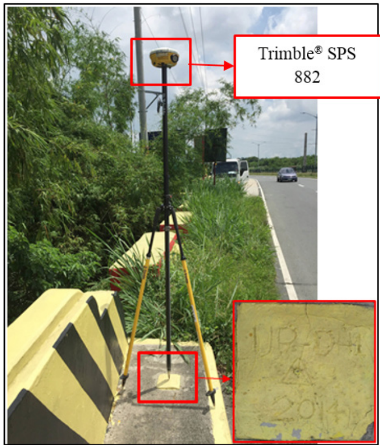
Figure 34. Trimble® SPS 882 setup at UP-DH1 located in Daang Hari Bridge, Brgy. Anabu II-A, Municipality of Imus, Cavite
