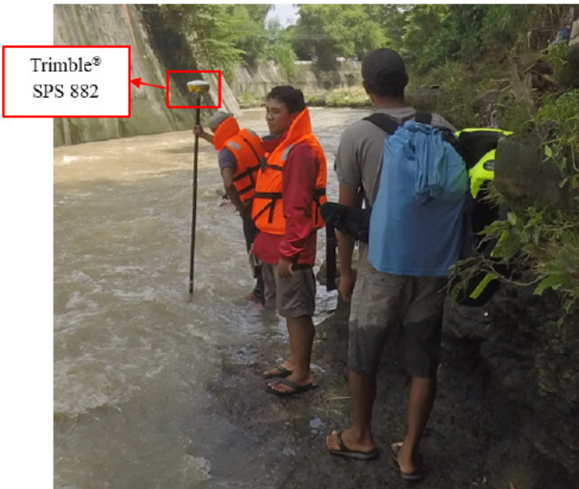
Figure 45. Manual Bathymetric Survey in Imus River in Brgy. Anabu, Imus
