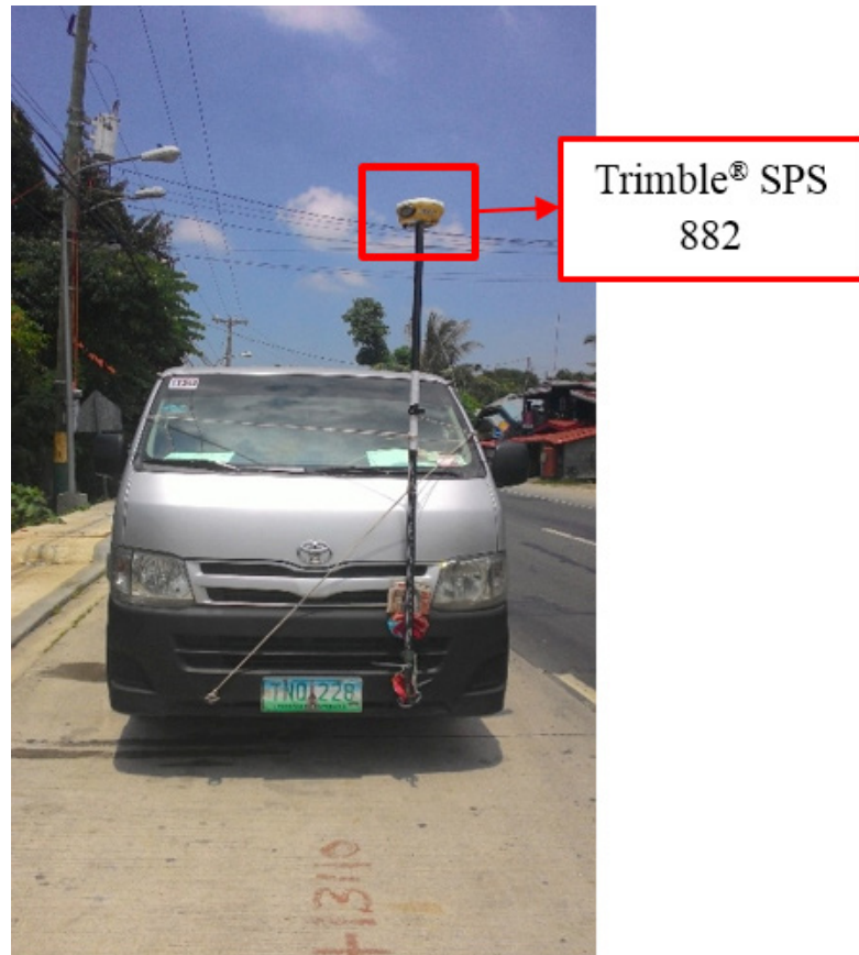
Figure 42. Validation points acquisition survey set up for Imus River Basin
