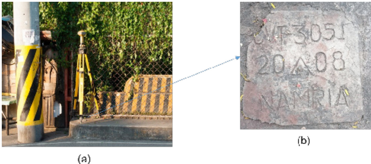
Figure 4. GPS set-up over CVT-3051 in a concrete bridge leading to Manggahan, 70 m SE of Jetti Gas Station and about 250 m from Gen. Trias Poblacion (a) and NAMRIA reference point CVT-3051 (b) as recovered by the field team.
