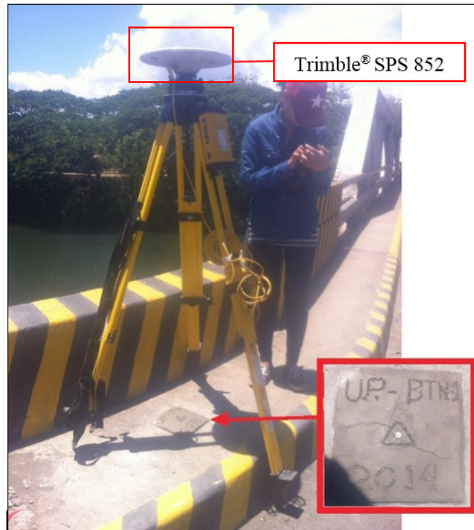
Figure 34. GNSS base receiver, Trimble® SPS 852, set-up at UP-BTN at Bantilan Bridge, Brgy. Manggalang Banitilan, Sariaya, Quezon
