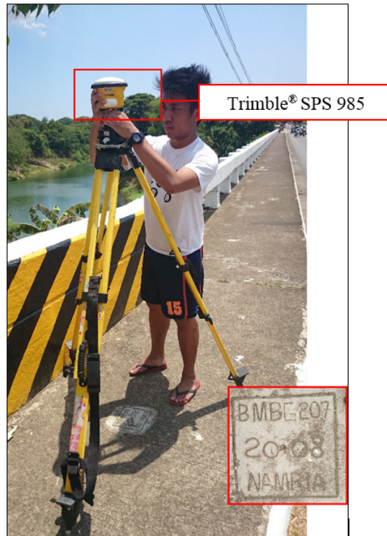
Figure 31. GNSS receiver, Trimble® SPS 985, set-up at BG-207 at Palico Bridge, Brgy. Luntal, Nasugbu, Batangas
