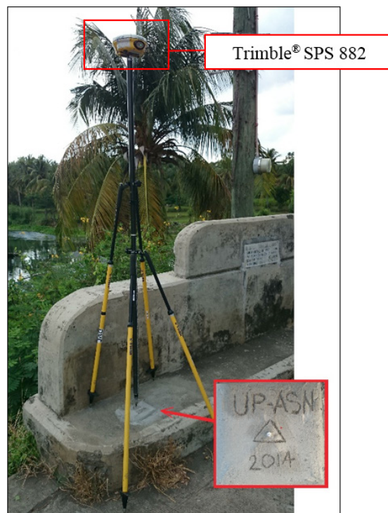
Figure 33. GNSS receiver, Trimble® SPS 882, set-up at UP-ASN at San Nicholas Bridge, Brgy. Poblacion, San Nicholas, Batangas
