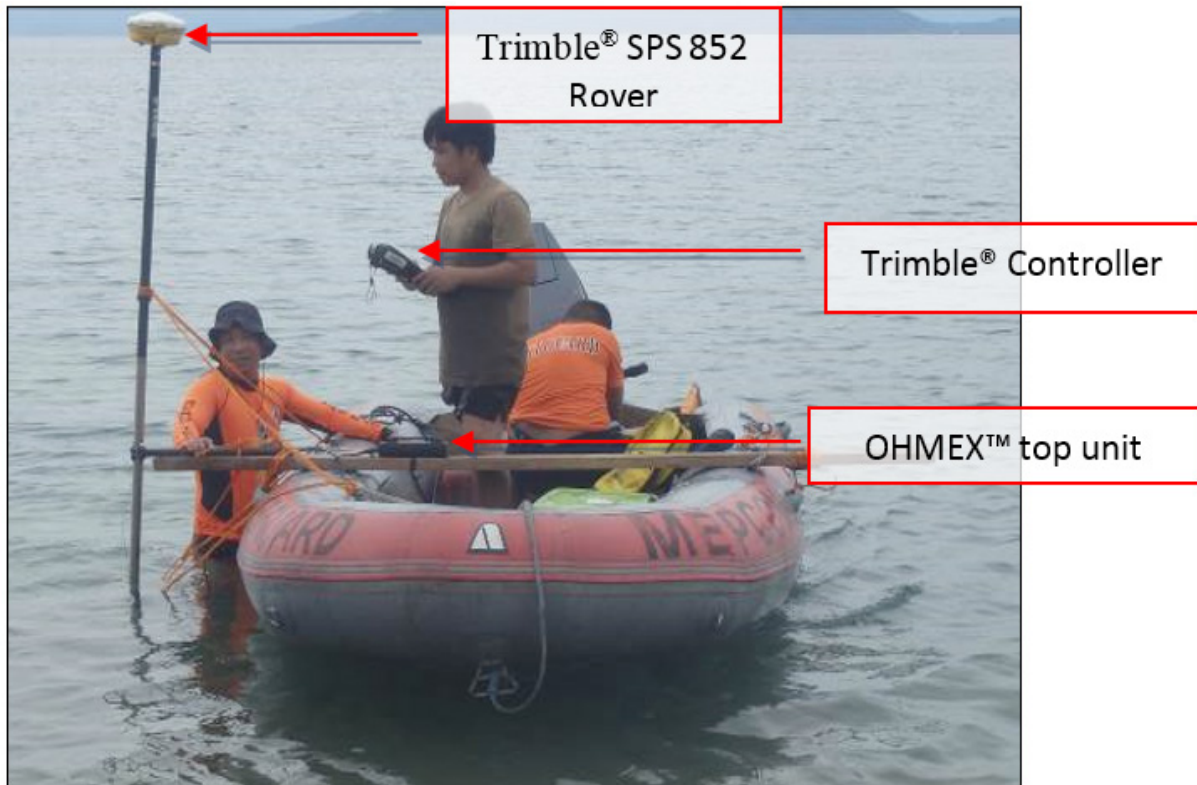
Figure 46. OHMEX™ single-beam echo sounder set-up on a rubber for the Calumpang River bathymetric survey
