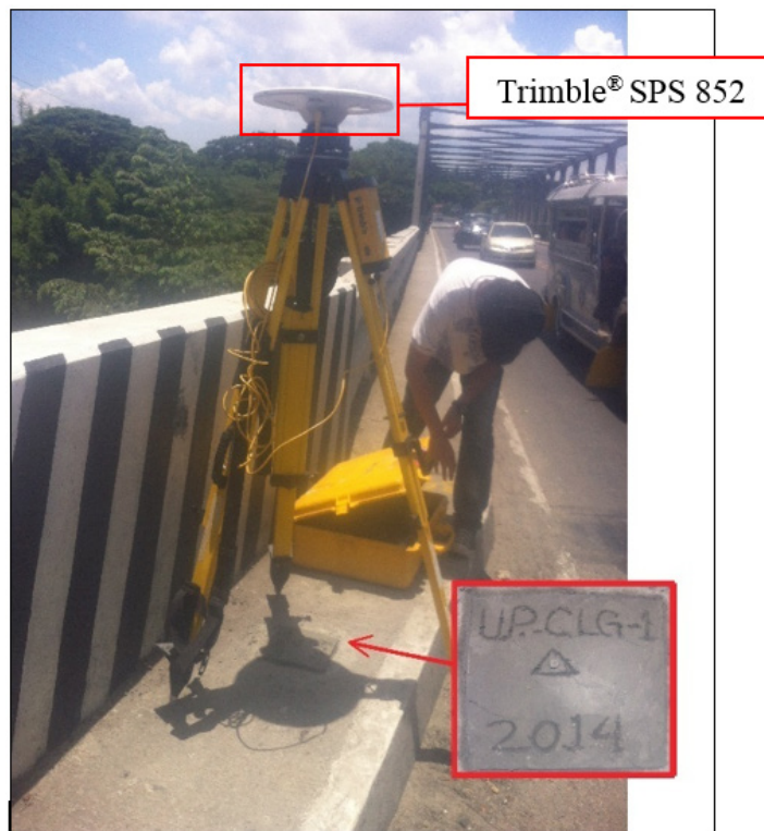
Figure 35. GNSS base receiver, Trimble® SPS 852, set-up at UP-CLG1 in Calumpang Bridge, Brgy. Cumintang Ibaba, Batangas City, Batangas
