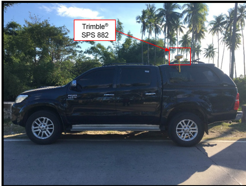
Figure 44. Ground Validation set up in Calumpang Survey
