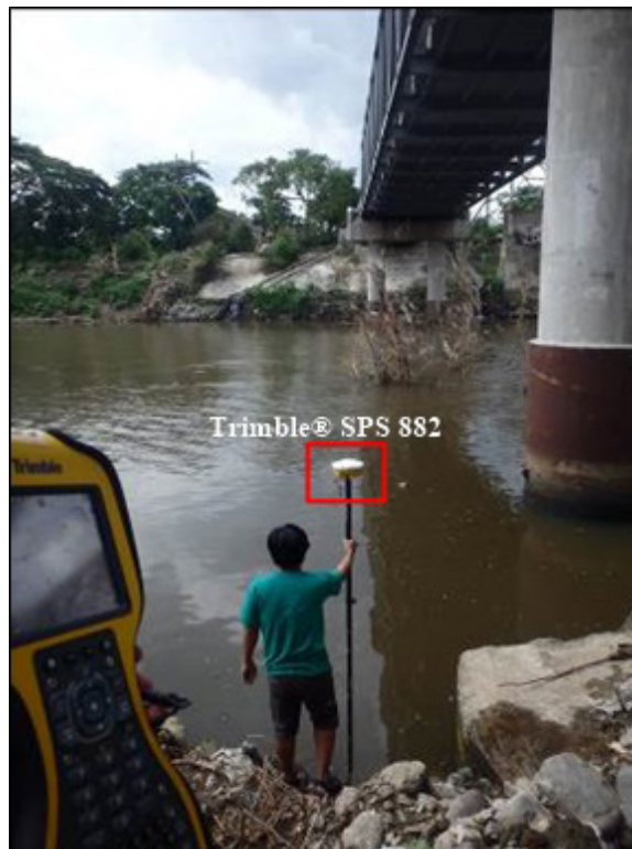
Figure 42. Determination of water surface elevation at the river banks of the Bridge of Promise
