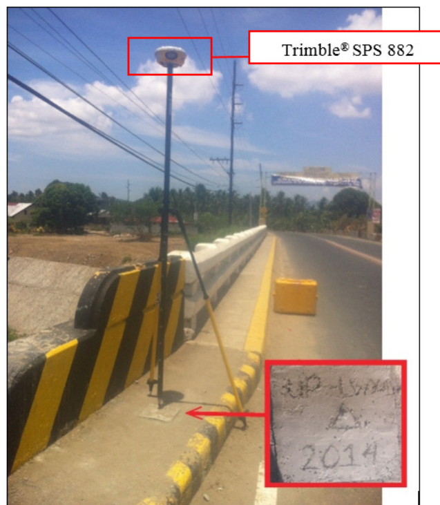
Figure 37. GNSS receiver, Trimble® SPS 882, set-up at UP-LWY1 at Lawaye Bridge, Brgy. Calitcalit-Mabalanoy, San Juan, Batangas
