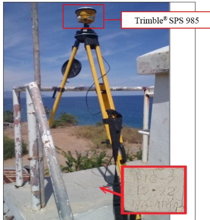
Figure 32. GNSS receiver, Trimble® SPS 985, set-up at BTG-7 in Dela Paz Lighthouse in Brgy. Dela Paz, Batangas City, Batangas
