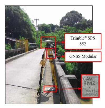
Figure 38. GPS set-up of Trimble<sup>®</sup> SPS 852 at CAV-BM 2, located at the Cañas Bridge in Barangay Tapia, Municipality of General Trias, Cavite
