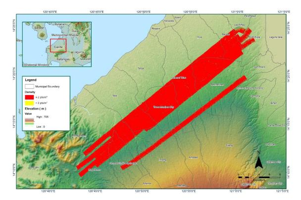
Figure A-8.45. Density map of merged LiDAR data
