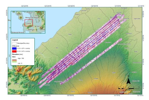
Figure A-8.46. Elevation difference between flight line
