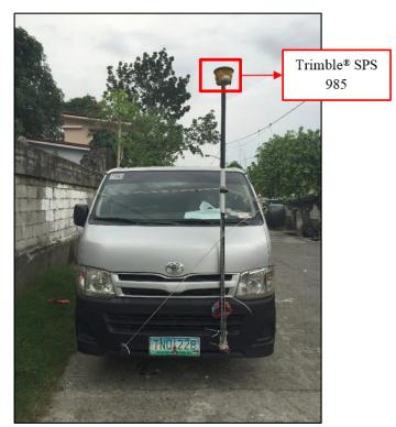
Figure 44. Validation points acquisition set-up for the Binabang-Molino River Basin
