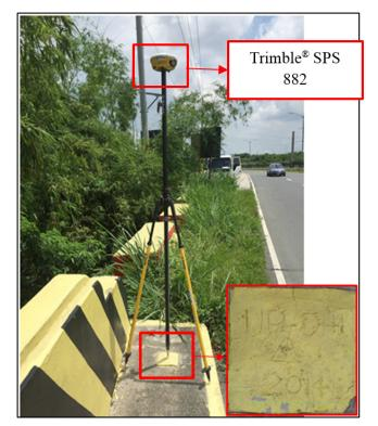
Figure 35. Trimble<sup>®</sup> SPS 882 set-up at UP-DH1, located at the Daang Hari Bridge in Barangay Anabu II-A, Municipality of Imus, Cavite
