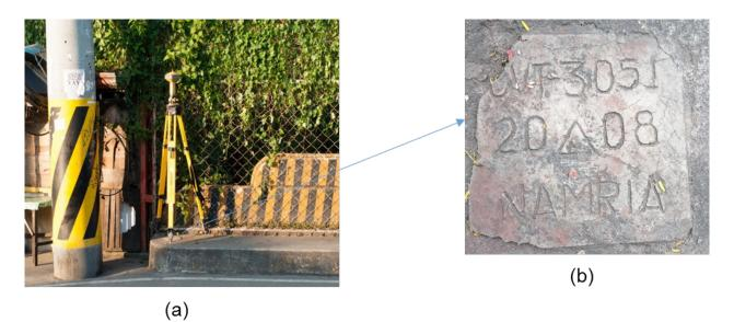
Figure 4. (a) GPS set-up over CVT-3051 in a concrete bridge leading to Manggahan, 70 m SE of Jetti Gas Station and about 250 m from Gen. Trias Poblacion; and (b) NAMRIA reference point CVT-3051, as recovered by the field team
