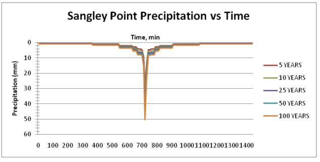
Figure 54. Synthetic storm generated from a 24-hour period rainfall, for various return periods
