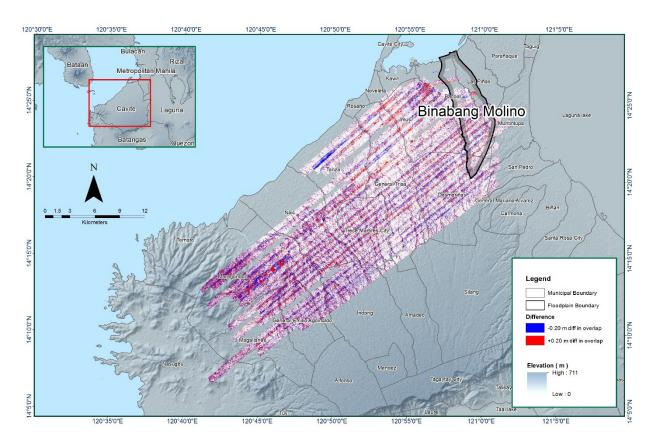
Figure 16. Elevation difference map between flight lines for the Binabang-Molino floodplain
