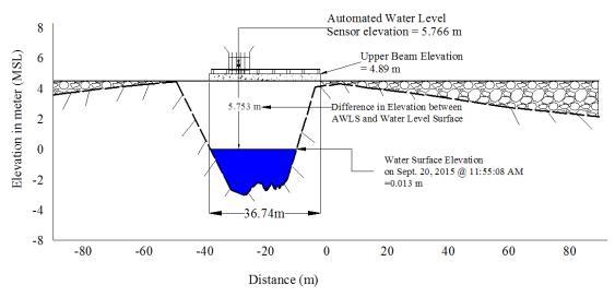
Figure 41. Zapote Bridge cross-sectional diagram
