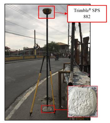
Figure 37. Trimble<sup>®</sup> SPS 882 set-up at UP-ZE, located at the Zapote Bridge in Barangay Zapote, Bacoor City, Cavite
