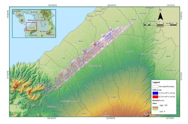
FigureA-8.7. Elevation difference between flight lines
