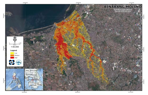
Figure 65. 100-year flood hazard map for the Binabang-Molino floodplain
