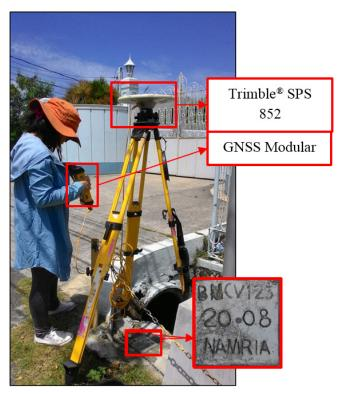
Figure 34. GPS set-up of Trimble<sup>®</sup> SPS 852 at CV-123, located in front of the Iglesia ni Cristo Chapel, Municipality of Naic, Cavite
