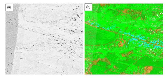
Figure 19. Point cloud (a) before and (b) after classification
