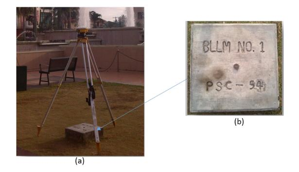
Figure 5. (a) GPS set-up over CVT-194 (BLLM NO.1 PSC-94) near the Municipal Hall of Gen. Trias, Cavite; and (b) NAMRIA reference point CVT-194, as recovered by the field team
