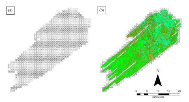
Figure 18. (a) Tiles for Binabang-Molino floodplain, and (b) classification results in TerraScan
