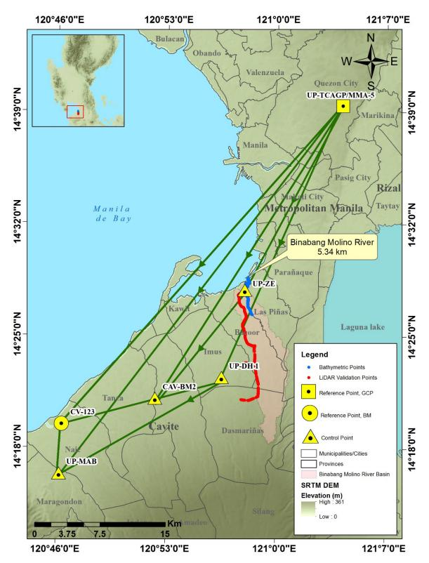
Figure 31. Extent of the bathymetric survey (in blue line) in the Binabang-Molino River and the LiDAR data validation survey (in red)
