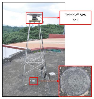
Figure 33. Trimble<sup>®</sup> SPS 852 set-up at MMA-5, located at the Melchor Hall, University of the Philippines, Diliman, Quezon City
