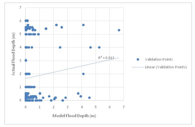
Figure 87. Model flood depth vs. actual flood depth
