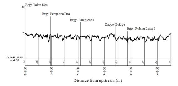
Figure 48. Riverbed profile of the Binabang-Molino River
