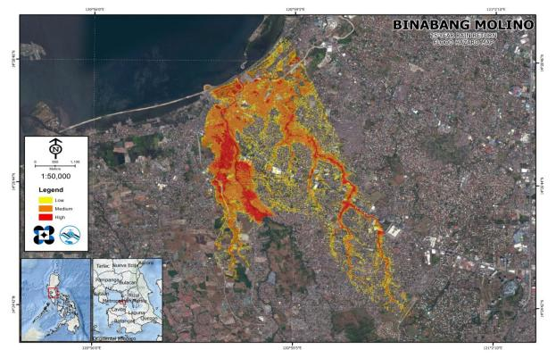
Figure 67. 25-year flood hazard map for the Binabang-Molino floodplain
