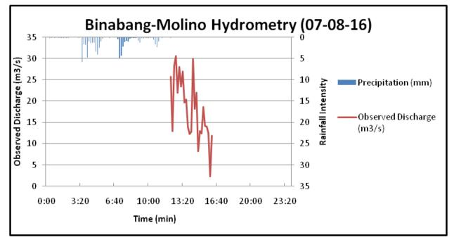
Figure 52. Rainfall and outflow data at Binabang-Molino, which were used for modeling
