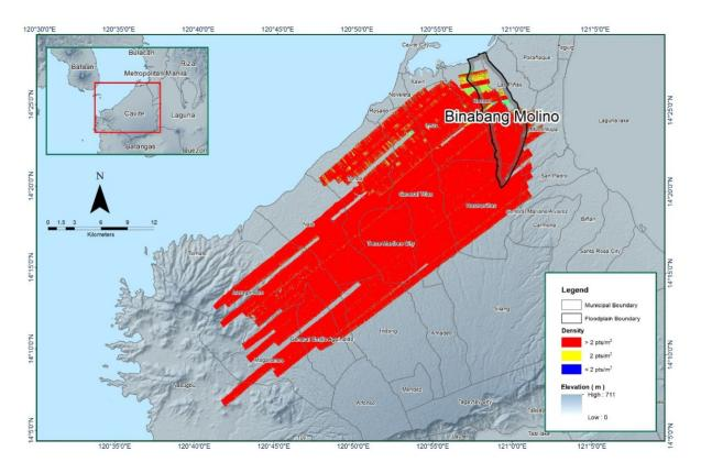
Figure 15. Pulse density map of merged LiDAR data for the Binabang-Molino floodplain
