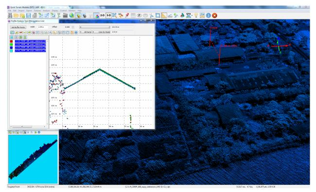
Figure 17. Quality checking for Binabang-Molino Flight 3309P, using the Profile Tool of QT Modeler
