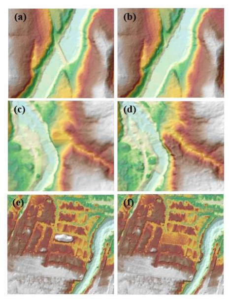
Figure 23. Portions in the DTM of the Binabang-Molino floodplain – a bridge (a) before and (b) after manual editing; a ridge (c) before and (d) after data retrieval; and a building (e) before and (f) after manual editing
