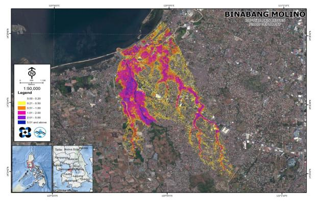
Figure 66. 100-year flow depth map for the Binabang-Molino floodplain
