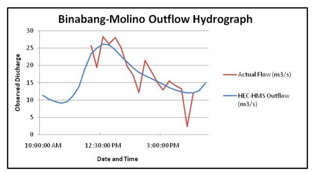
Figure 62. Outflow hydrograph of the Binabang-Molino produced by the HEC-HMS model, compared with observed outflow
