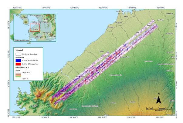
Figure A-8.32. Elevation difference between flight lines
