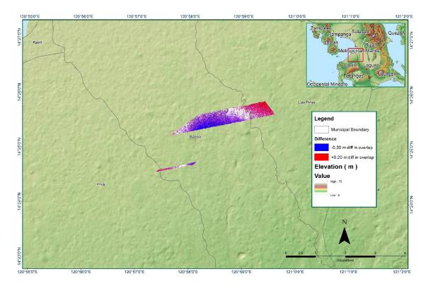
Figure A-8.25. Elevation difference between flight lines
