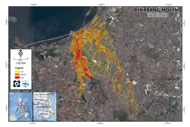
Figure 69. 5-year flood hazard map for the Binabang-Molino floodplain
