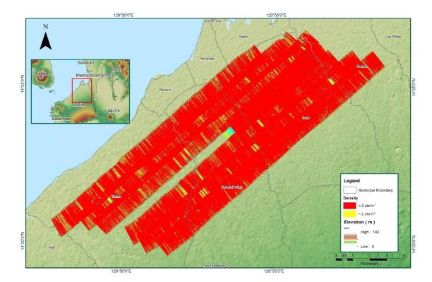
Figure A-8.52. Density map of merged LiDAR data
