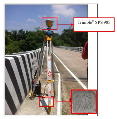
Figure 36. Trimble<sup>®</sup> SPS 985 set-up at UP-MAB, located at the approach of the Mabacao Bridge in Barangay Bucal IV B, Municipality of Maragondon, Cavite
