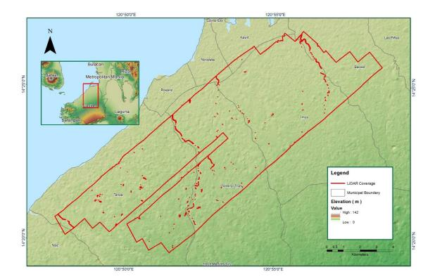
Figure A-8.50. Coverage of LiDAR data
