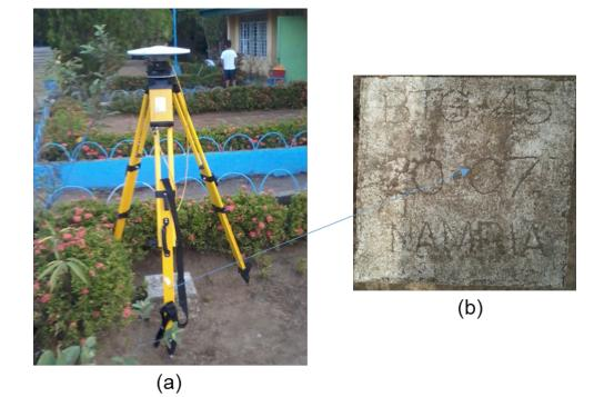
Figure 6. (a) GPS set-up over BTG-45 inside Santiago De Guzman Elementary School in Barangay Malibu, Tuy, Batangas Province; and (b) NAMRIA reference point BTG-45, as recovered by the field team
