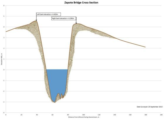
Figure 50. Cross-section plot of the Zapote Bridge
