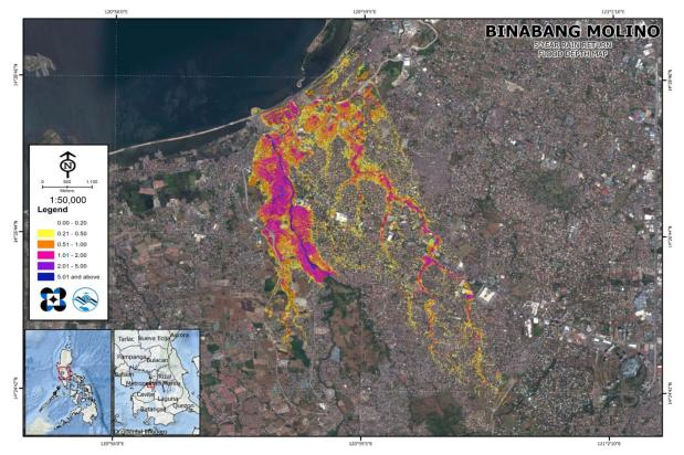
Figure 70. 5-year flow depth map for the Binabang-Molino floodplain
