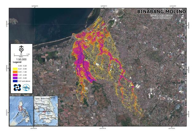
Figure 68. 25-year flow depth map for the Binabang-Molino floodplain
