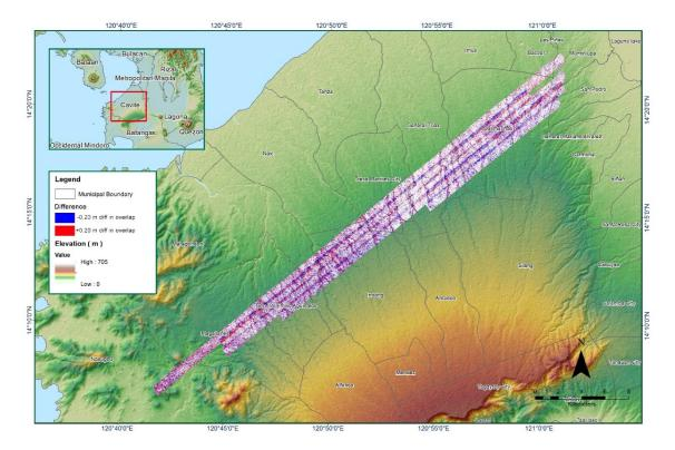
Figure A-8.39. Elevation difference between flight lines
