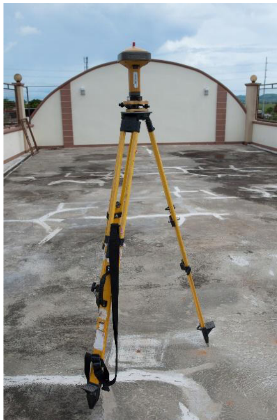
Figure 4. GPS set-up over BRS-1 as established in the rooftop of D' One Resort & Restaurant in Baras, Rizal.
