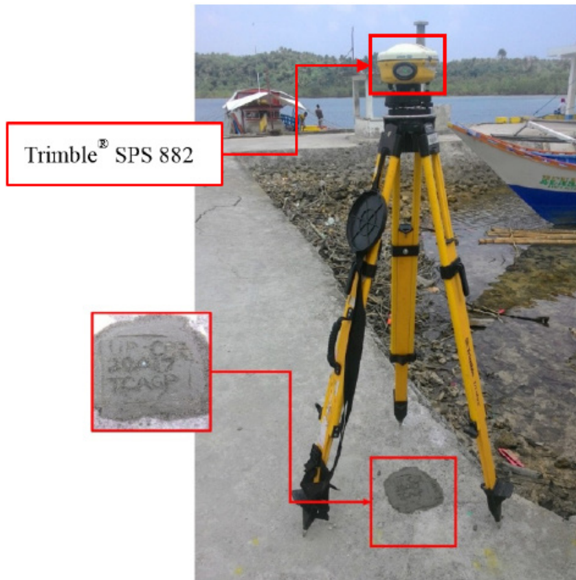
Figure 29. GNSS receiver setup, Trimble® SPS 882, at UP-CAR, located in Brgy. Carlagan. Municipality of Burdeos, Quezon
