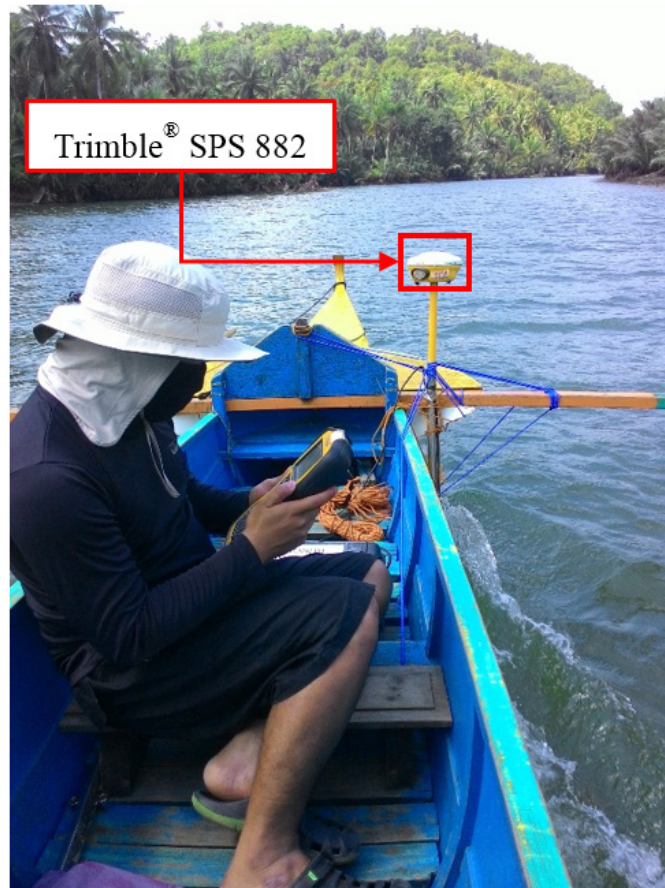
Figure 37. Bathymetric survey using Ohmex™ single beam echo sounder in Anibawan River
