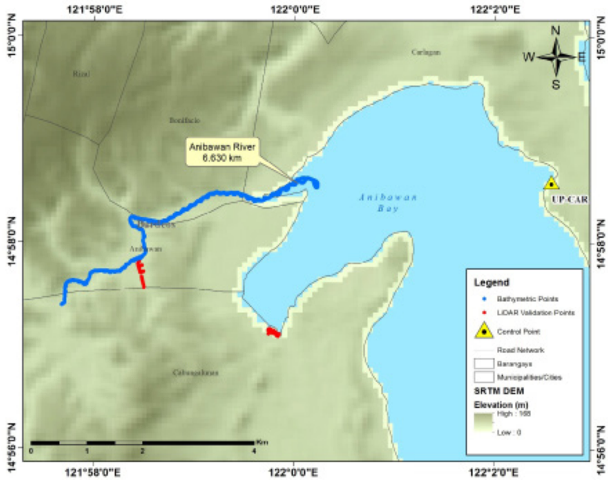
Figure 36. LiDAR validation points acquisition survey for Anibawan River Basin
