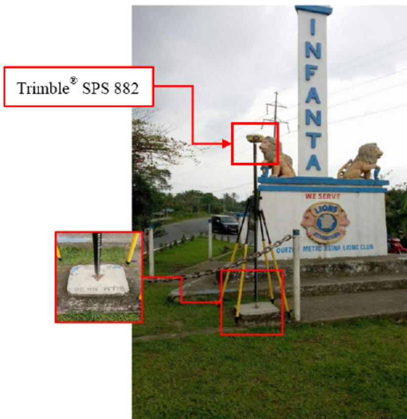
Figure 27. GNSS receiver setup, Trimble® SPS 882, at QZ-555, located in Brgy. Gumian, Municipality of Infanta, Quezon
