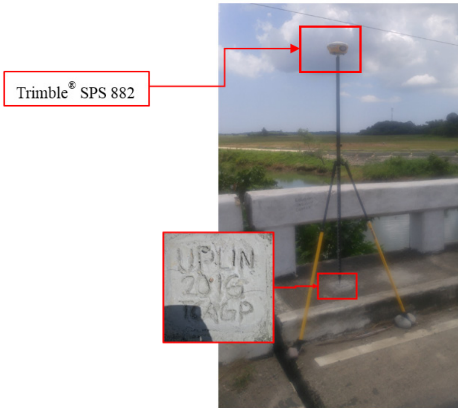
Figure 35. GNSS receiver setup, Trimble® SPS 882, at UP-LIN, located at the approach of Linao Bridge in Brgy. Bangag-Zingag, Municipality of Aparri, Cagayan
