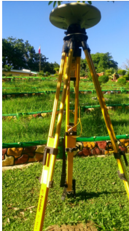
Figure 5. GPS set-up over CGY-110 located inside the compound of Pamplona Central School, Municipality of Pamplona.
