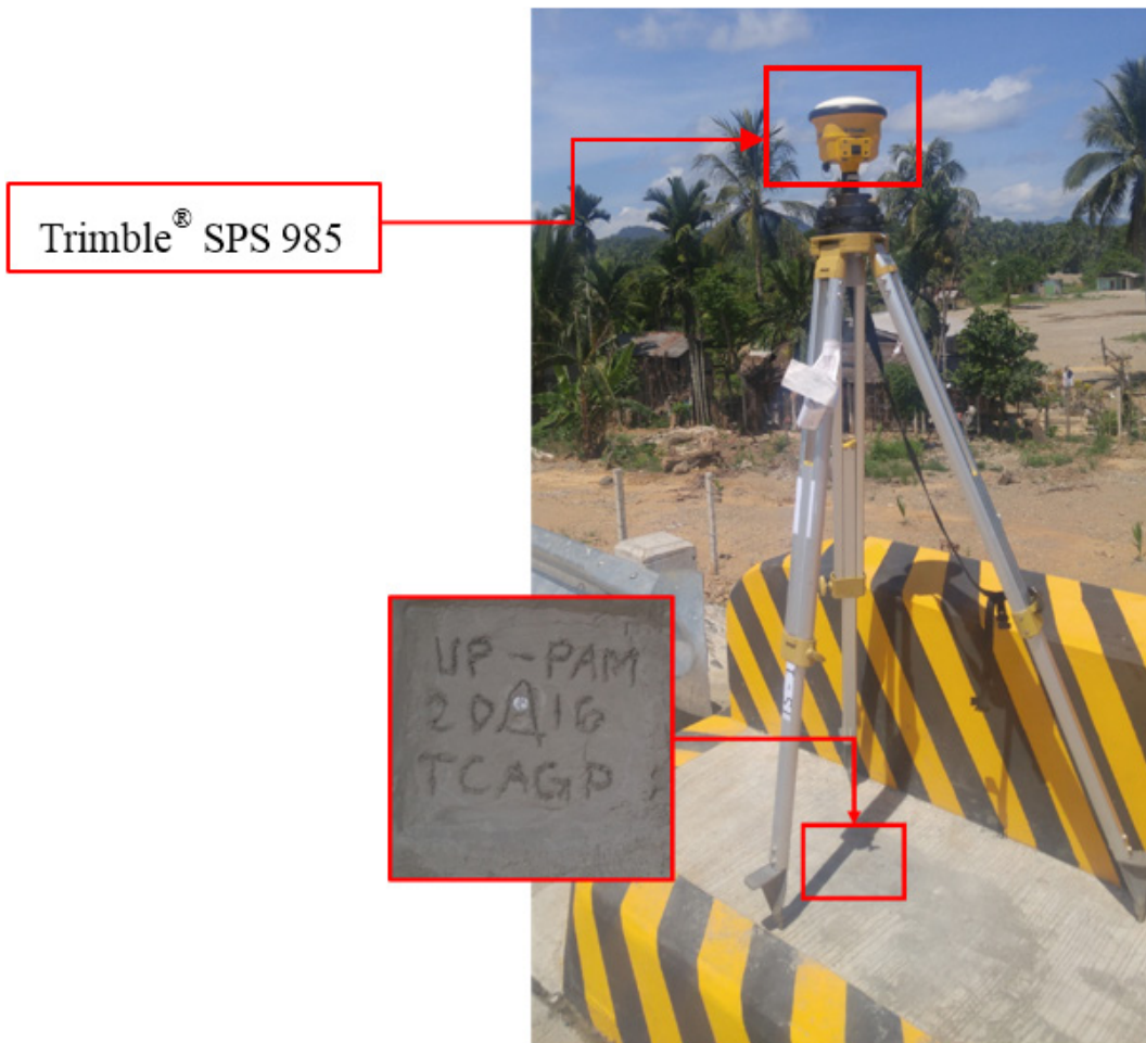
Figure 36. GNSS receiver setup, Trimble® SPS 985, at UP-PAM, located at the approach of New Pamplona Bridge in Brgy. Masi, Municipality of Pamplona, Cagayan
