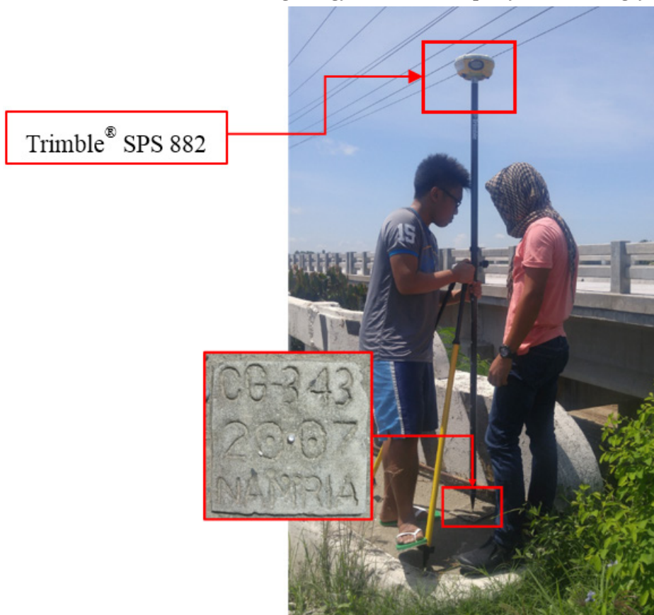
Figure 32. GNSS receiver setup, Trimble® SPS 882, at CG-343, located at the approach of Likban Bridge in Brgy. Libertad, Municipality of Abulug, Cagayan
