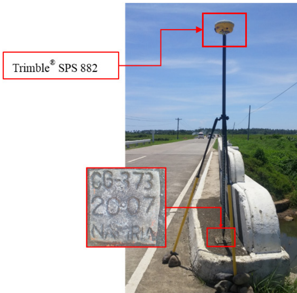
Figure 33. GNSS receiver setup, Trimble® SPS 882, at CG-373, located at the approach of Bangan Bridge in Brgy. Bangan, Municipality of Sanchez Mira, Cagayan
