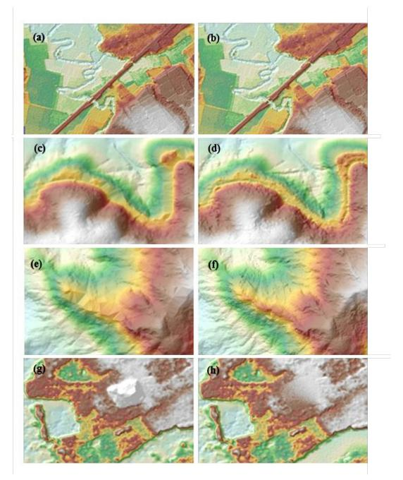
Figure 24. Portions in the DTM of the Linao floodplain – a road before (a) and after (b) manual editing; an irrigation before (c) and after (d) retrieval; interpolated ridge before (e) and after (f) object retrieval; and a building before (g) and after (h) manual editing.
