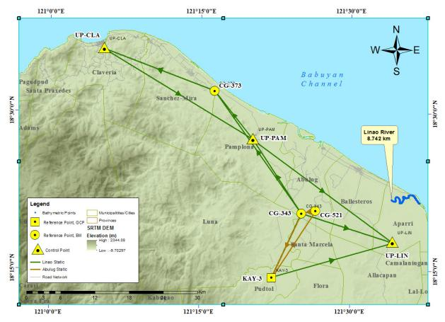
Figure 33. GNSS Network covering the Linao River
