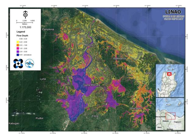
Figure 71. 5-year Flood Depth Map for the Linao Floodplain
