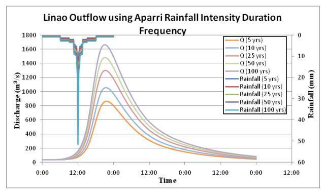
Figure 64. Outflow hydrograph at the Linao Station, generated using the Aparri RIDF simulated in HEC-HMS
