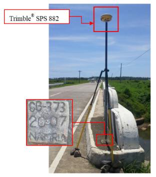
Figure 36. GNSS receiver set-up, Trimble<sup>®</sup> SPS 882, at CG-373, located at the approach of the Bangan Bridge in Barangay Bangan, Municipality of Sanchez Mira, Cagayan
