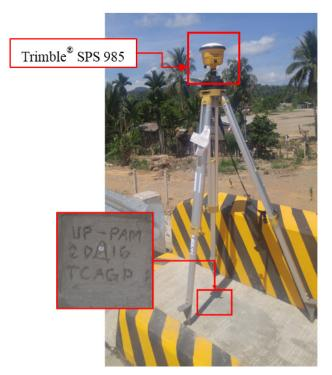
Figure 39. GNSS receiver set-up, Trimble<sup>®</sup> SPS 985, at UP-PAM, located at the approach of the New Pamplona Bridge in Barangay Masi, Municipality of Pamplona, Cagayan
