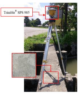
Figure 34. GNSS base set-up, Trimble<sup>®</sup> SPS 985, at KAY-3, situated on top of the flood gate near Pudtol Municipal Building in Barangay Imelda, Municipality of Pudtol, Cagayan
