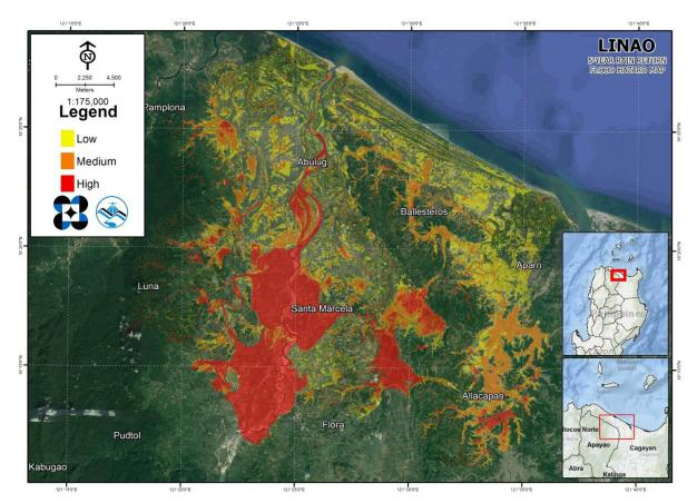
Figure 70. 5-year Flood Hazard Map for the Linao Floodplain
