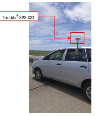
Figure 45. Validation points acquisition survey set-up along the Linao River Basin
