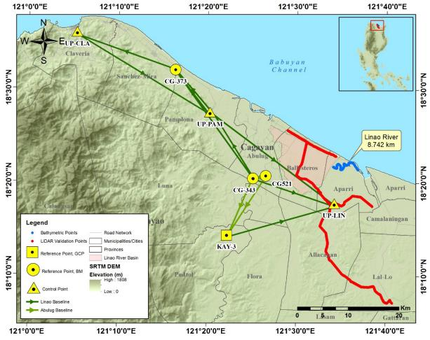
Figure 32. Extent of the bathymetric survey (in blue line) in the Linao River and the LiDAR data validation survey (in red).
