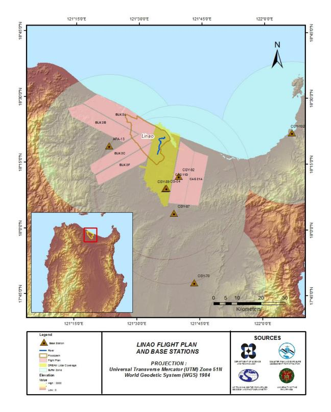
Figure 2. Flight plans and base stations used to cover the Linao floodplain survey
