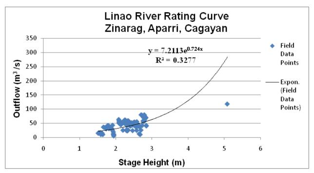
Figure 53. HQ Curve of the HEC-HMS model
