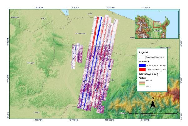
Figure A-8.14. Elevation difference between flight lines
