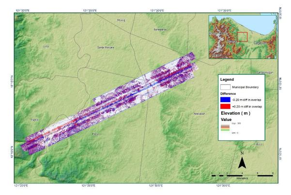
Figure A-8.21. Elevation difference between flight lines
