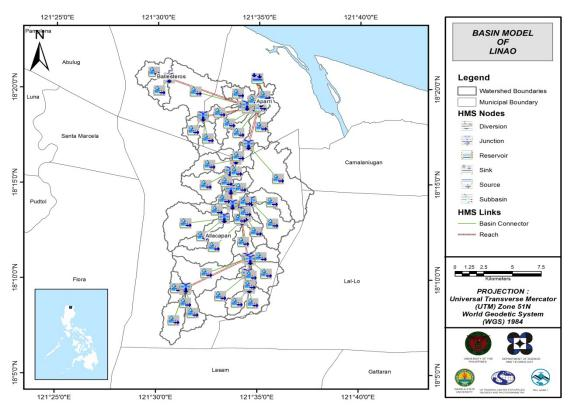
Figure 60. Linao River Basin Model generated in HEC-HMS
