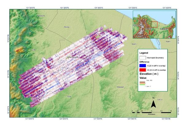
Figure A-8.28. Elevation difference between flight lines
