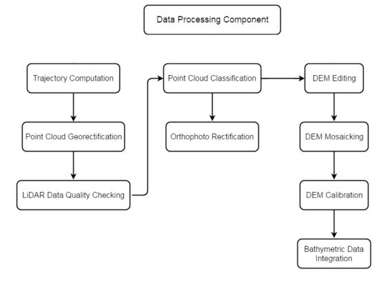
Figure 10. Schematic Diagram for Data Pre-Processing Component
