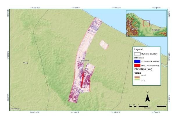
Figure A-8.7. Elevation difference between flight lines
