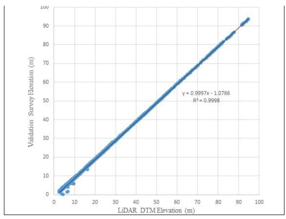
Figure 28. Correlation plot between the validation survey points and the LiDAR data.
