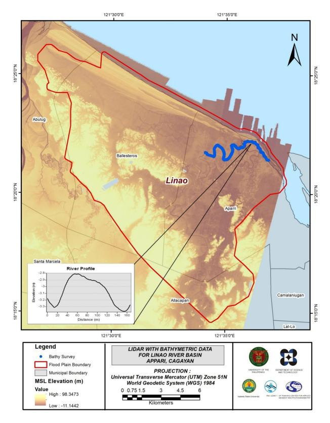
Figure 29. Map of the Linao floodplain with bathymetric survey points shown in blue
