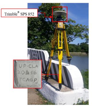
Figure 37. GNSS receiver set-up, Trimble<sup>®</sup> SPS 852, at UP-CLA, located at the approach of Cabicungan Bridge in Barangay Dibalio, Municipality of Claveria, Cagayan
