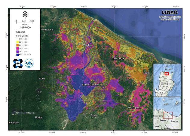
Figure 69. 25-year Flow Depth Map for the Linao Floodplain
