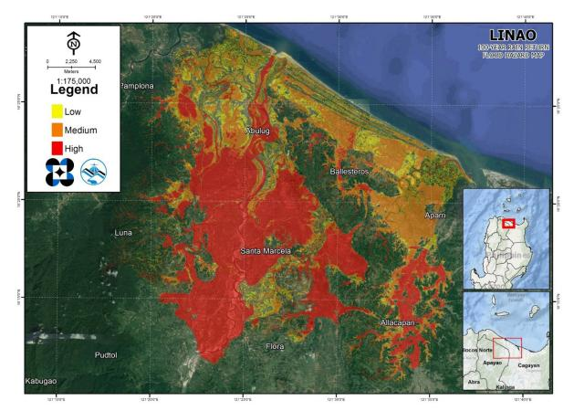
Figure 66. 100-year Flood Hazard Map for the Linao Floodplain
