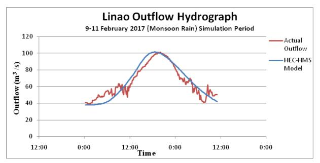
Figure 63. Outflow Hydrograph of Linao produced by the HEC-HMS model compared with observed outflow.
