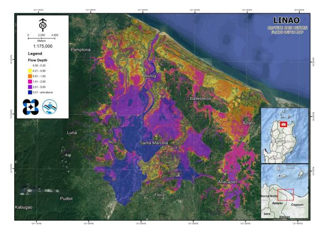
Figure 67. 100-year Flow Depth Map for the Linao Floodplain
