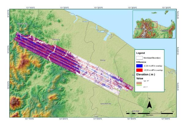
Figure A-8.56. Elevation difference between flight lines
