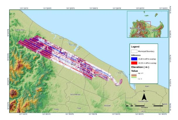
Figure A-8.35. Elevation difference between flight lines
