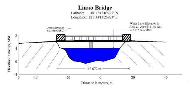
Figure 42. Linao Bridge cross-section diagram
