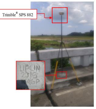
Figure 38. GNSS receiver set-up, Trimble<sup>®</sup> SPS 882, at UP-LIN, located at the approach of the Linao Bridge in Barangay Bangag-Zingag, Municipality of Aparri, Cagayan
