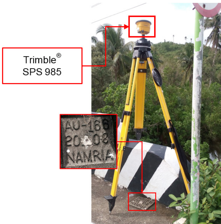
Figure 34. GNSS receiver setup, Trimble® SPS 985 at AU-166, located at the approach of Disulon Bridge in Brgy. Tinib, Municipality of Casiguran, Aurora
