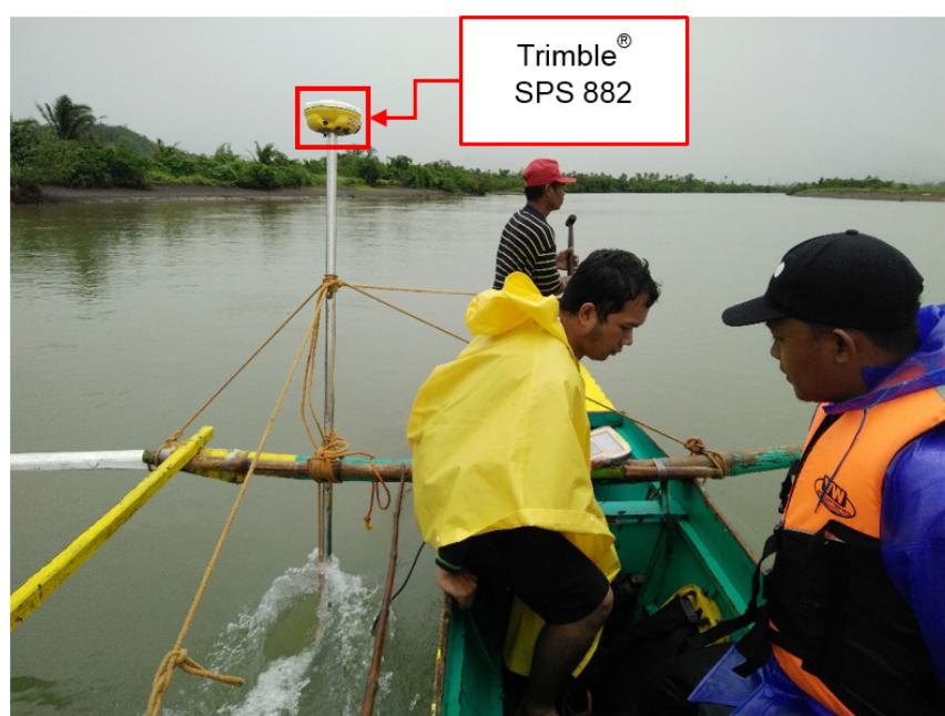
Figure 51. Bathymetric survey using a Trimble® SPS 882 in GNSS PPK survey technique in Casiguran and Casalugan Rivers
