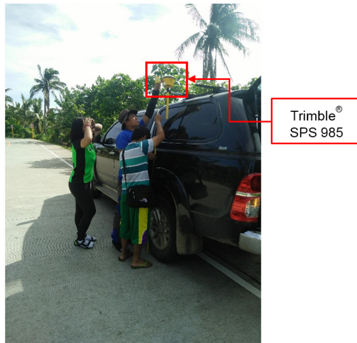
Figure 49. Validation Points Acquisition survey set up along Amro River Basin
