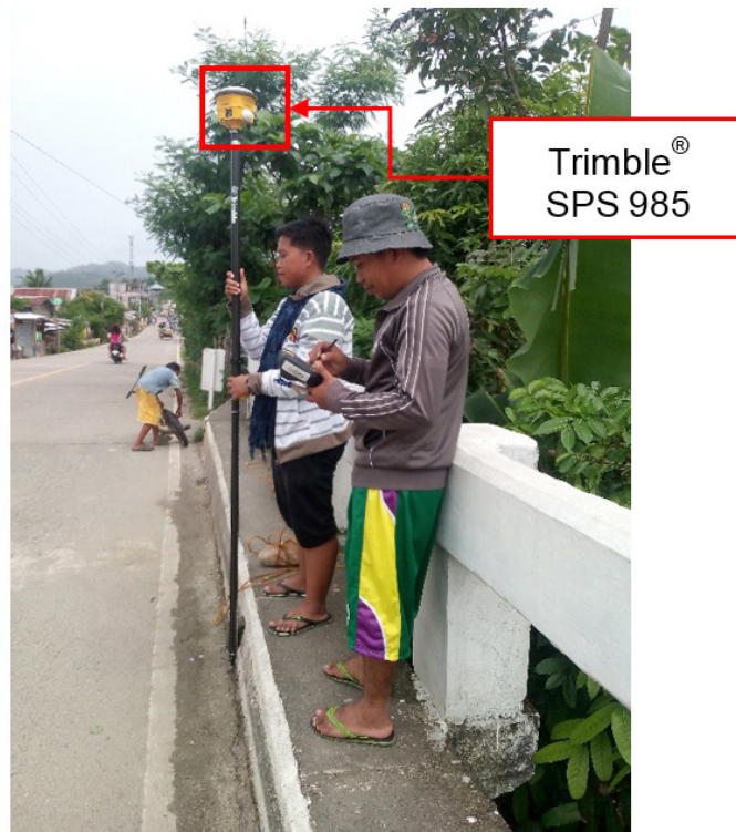
Figure 39. As-built survey of Casiguran Bridge
