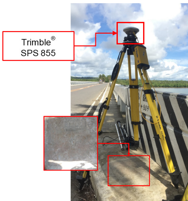
Figure 37. GNSS receiver setup, Trimble® SPS 855, at UP-ULO-2, located at the approach of Casalugan Bridge in Brgy. Culat, Municipality of Casiguran, Aurora
