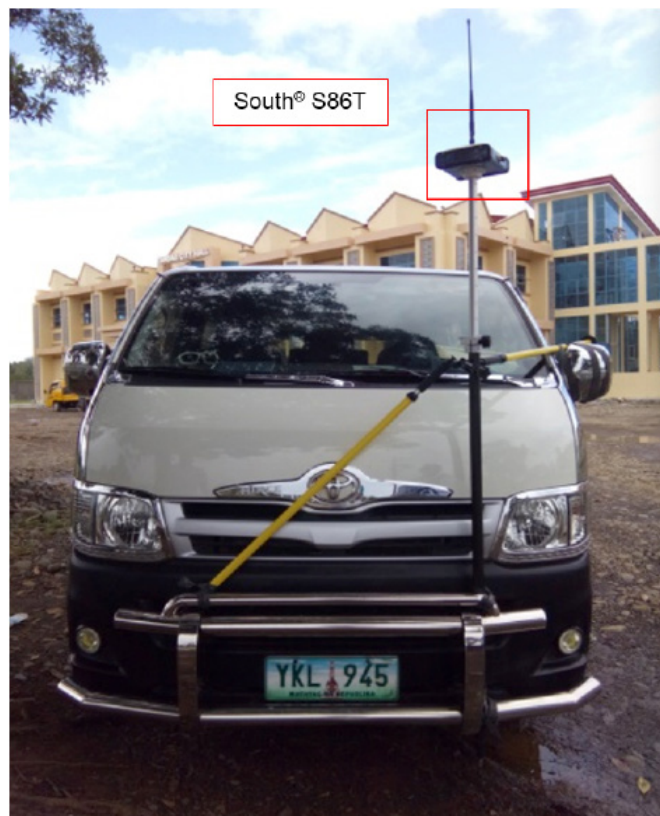
Figure 37. GNSS Receiver South® S86T installed on a vehicle for ground validation survey
