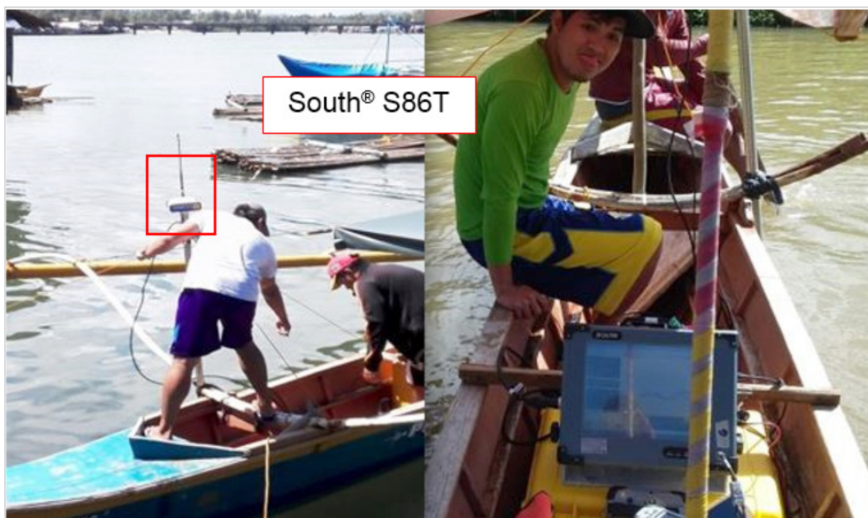
Figure 39. Set up of bathymetric survey in Tandag River
