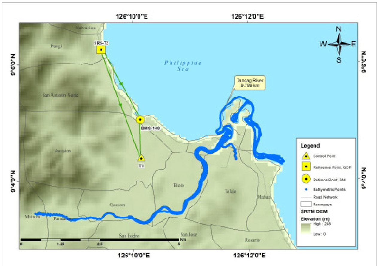
Figure 31. GNSS network of Tandag River field survey
