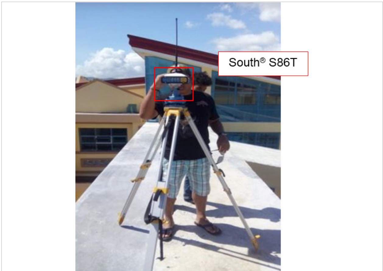
Figure 34. GNSS base receiver set-up, South® S86T, on T-1 on top of the New Tandag City Hall in Brgy. Awasian, Tandag City
