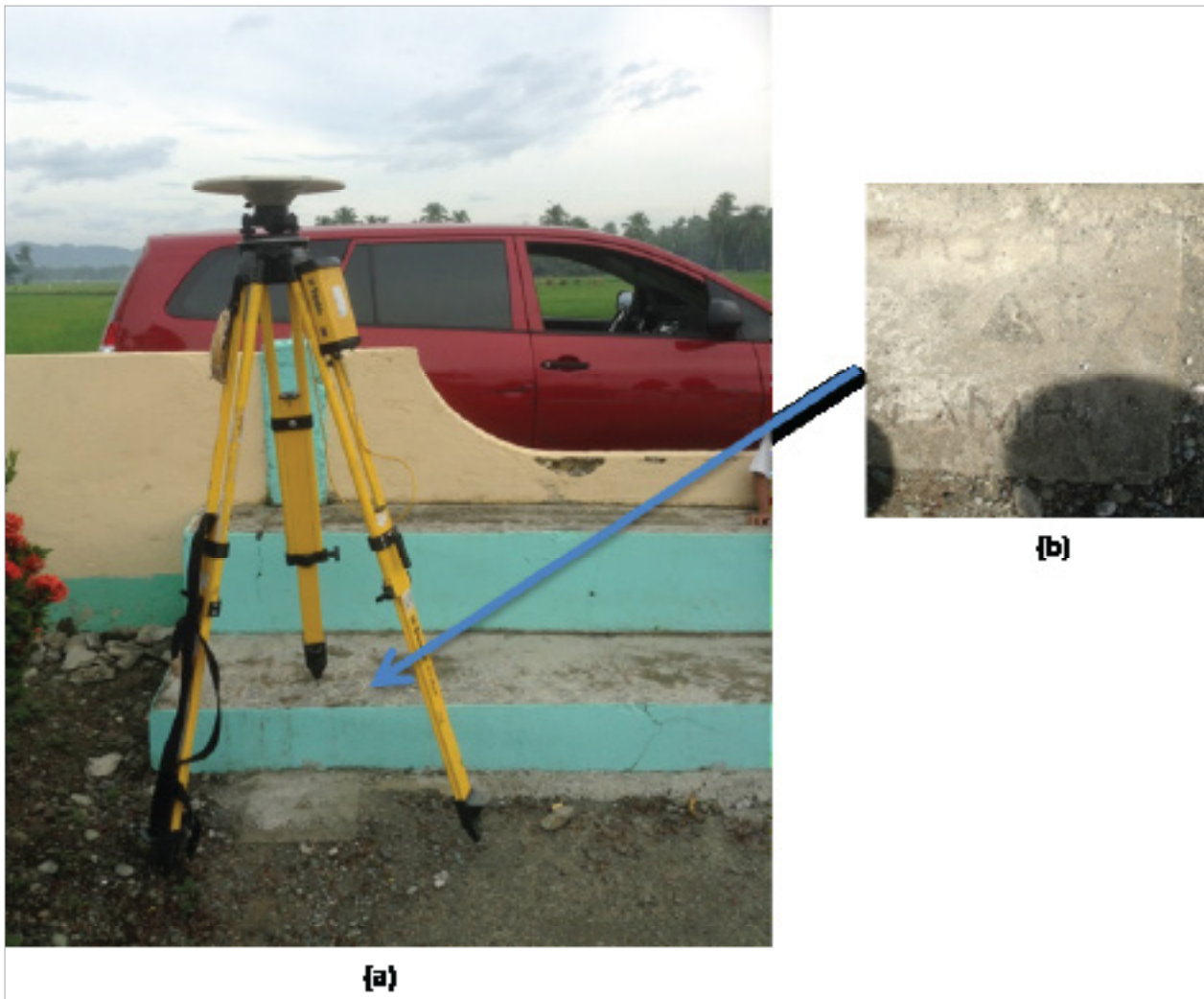
Figure 6. GPS set-up over SRS-47 located on the left side ground corner of the barangay hall about 60 m from the crossing in Brgy. Manga, Madrid, Surigao del Sur (a) NAMRIA reference point SS-101 (b) as recovered by the field team
