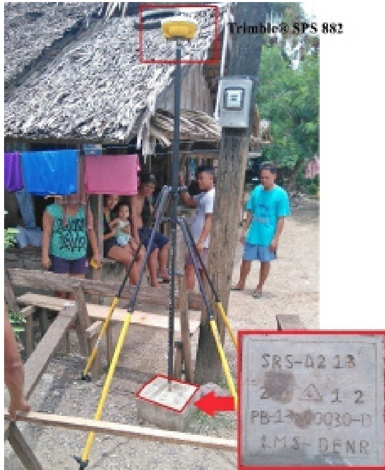
Figure 36. GNSS receiver set-up, Trimble® SPS 882 at BMSS-4213, located near Burboanan Bridge in Brgy. Burboanan, Bislig City, Surigao del Sur
