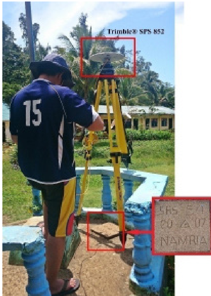
Figure 32. Trimble® SPS 852 set-up at SRS-54 near the flag pole of Gata Integrated School in San Agustin, Surigao del Sur
