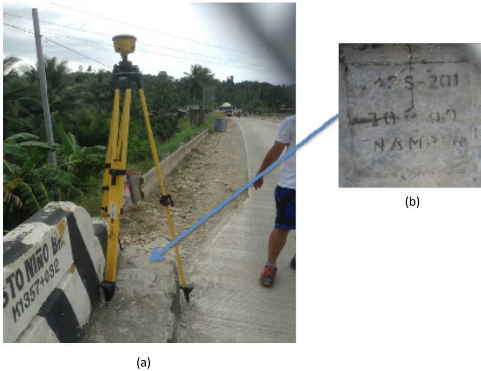
Figure 5. GPS set-up over BMSS-201 located in Sto. Nino Bridge in San Agustin, Surigao del Sur (a) and NAMRIA reference point SM-201 (b) as recovered by the field team
