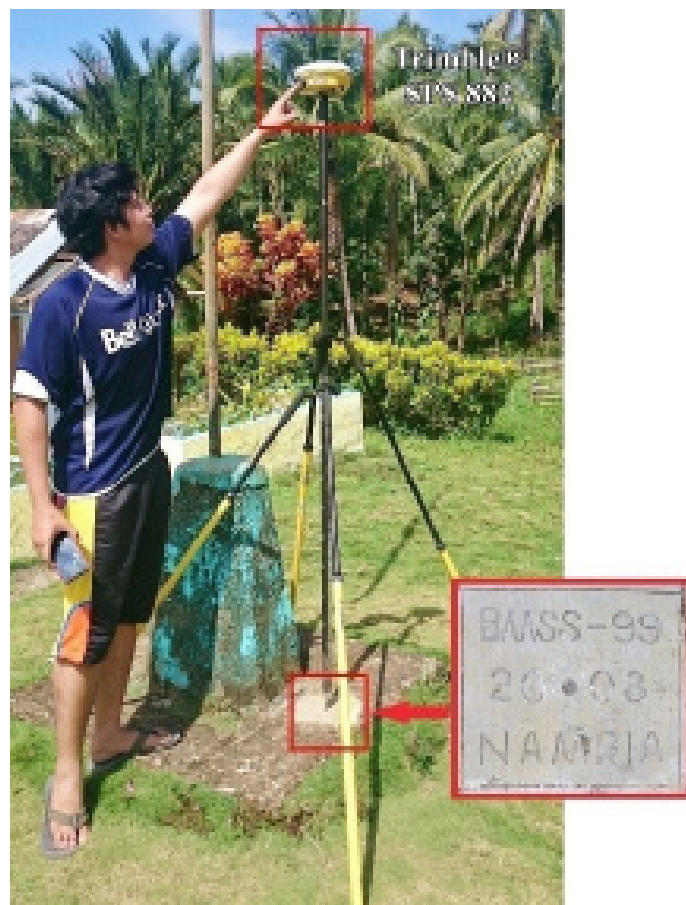
Figure 35. GNSS receiver set-up, Trimble® SPS 882 at BMSS-99, located inside Mahayhay Primary School in the Municipality of Hinatuan, Surigao del Sur
