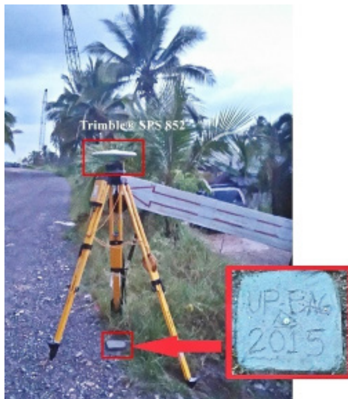
Figure 37. GNSS base set-up, Trimble® SPS 852 at UP-BAG, located near Bagnan Bridge in Brgy. Mone, Bislig City, Surigao del Sur
