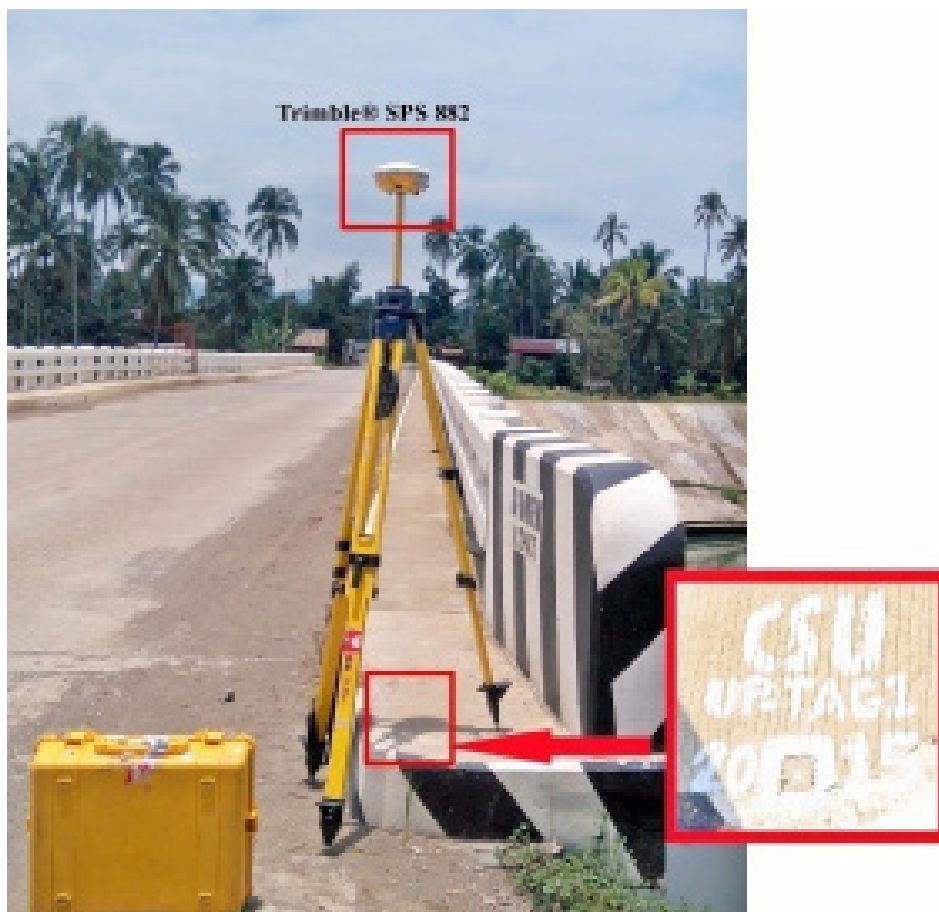
Figure 40. GNSS base set-up, Trimble® SPS 882 at UP-TAG1, located at Tago-San Miguel Bridge, Municipality of San Miguel, Surigao del Sur
