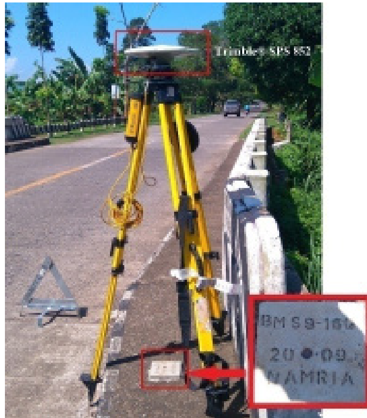
Figure 34. GNSS base set-up, Trimble® SPS 852 at BMSS-160, located at Pamuksukan Bridge in Brgy. Gamut, Tago, Surigao del Sur
