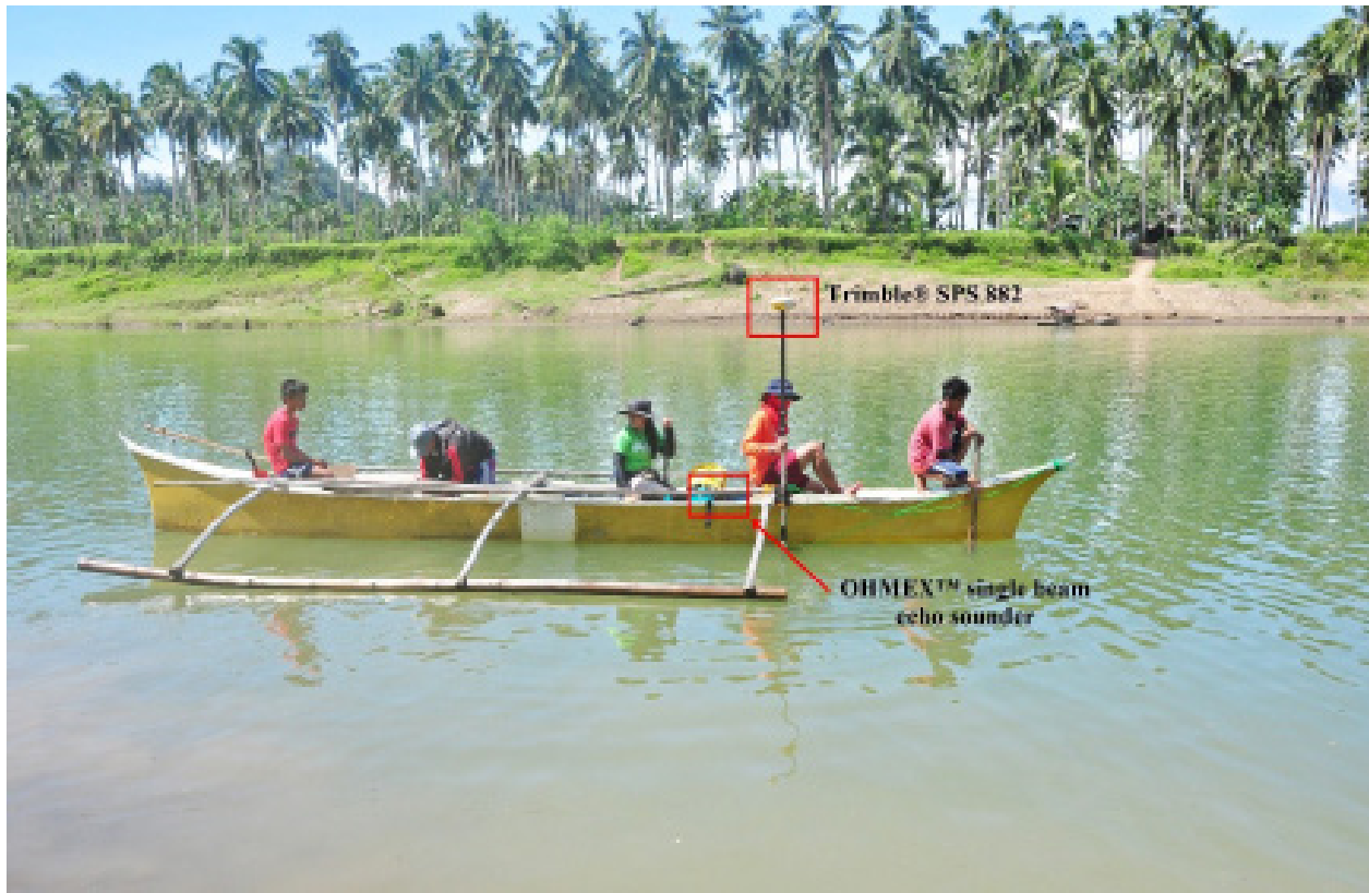
Figure 47. Bathymetry set-up using OHMEX™ single beam echo sounder with a Trimble® SPS 882
