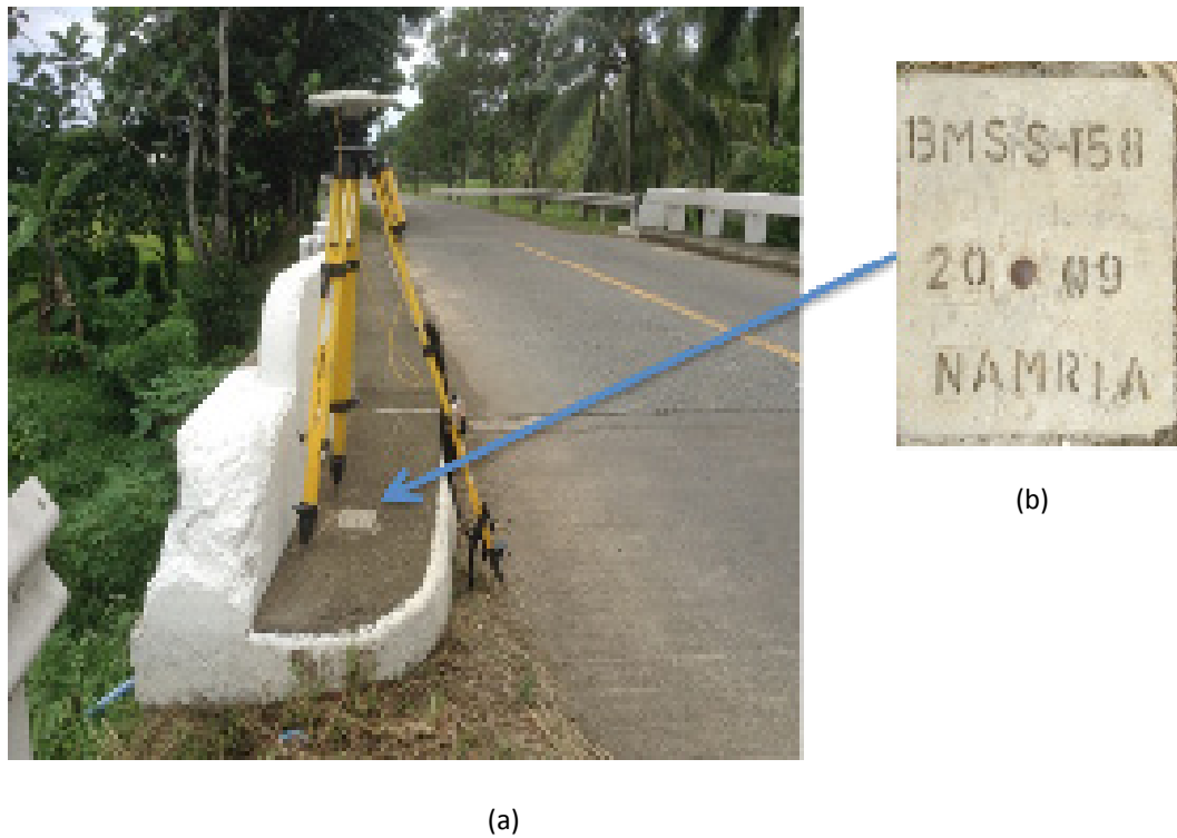
Figure 3. GPS set-up over BMSS-158 located at Batang Bridge in Brgy. Dayo-an, Surigao del Sur (a) and NAMRIA reference point SM-286 (b) as recovered by the field team
