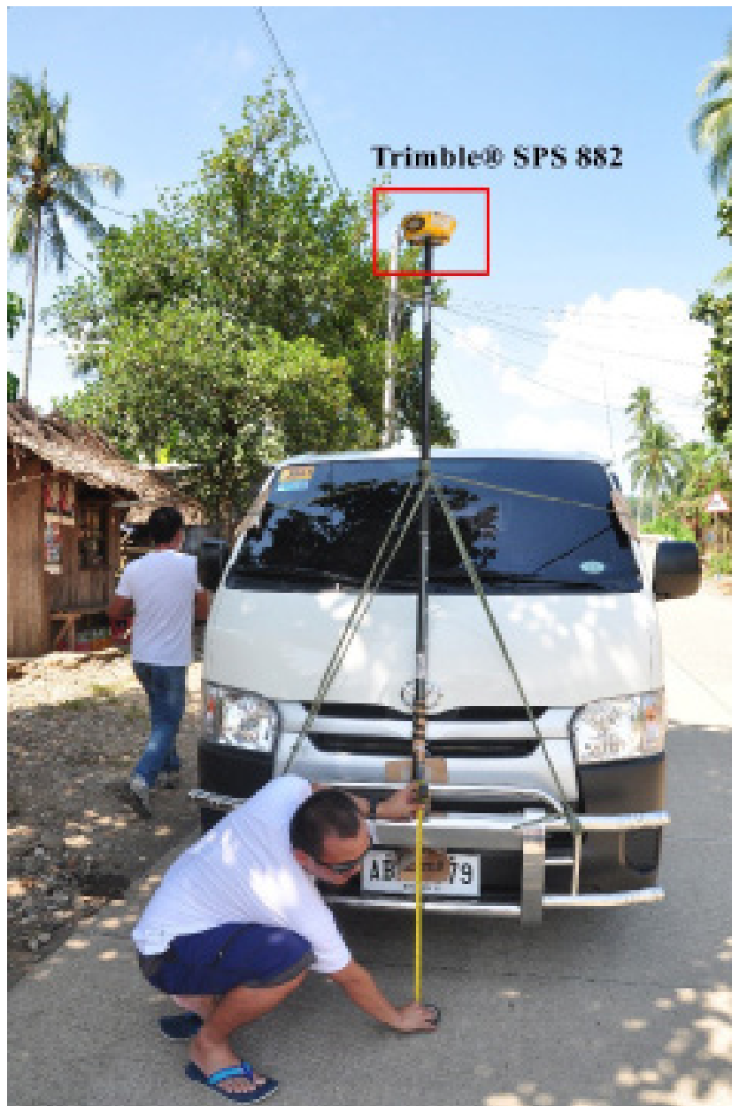
Figure 45. Validation points acquisition survey set-up: A Trimble® SPS 882, mounted in a 2-meter pole and attached in front of the vehicle
