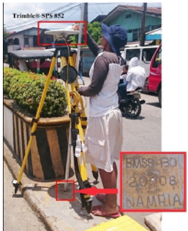
Figure 33. GNSS base set-up, Trimble® SPS 852 at BMSS-130, located on one end of a concrete barrier along Surigao-Davao Coastal Road in Brgy. Mangagoy, Bislig City, Surigao del Sur
