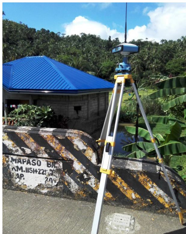
Figure 34. GNSS base set up, South® S86T, at SN-59, located at the approach of Mapaso Bridge in Brgy. Magsaysay, Placer, Province of Surigao del Norte.
