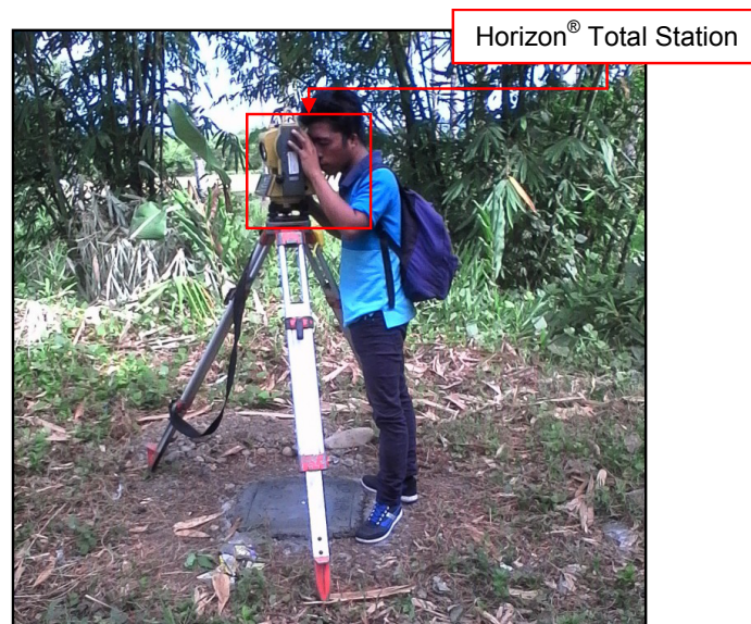
Figure 37. Cross-section survey conducted at Kinabutan Bridge.
