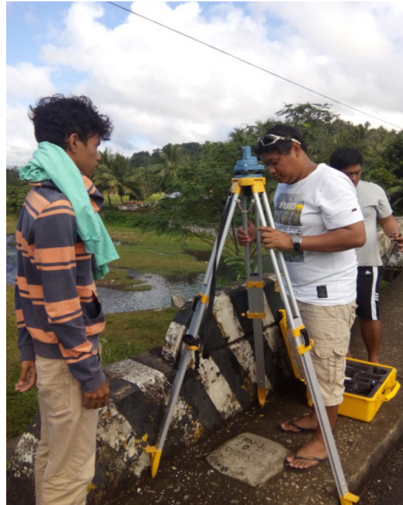
Figure 32. GNSS receiver set up, South® S86T, at SRN-3031, located at the approach of Mabuhay Bridge in Brgy. Mabuhay, Sison, Province of Surigao del Norte.
