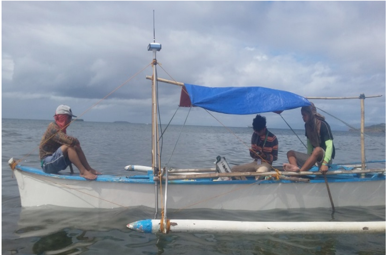
Figure 44. Set up of the bathymetric survey in Surigao River
