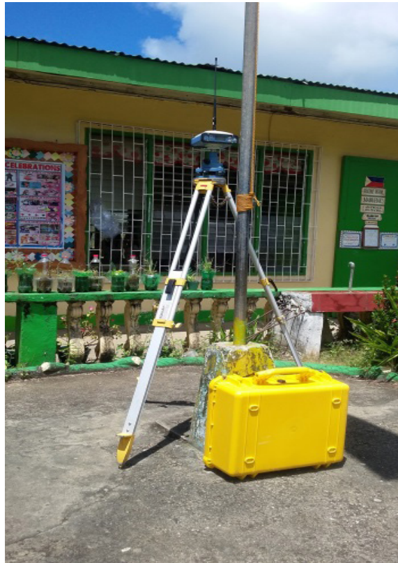
Figure 33. GNSS receiver set up, South® S86T, at SRN-99, located inside Bonifacio Elementary School in Brgy. Bonifacio, Surigao City, Province of Surigao del Norte.
