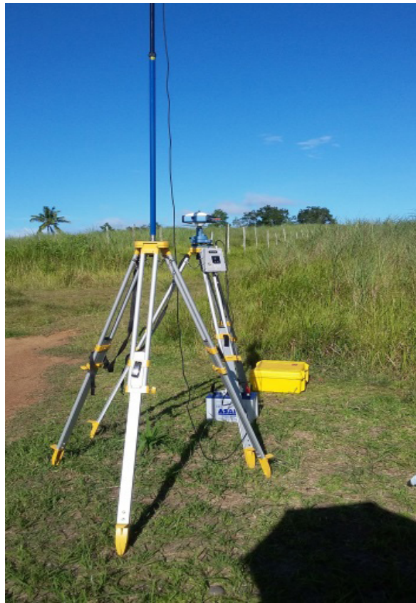
Figure 35. GNSS receiver set up, South® S86T, at T-1, located in Brgy. Luna, Surigao City, Province of Surigao del Norte.
