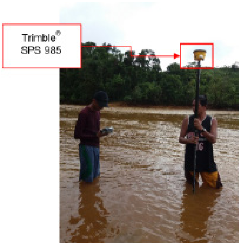
Figure 38. Manual bathymetric survey using a Trimble® SPS 985 in GNSS PPK survey technique in Malinao Inlet River
