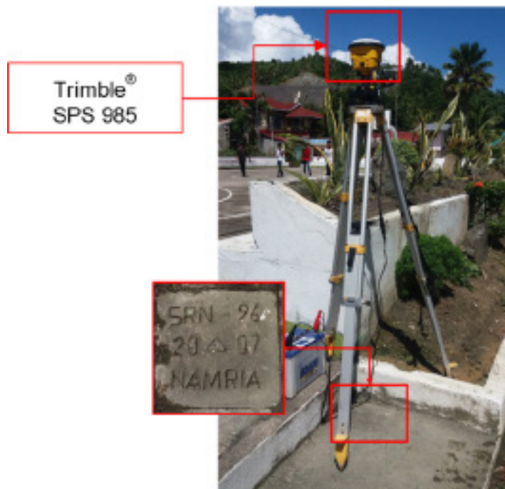
Figure 30. GNSS base receiver setup, Trimble® SPS 985, at SRN-96 in Brgy. Poblacion, Municipality of Cagdianao, Dinagat Islands.
