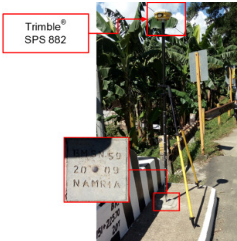
Figure 29. GNSS base receiver setup, Trimble® SPS 882 at SN-59 in Brgy. Magsaysay, Municipality of Placer, Surigao Del Norte.
