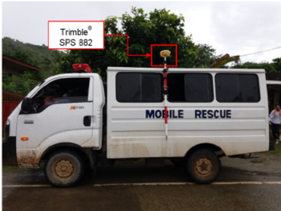
Figure 35. GNSS Receiver Trimble® SPS 882 installed on a vehicle for Ground Validation Survey
