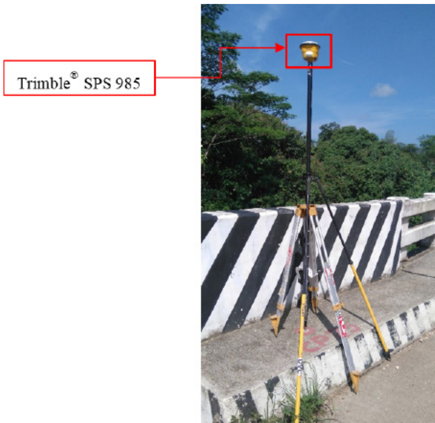
Figure 45. GNSS base set-up, Trimble® SPS 985, at UP-MAG, located at the Maglambing Bridge along Surigao-Davao Coastal Road in Barangay Maglambing in the Municipality of Tagbina, Surigao del Sur
