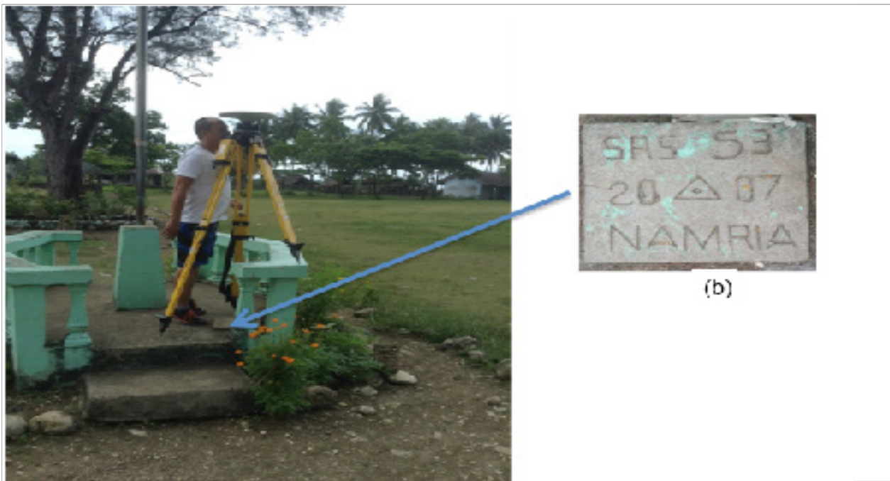
(a) Figure 12. GPS Set-up over SRS-53
