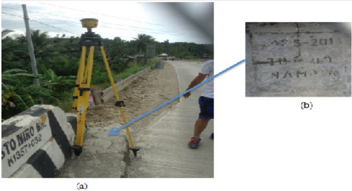
Figure 11. GPS Set-up over BMSS-201
