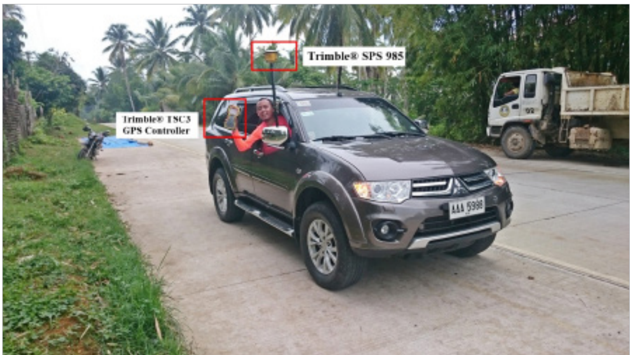
Figure 51. Validation points acquisition survey set up along the Hinatuan River Basin
