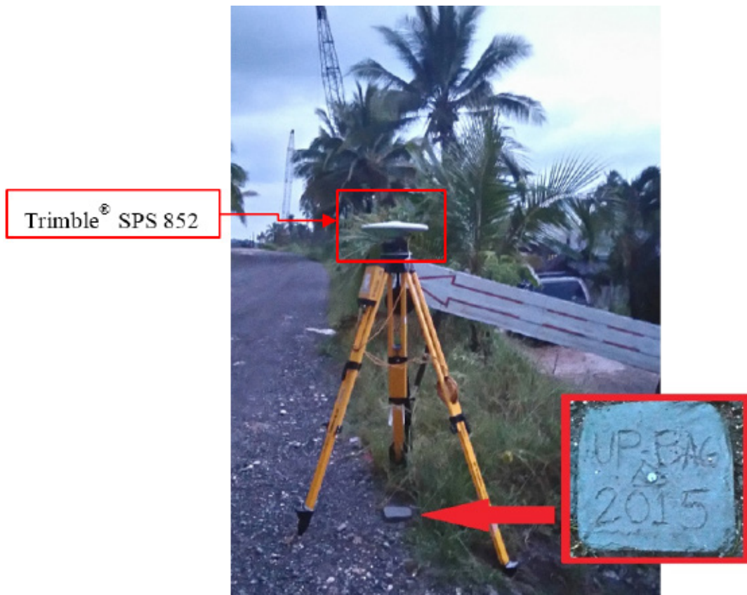
Figure 43. GNSS base set-up, Trimble® SPS 852, at UP-BAG, located near the Bagnan Bridge in Barangay Mone, Bislig City, Surigao del Sur
