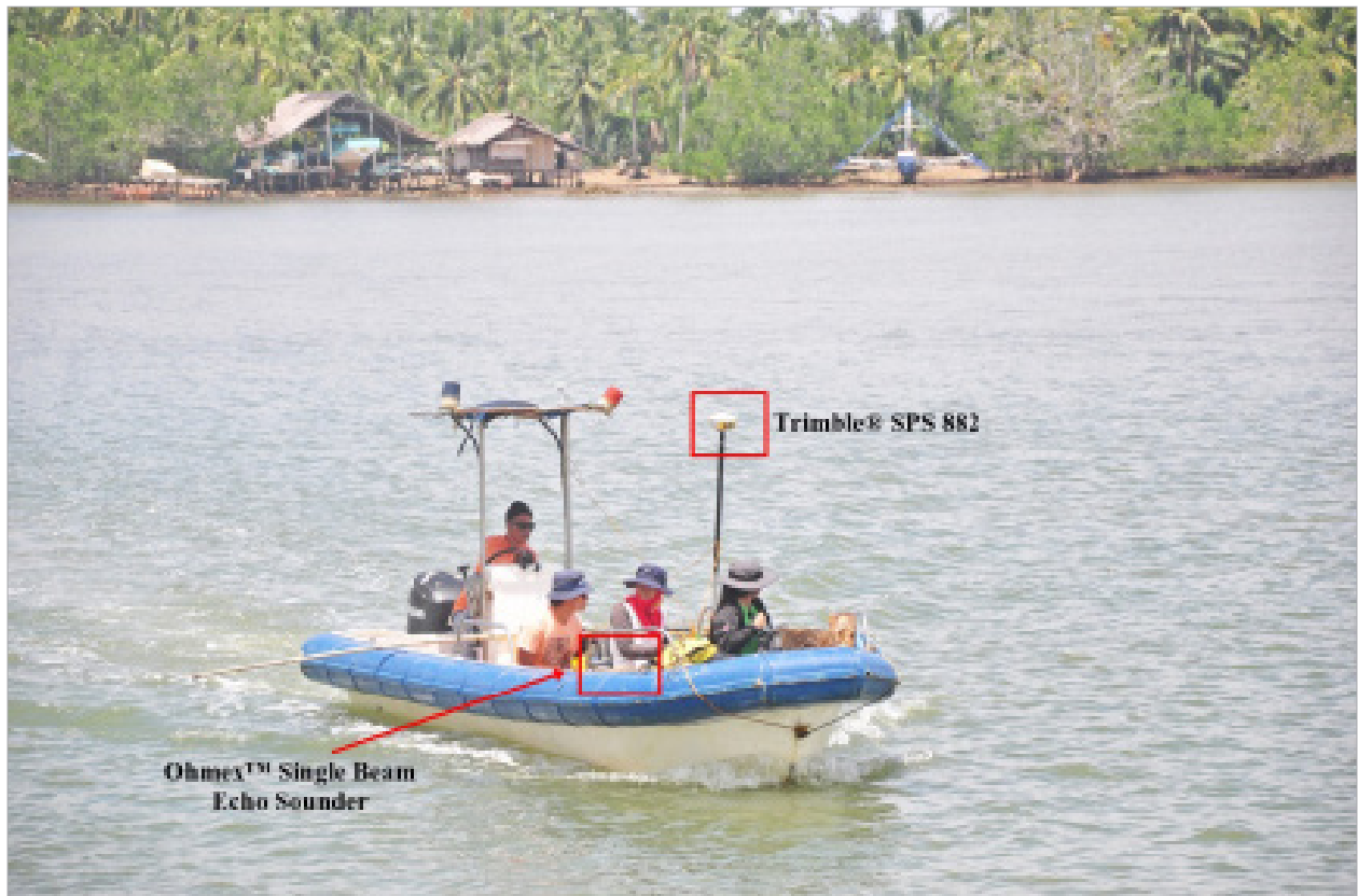
Figure 53. Bathymetry set-up using OHMEX™ single beam echo sounder in Hinatuan River
