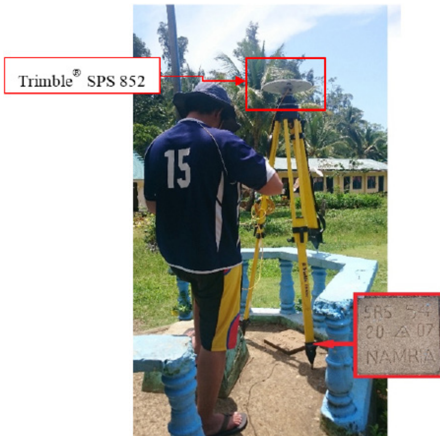
Figure 41. GNSS receiver set-up, Trimble® SPS 853, at SRS-54 near the flag pole of the Gata Integrated School in San Agustin, Surigao del Sur
