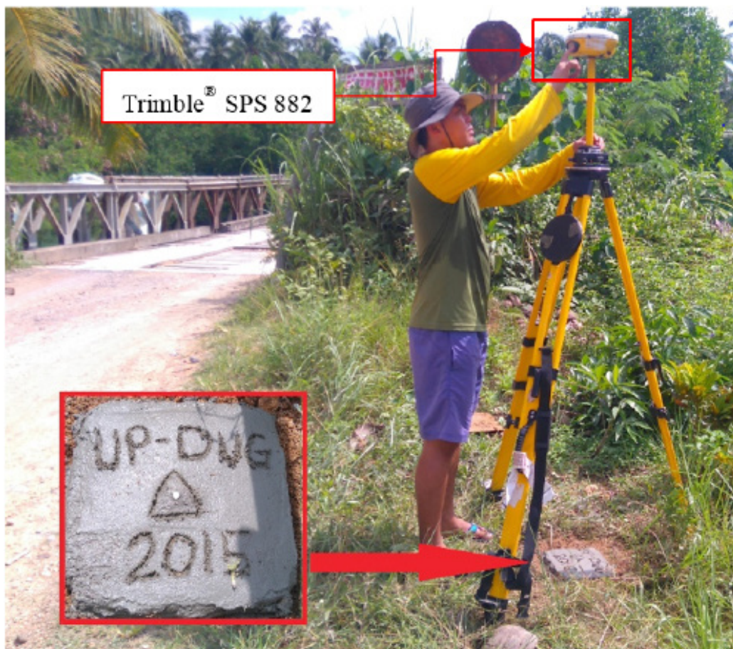
Figure 44. GNSS receiver set-up, Trimble® SPS 882, at UP-DUG, located near the Hinatuan Bridge in the Municipality of Hinatuan, Surigao del Sur
