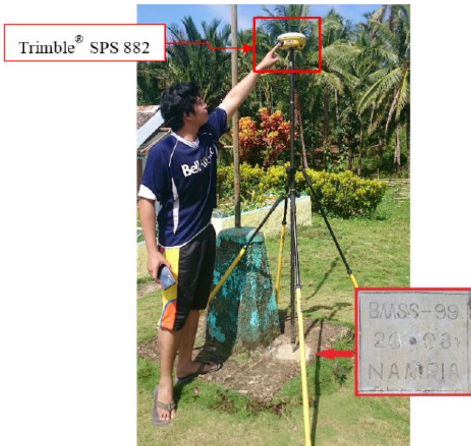
Figure 40. GNSS receiver set-up, Trimble® SPS 882, at BMSS-99 located inside the Mahayhay Primary School in the Municipality of Hinatuan, Surigao del Sur
