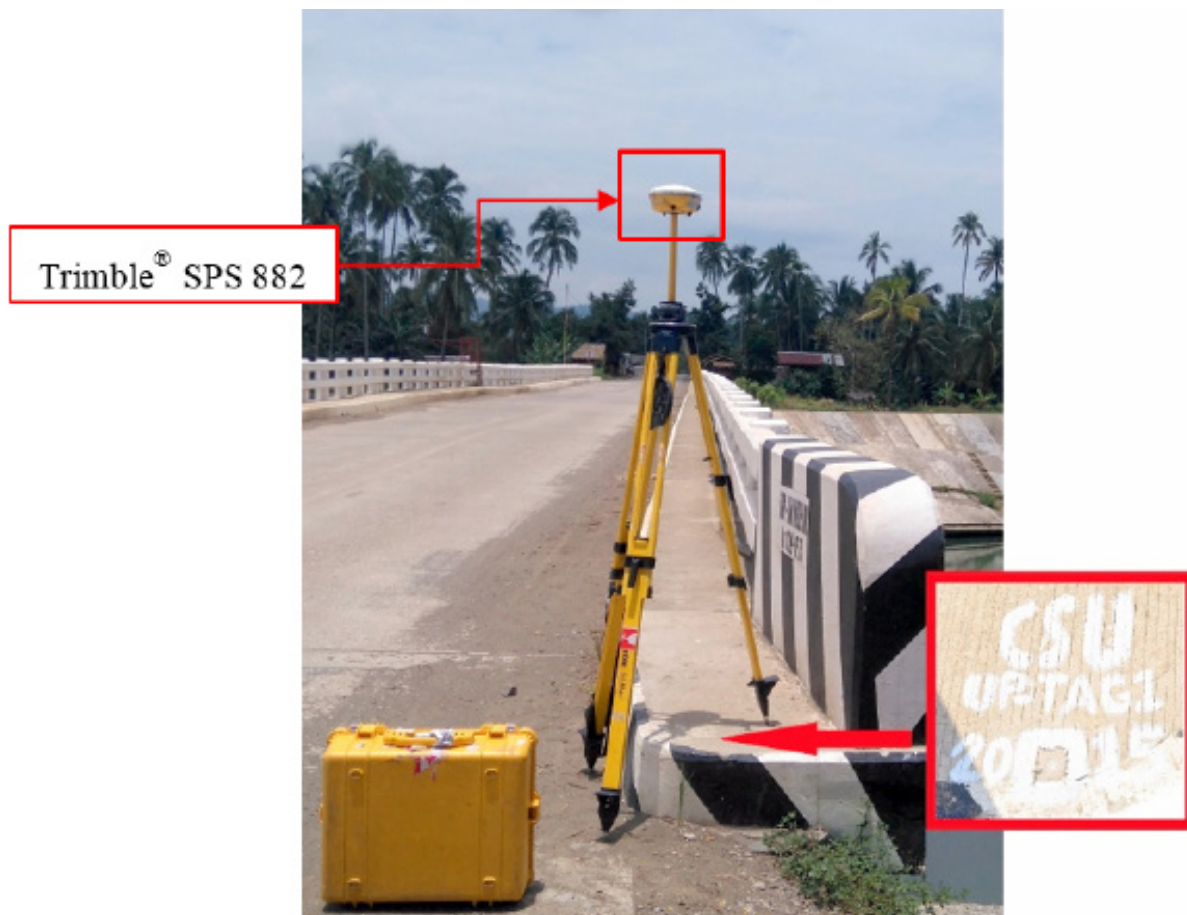
Figure 46. GNSS base set-up, Trimble® SPS 882, at UP-TAG1, located at the Tago-San Miguel Bridge, Municipality of San Miguel, Surigao del Sur
