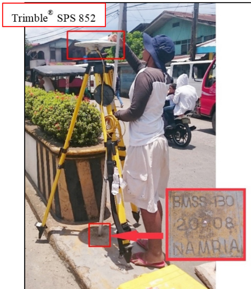
Figure 38. GNSS base set-up, Trimble® SPS 852, at BMSS-130 located on one end of a concrete barrier along Surigao-Davao Coastal Road in Barangay Mangagoy, Bislig City, Surigao del Sur
