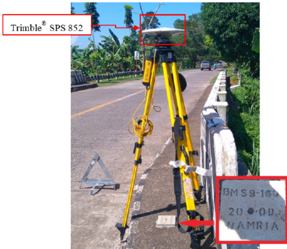
Figure 39. GNSS base set-up, Trimble® SPS 852, at BMSS-160, located at Pamuksukan Bridge in Barangay Gamut, Tago, Surigao del Sur
