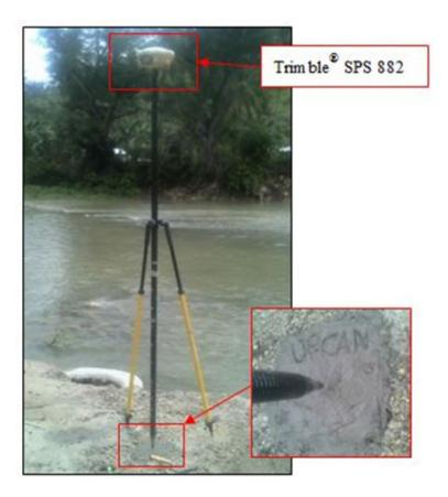
Figure 33. Trimble® SPS 882 receiver set-up at UP-CAN located at the right side of Cangabo Spillway in Brgy. Pangca, Municipality of La Libertad.
