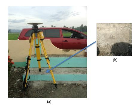
Figure 4 GPS set-up over SRS-47 located on the left side ground corner of the barangay hall about 60m from the crossing in Brgy. Manga, Madrid, Surigao del Sur (a) NAMRIA reference point SS-101 (b) as recovered by the field team
