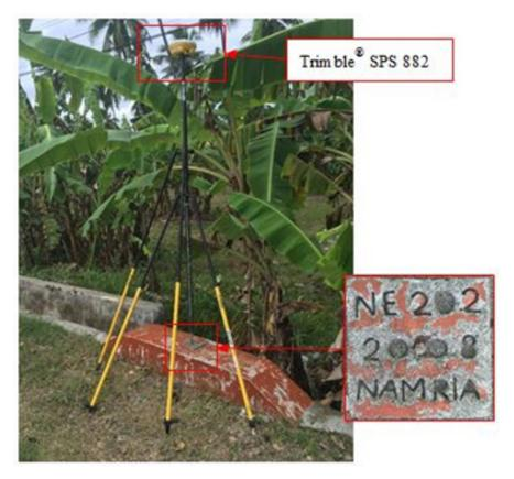
Figure 32. Trimble® SPS 882 receiver set-up at UP-CAN located at the right side of Cangabo Spillway in Brgy. Pangca, Municipality of Libertad.
