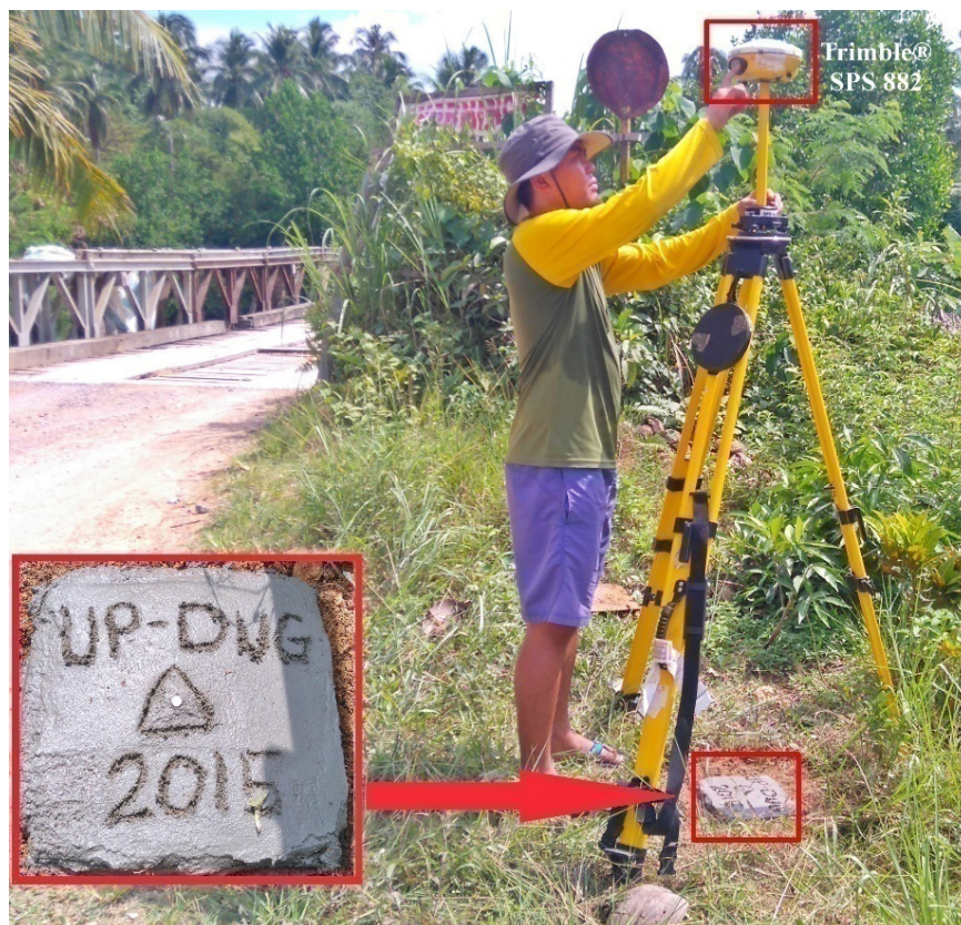
Figure 41. Trimble® SPS 882 setup at UP-DUG, located near Dugmanon Bridge in the Municipality of Hinatuan, Surigao del Sur
