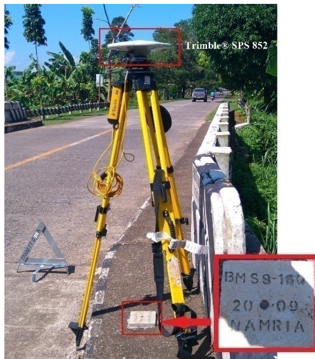
Figure 37. GNSS base set up, Trimble® SPS 852 at BMSS-160, located at Pamuksukan Bridge in Brgy. Gamut, Tago, Surigao del Sur
