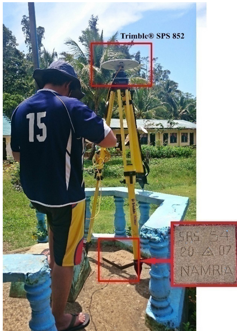
Figure 35. Trimble® SPS 852 setup at SRS-54 near the flag pole of Gata Integrated School in San Agustin, Surigao del Sur
