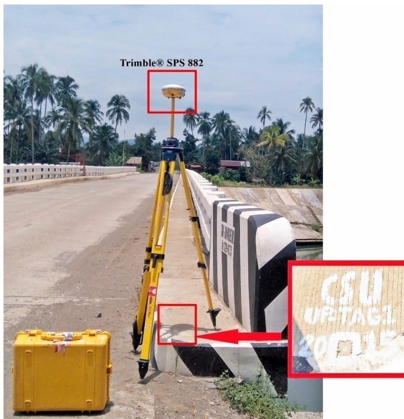
Figure 43. GNSS base set up, Trimble® SPS 882 at UP-TAGI, located at Tago-San Miguel Bridge, Municipality of San Miguel, Surigao del Sur
