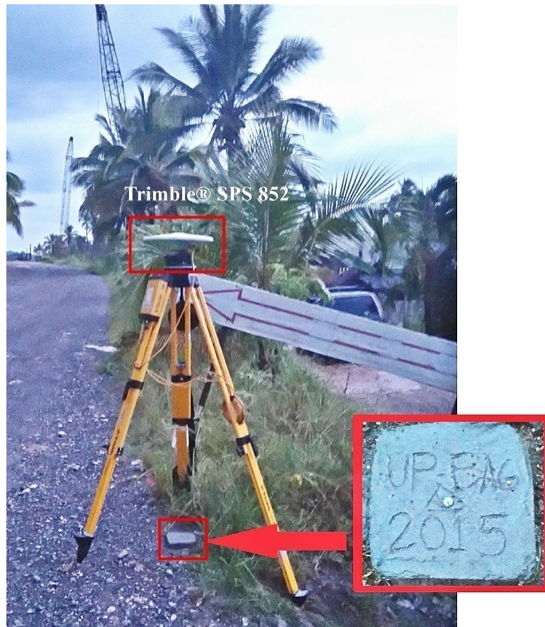
Figure 40. GNSS base set up, Trimble® SPS 852 at UP-BAG , located near Bagnan Bridge in Brgy. Mone, Bislig City, Surigao del Sur
