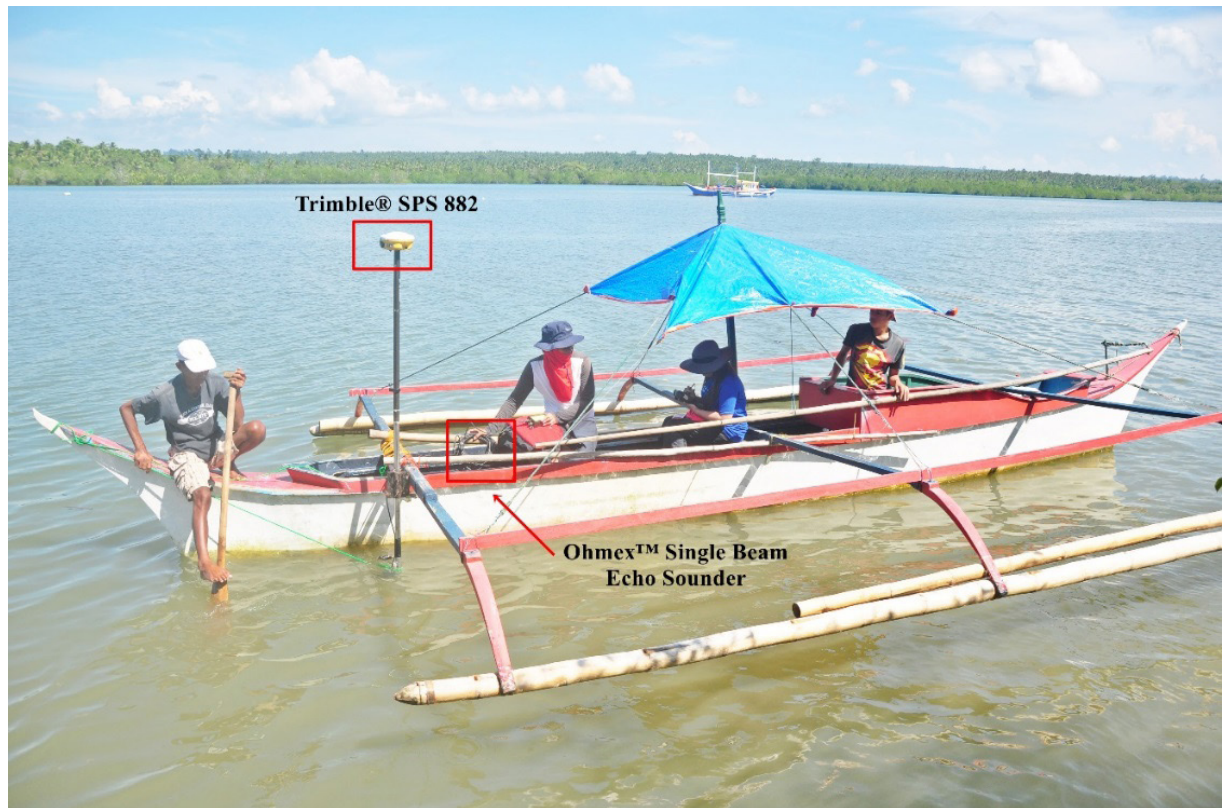
Figure 53. Bathymetry Set-up using OHMEX™ single beam echo sounder with a Trimble® SPS 882
