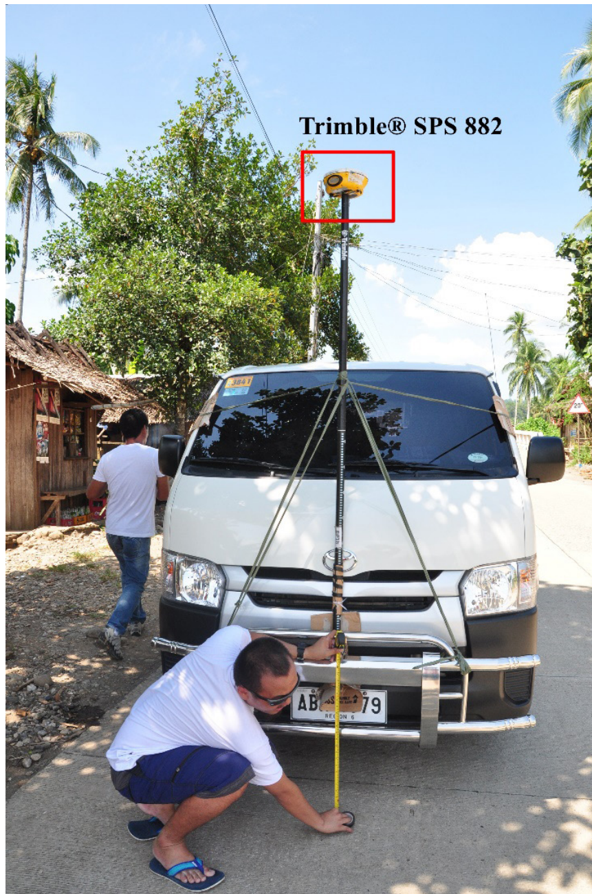
Figure 51. Ground Validation setup: A Trimble® SPS 82, mounted in a 2-meter pole and attached in front of the vehicle
