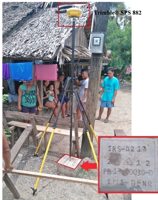
Figure 39. GNSS receiver set up, Trimble® SPS 882 at BMSS-4213 located near Burboanan Bridge in Brgy. Burboanan, Bislig City, Surigao del Sur
