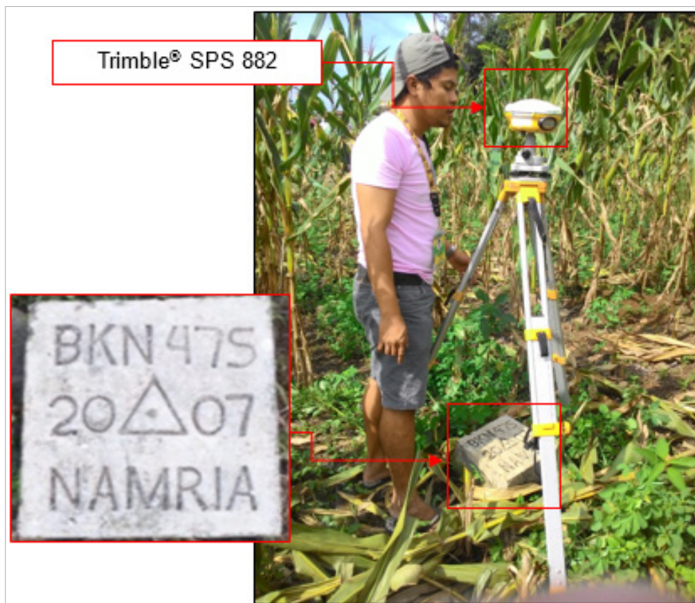
Figure 36. GNSS receiver setup, BKN-475, located within the DPWH Compound in Brgy. Aglayan, Valencia City, Bukidnon.
