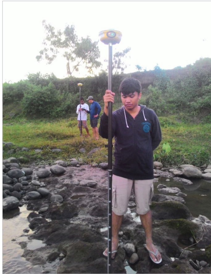
Figure 48. Gathering of random bathymetric points along Upper Pulangui River
