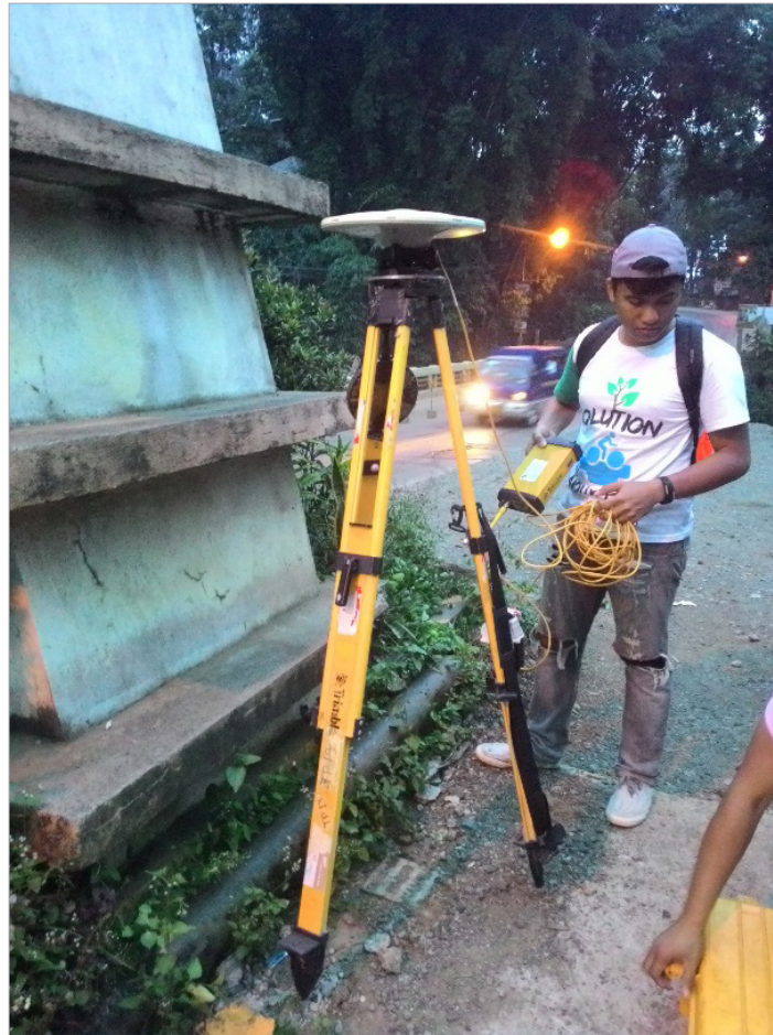
Figure 9. GPS set-up over NAMRIA benchmark BK-56 inside Agusan Barangay Plaza
