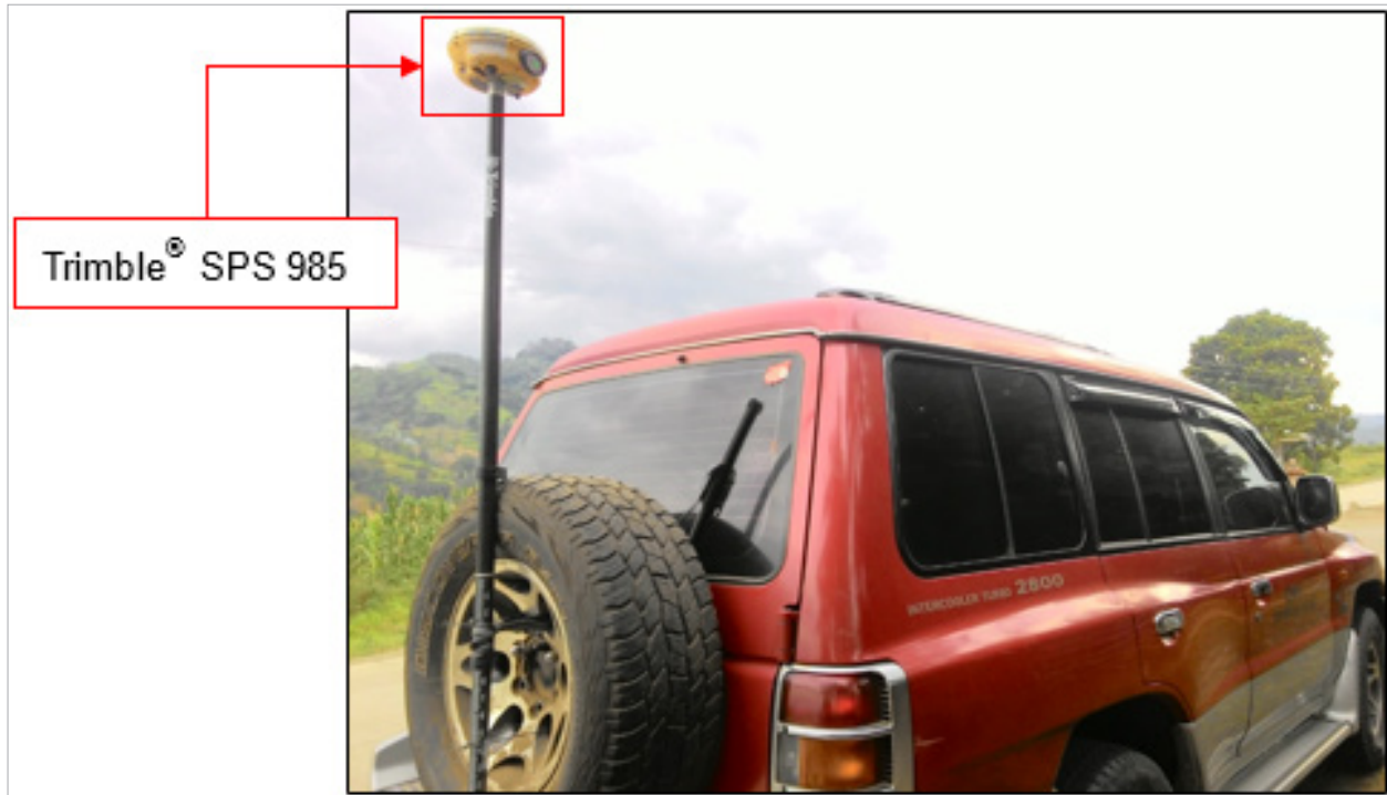
Figure 45. Validation points acquisition survey set-up for Upper Pulangi River
