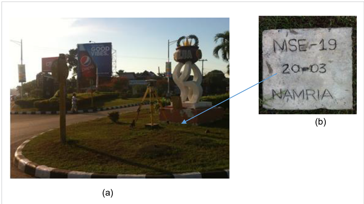
Figure 3. GPS set-up over MSE-19 at the center island located at the road intersections going to Cagayan de Oro, Butuan City and Iligan City (a) and NAMRIA reference point MSE-19 (b) as recovered by the field team.
