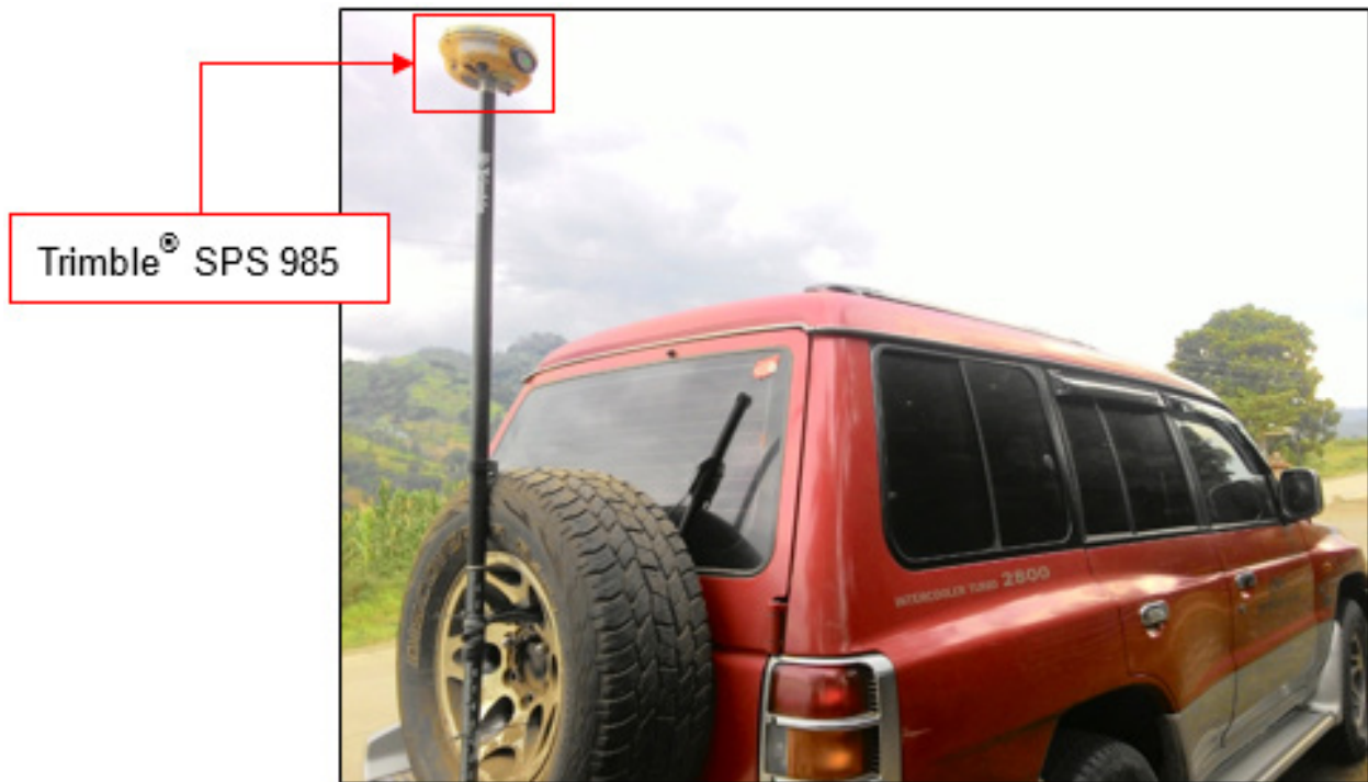
Figure 45. Validation points acquisition survey set-up for Sawaga River
