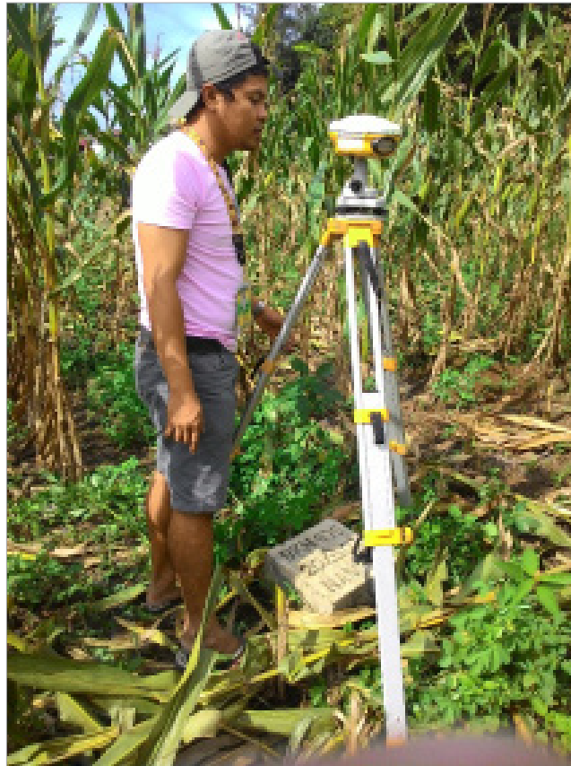
Figure 7. GPS set-up over NAMRIA reference point BKN-475 inside Agusan Barangay Plaza
