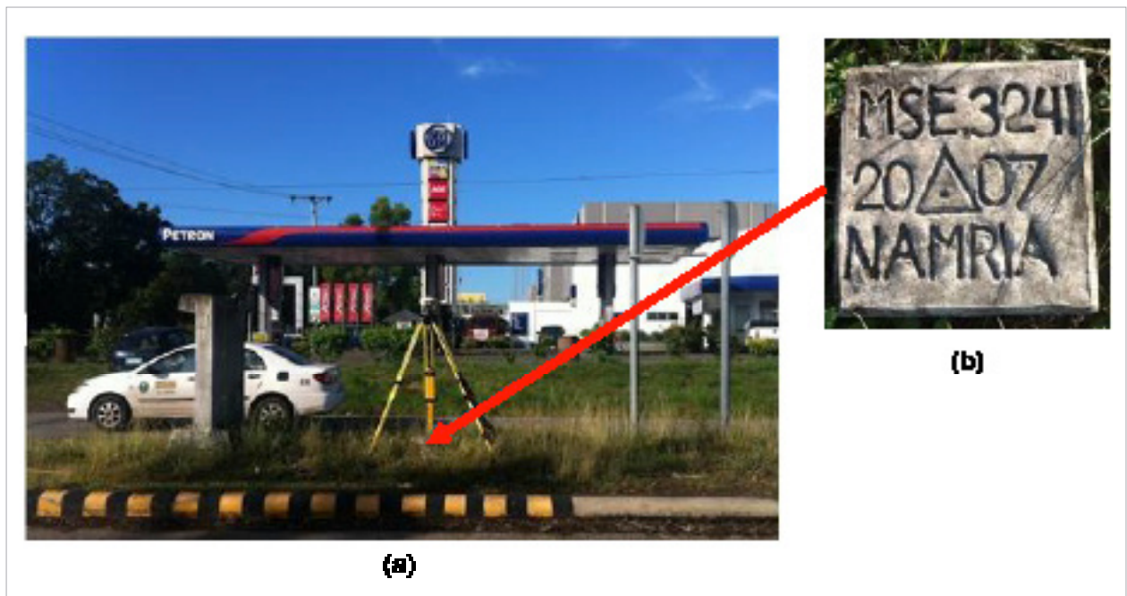
Figure 5. GPS set-up over MSE-3241 on a center island near a gasoline station beside SM Cagayan de Oro (a) and NAMRIA reference point MSE-3241 (b) as recovered by the field team.
