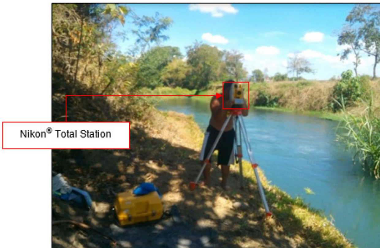
Figure 47. Manual Bathymetric survey of ABSD at Sawaga River using Nikon® Total Station
