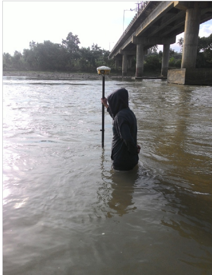
Figure 48. Gathering of random bathymetric points along Sawaga River
