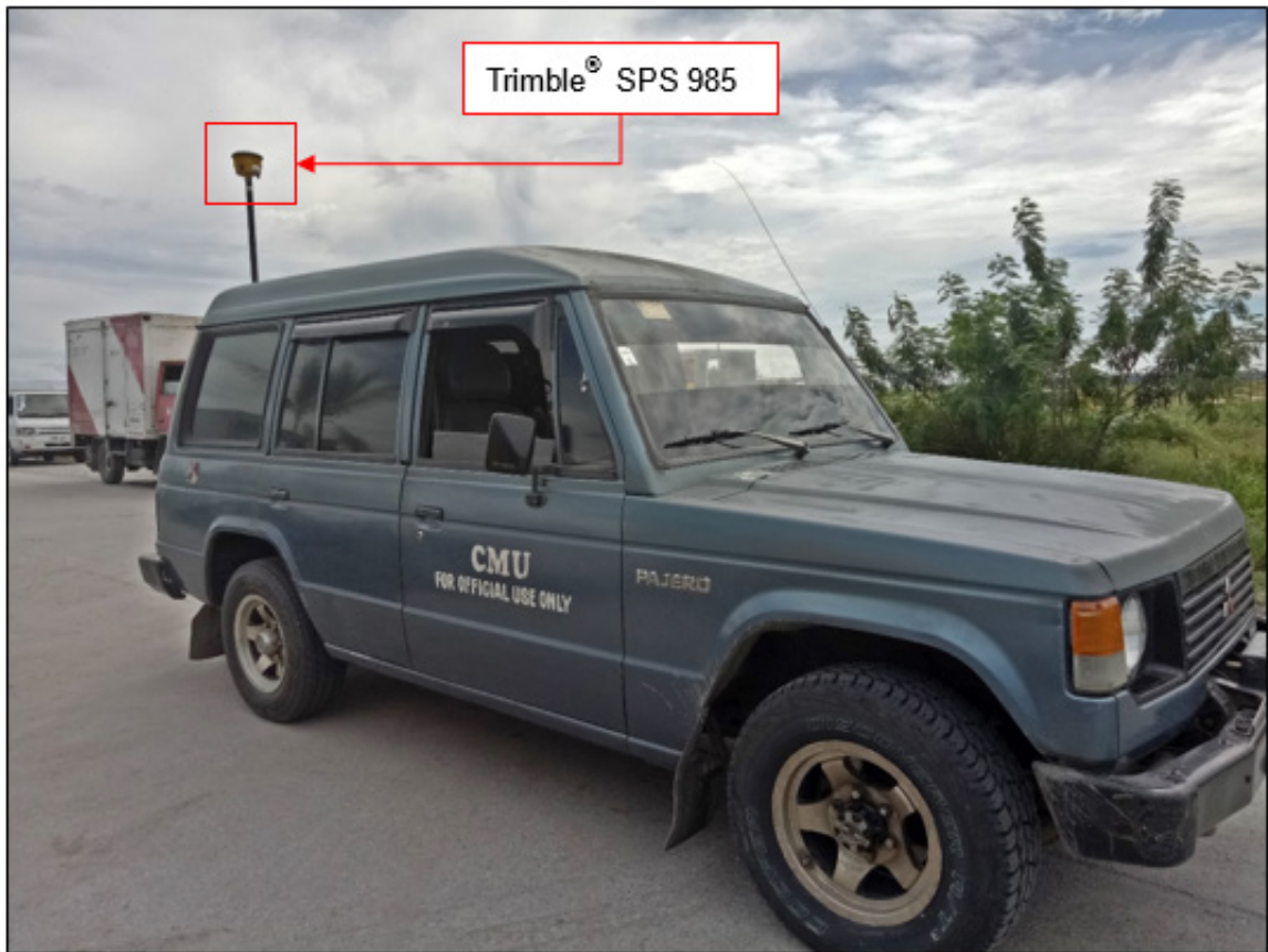
Figure 45. Validation points acquisition survey set-up for the Saub River.
