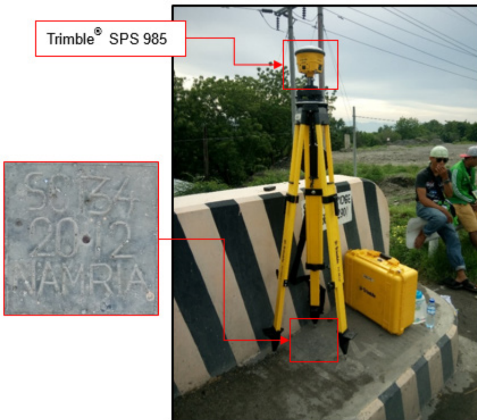
Figure 29. GNSS receiver set-up, Trimble® SPS 985, at SC-134, located at the approach of the Sinawal Bridge in Barangay Labangal, General Santos City, South Cotabato.
