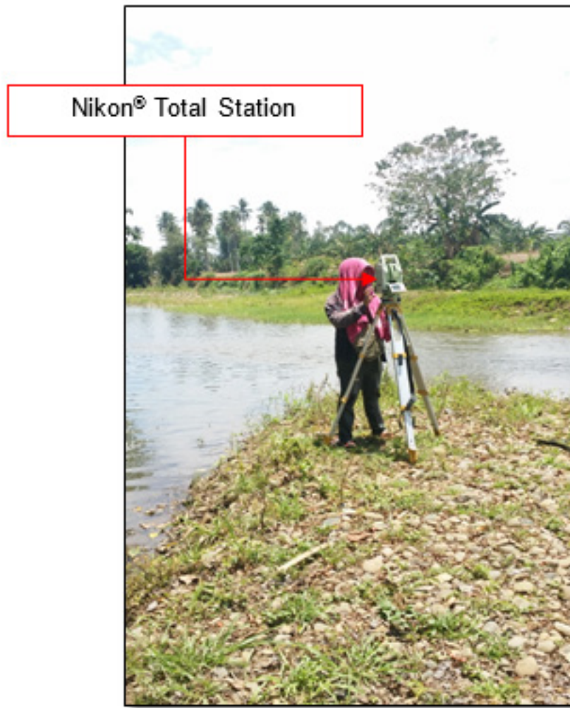
Figure 47. Manual bathymetric survey by the ABSD at the Saub River using a Nikon® Total Station.
