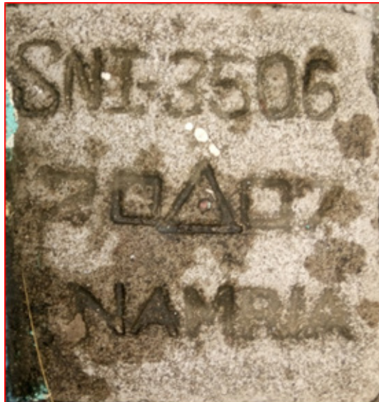
Figure 30. SNI-3506, a third-order GCP, located beside a flag pole inside Lomuyon Elementary School in Barangay Lomuyon, Kiamba, Sarangani.
