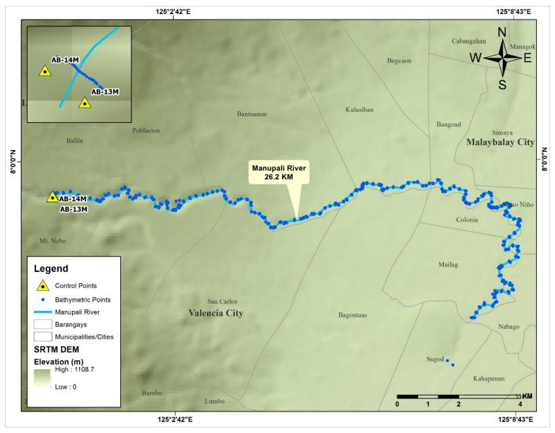
Figure 48. Bathymetric survey of Manupali River
