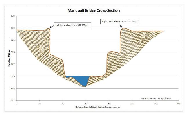
Figure 52. The cross-section plot of the Manupali Bridge
