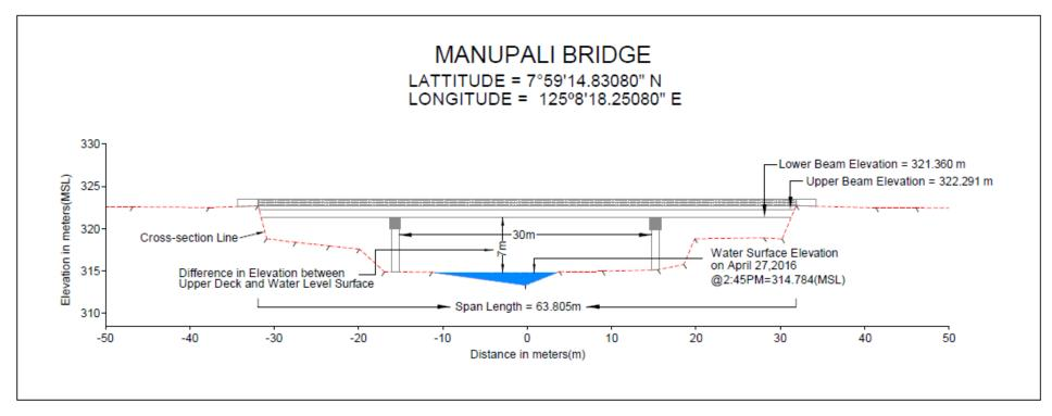
Figure 41. Manupali Bridge Cross-section Diagram
