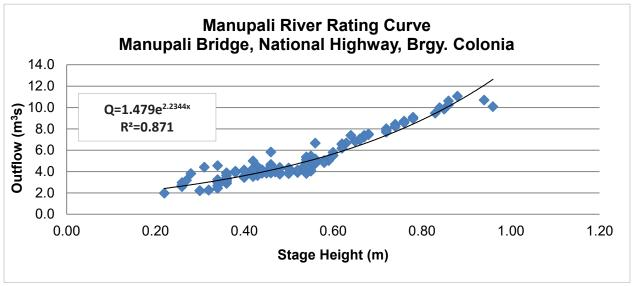
Figure 54. HQ Curve of HEC-HMS model.
