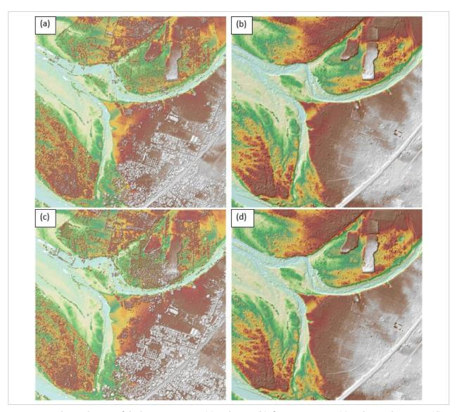
Figure 22. The production of the last return DSM (a) and DTM (b), first return DSM (c) and secondary DTM (d) in some portion of Manupali floodplain
