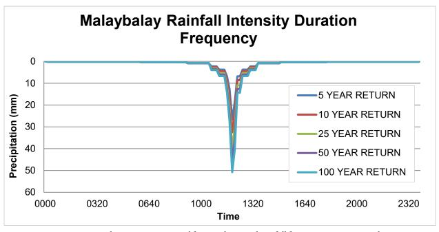
Figure 56. Synthetic storm generated for a 24-hr period rainfall for various return periods.
