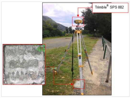
Figure 35. GNSS receiver set up, Trimble® SPS 882, at BK~56, located at the west post of the welcome arc of Malaybalay City in Brgy. Sumpong, Bukidnon
