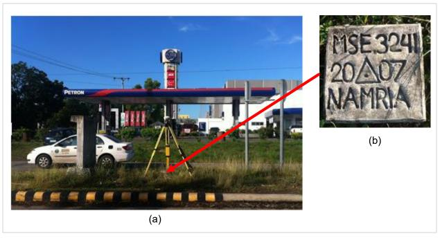
Figure 5. GPS set-up over MSE-3241 on a center island near a gasoline station beside SM Cagayan de Oro (a) and NAMRIA reference point MSE-3241 (b) as recovered by the field team.
