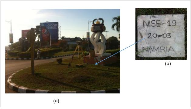
Figure 3. GPS set-up over MSE-19 at the center island located at the road intersections going to Cagayan de Oro, Butuan City and Iligan City (a) and NAMRIA reference point MSE-19 (b) as recovered by the field team.
