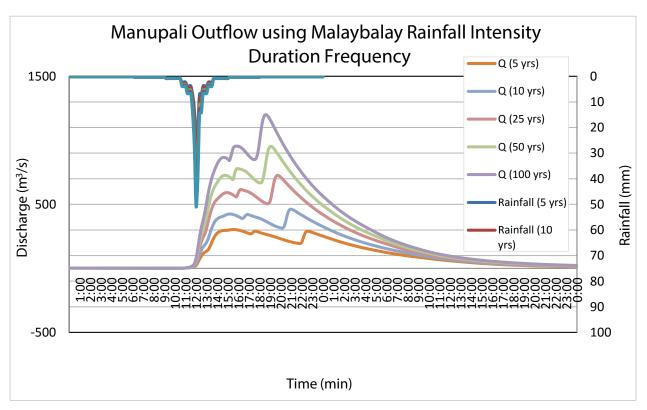
Figure 65. Outflow hydrograph at Manupali Station generated using Malaybalay RIDF simulated in HEC-HMS
