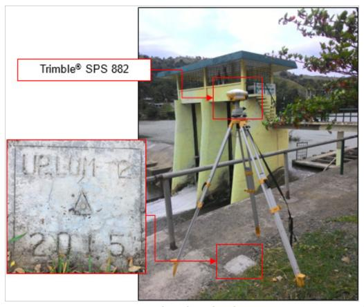
Figure 38. GNSS receiver serup, UP\_LUM-2, located near the Pulangui Diversion Dam in Brgy. Lumbayao, Valencia City, Province of Bukidnon.
