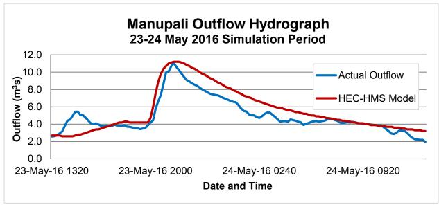
Figure 64. Outflow Hydrograph of Manupali produced by the HEC-HMS model compared with observed
