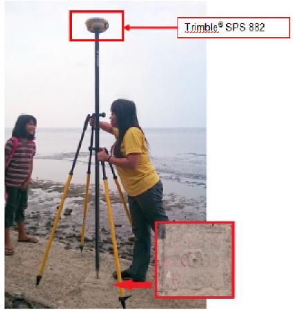
Figure 30. Trimble® SPS 882 GPS set-up at MSE-35, Brgy. Talisayan, Misamis Oriental
