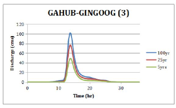
Figure 57. Gahub-Gingoog Rriver (3) generated discharge using 5-, 25-, and 100-year Lumbia rainfall intensity-duration-frequency (RIDF) in HEC-HMS
