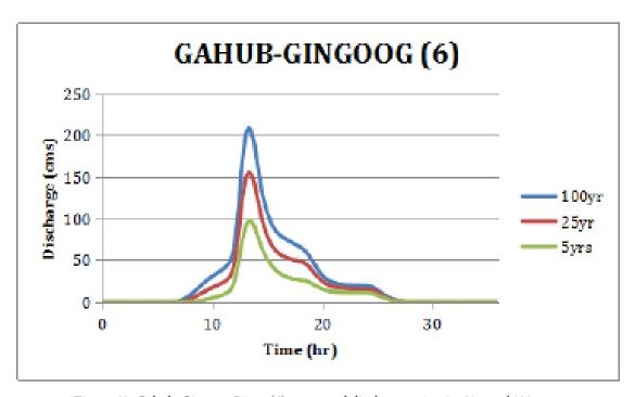
Figure 60. Gahub-Gingoog River (6) generated discharge using 5-, 25-, and 100-year Lumbia rainfall intensity-duration-frequency (RIDF) in HEC-HMS
