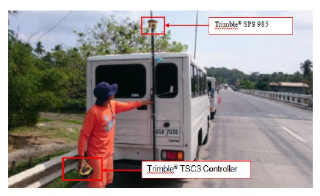
Figure 35. LiDAR Validation survey set up
