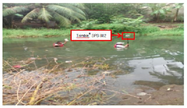
Figure 38. Set-up of manual bathymetricy survey for Gahub River using a Trimble® SPS 882 Rover
