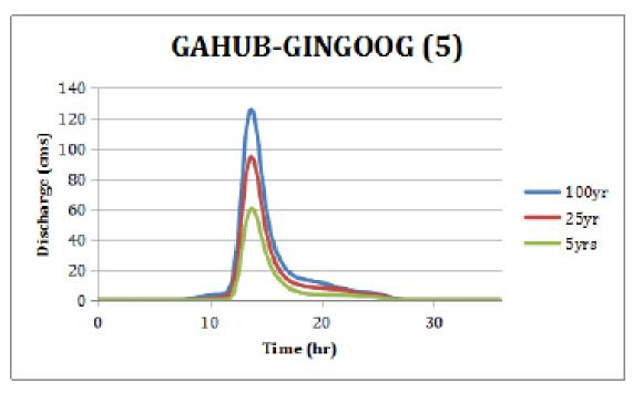
Figure 59. Gahub-Gingoog River (5) generated discharge using 5-, 25-, and 100-year Lumbia rainfall intensity-duration-frequency (RIDF) in HEC-HMS
