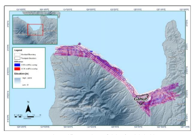
Figure 15. Elevation difference map between flight lines for Gahub Floodplain.
