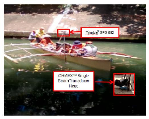
Figure 37. Bathymetric survey equipment set-up in a rented boat in Gahub River
