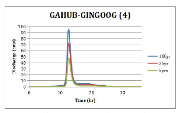
Figure 58. Gahub-Gingoog River (4) generated discharge using 5-, 25-, and 100-year Lumbia rainfall intensity-duration-frequency (RIDF) in HEC-HMS
