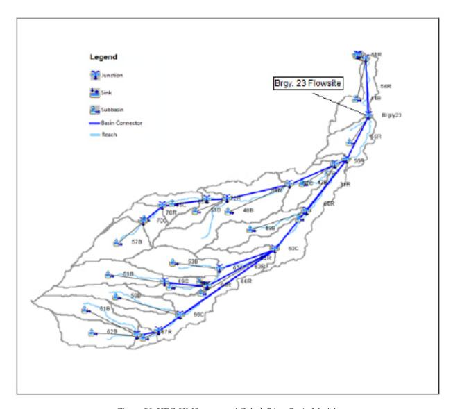
Figure 50. HEC-HMS generated Gahub River Basin Model
