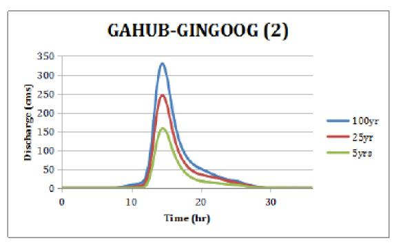
Figure 56. Gahub-Gingoog River (2) generated discharge using 5-, 25-, and 100-year Lumbia rainfall intensity-duration-frequency (RIDF) in HEC-HMS
