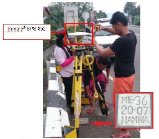
Figure 31.Trimble® SPS 852 Base set-up at ME-36, Gingoog Bridge located at Gingoog City
