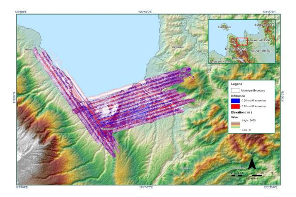
Figure A-8.7 Elevation difference between flight lines
