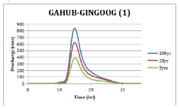
Figure 55. Gahub-Gingoog River (1) generated discharge using 5-, 25-, and 100-year Lumbia rainfall intensity-duration-frequency (RIDF) in HEC-HMS
