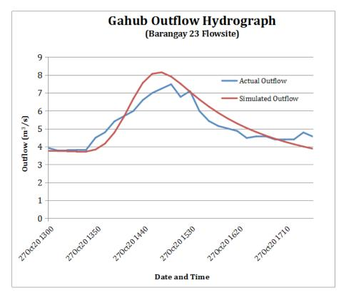
Figure 53. Outflow hydrograph of Gahub produced by the HEC-HMS model compared with observed outflow
