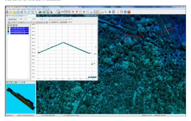
Figure 16. Quality checking for a Gahub flight 1521P using the Profile Tool of QT Modeler
