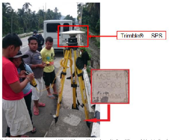
Figure 32. Trimble® SPS 852 Base set-up at MSE-44, Kibungsod Bridge, located in Brgy. Kibungsod, Municipality of Magsaysay
