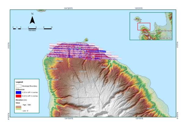
Figure A-8.21 Elevation difference between flight lines
