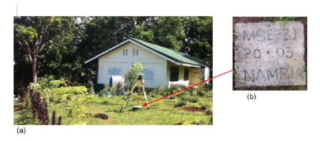
Figure 4. GPS set-up over MSE-31 inside the school grounds of Binuangan National High School of Sitio Naratulan, Binuangan, Misamis Oriental (a) and NAMRIA reference point MSE-31 (b) as recovered by the field team
