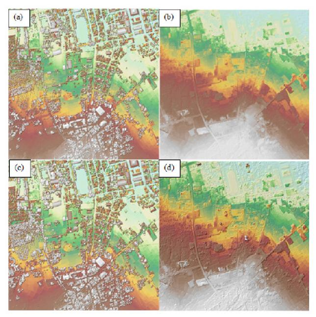
Figure 19. The production of last return DSM (a) and DTM (b), first return DSM (c) and secondary DTM (d) in some portion of Gahub Floodplain
