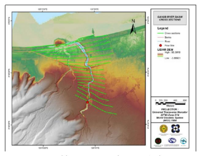
Figure 51. Gahub River Cross-section generated using HEC GeoRAS tool
