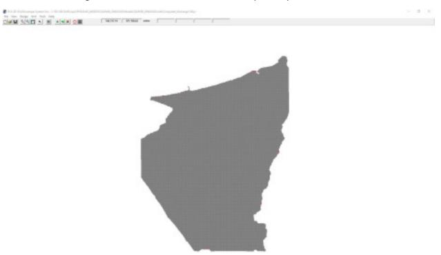
Figure 52. Screenshot of subcatchment with the computational area to be modeled in FLO-2DFLO-2D GDS Pro
