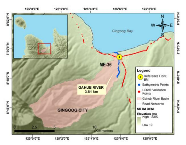
Figure 28. General survey area for Gahub River BasinExtent of the bathymetric survey (in blue) in Gahub River and the LiDAR data validation survey (in red)
