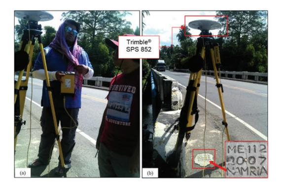
Figure 30. GNSS base receiver set-up, Trimble<sup>®</sup> SPS 852 at ME-112 at Musi-Musi Bridge in Brgy. Talusan, Municipality of Balingasag, Misamis Oriental
