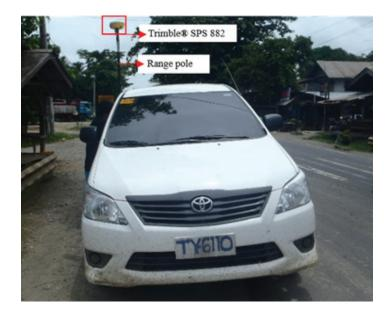
Figure 37. Validation points acquisition survey set-up on a vehicle using a Trimble® SPS 882, mounted on a 2 m pole attached to the side of the vehicle
