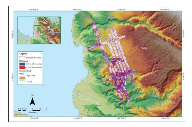
Figure A-8.14. Elevation difference between flight lines
