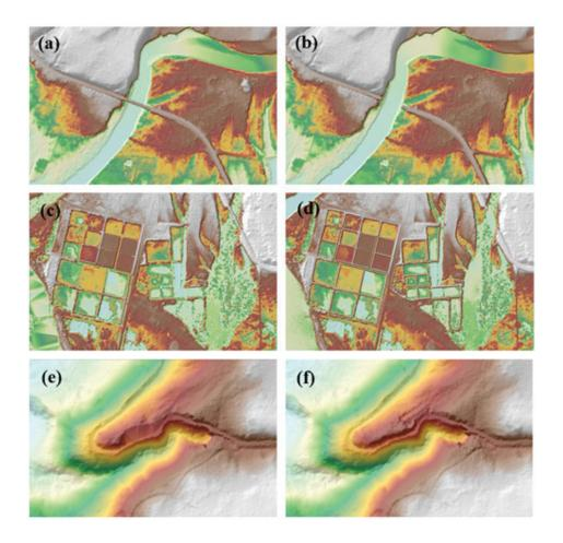
Figure 19. Portions in the DTM of Cabulig Floodplain – Cabulig bridge before (a) and after (b) interpolation; a paddy field before (c) and after (d) data retrieval; and a misclassified hill before (e) and after (f) data retrieval
