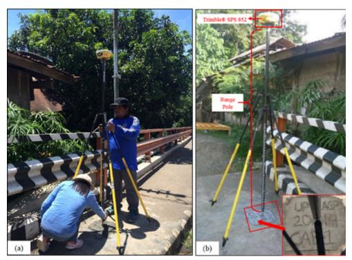
Figure 31. GNSS base occupation, Trimble<sup>®</sup> SPS 882 at CAB-1 along Iligan-Cagayan de Oro-Butuan Road at the approach of Cabulig Bridge in Brgy. Bobontugan, Municipality of Jasaan, Misamis Oriental
