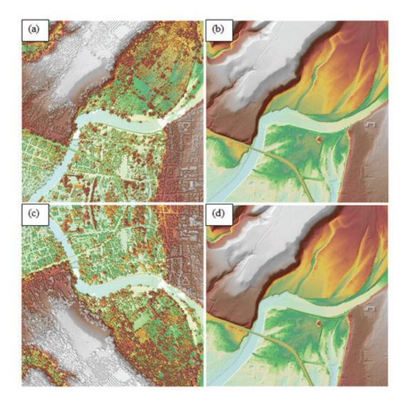
Figure 18. The production of last return DSM (a) and DTM (b), first return DSM (c) and secondary DTM (d) in some portion of Cabulig Floodplain.
