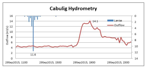
Figure 44. Rainfall and outflow data at Cabulig used for modeling
