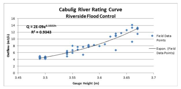
Figure 43. HQ curve of HEC-HMS model
