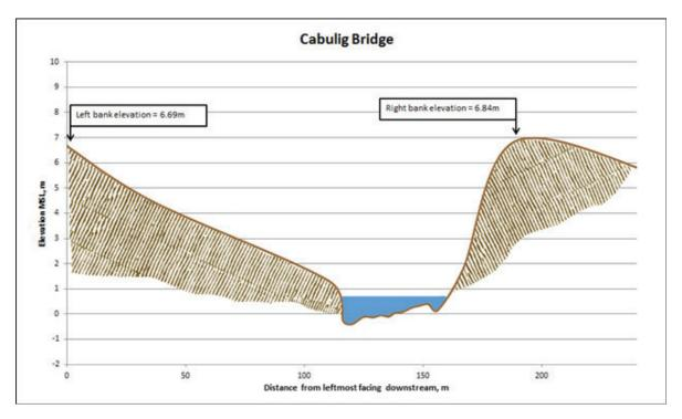
Figure 42. Cross-section plot of Cabulig Bridge
