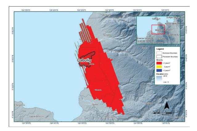
Figure 13. Density map of merged LiDAR data for Cabulig Floodplain
