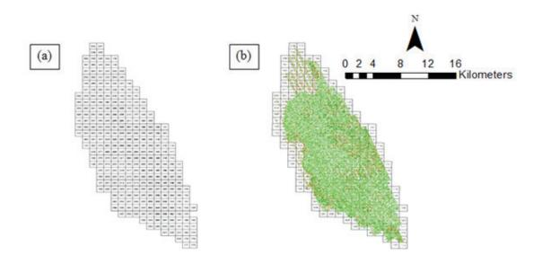
Figure 16. Tiles for Cabulig Floodplain (a) and classification results (b) in TerraScan
