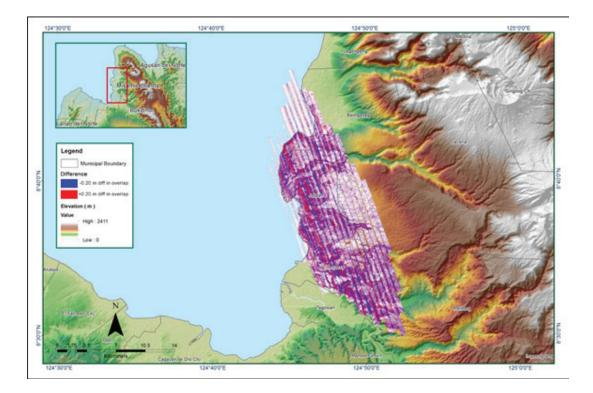
Figure A-8.7. Elevation difference between flight lines
