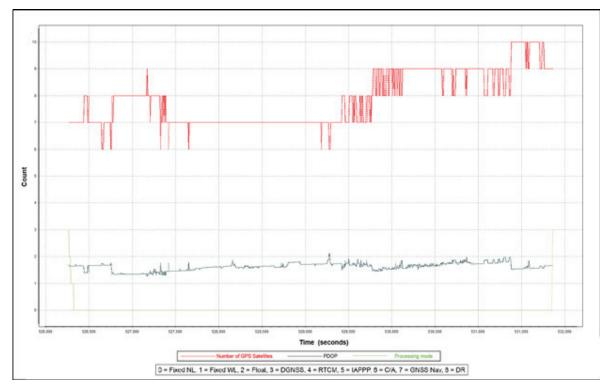
Figure 9. Solution Status Parameters of Cabulig Flight 1561P
