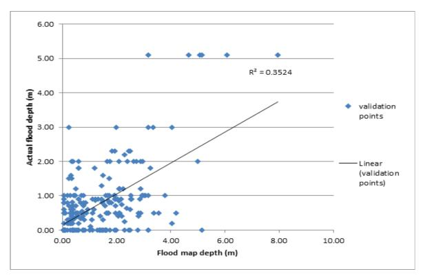
Figure 68. Flood map depth vs. actual flood depth
