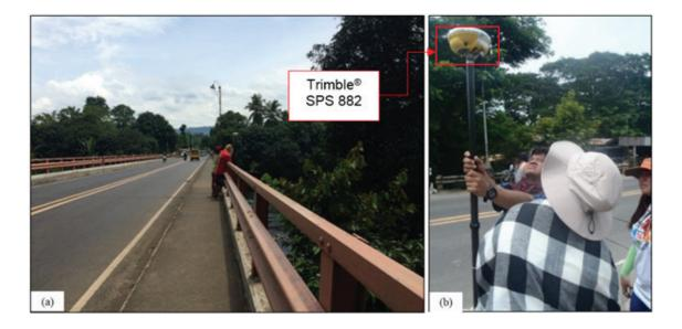
Figure 32. GNSS base occupation, Trimble<sup>®</sup> SPS 882 at CAB-1 along Iligan-Cagayan de Oro-Butuan Road at the approach of Cabulig Bridge in Brgy. Bobontugan, Municipality of Jasaan, Misamis Oriental
