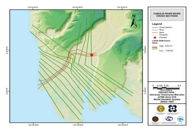
Figure 52. River cross-section of Cabulig River generated through Arcmap HEC GeoRAS tool
