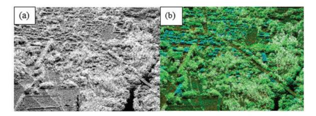
Figure 17. Point cloud before (a) and after (b) classification
