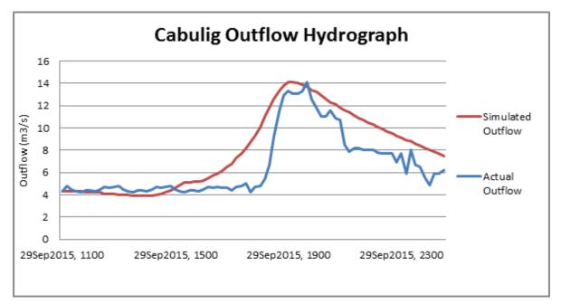
Figure 54. Outflow hydrograph of Cabulig produced by the HEC-HMS model compared with observed outflow
