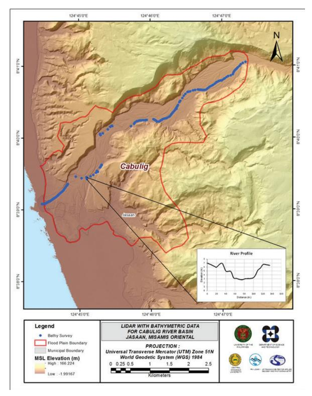
Figure 24. Map of Cabulig Floodplain with bathymetric survey points shown in blue
