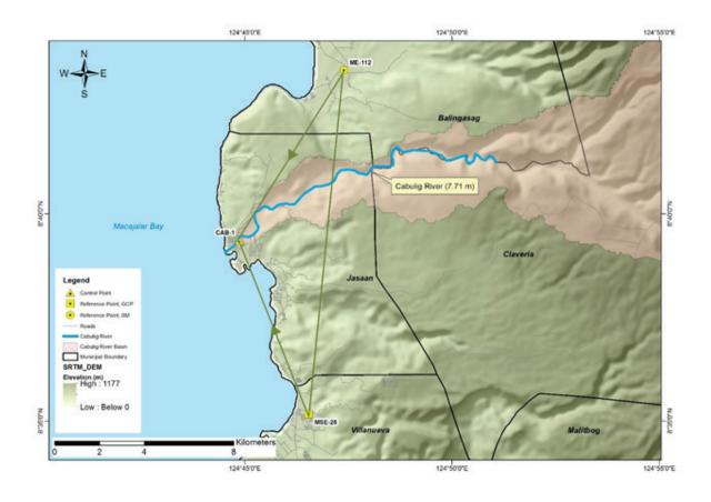
Figure 28. GNSS network of Cabulig River field survey
