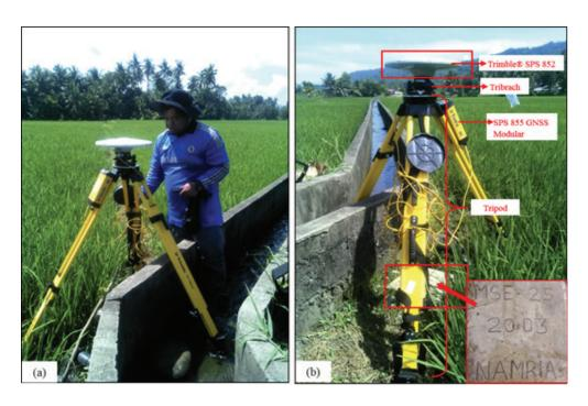
Figure 29. GNSS base receiver set-up, Trimble<sup>®</sup> SPS 852 at MSE-25 in Brgy. Poblacion 1, Municipality of Villanueva, Misamis Oriental
