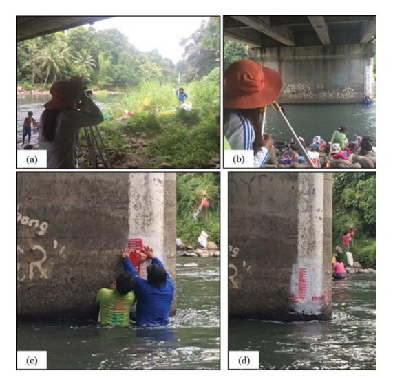
Figure 36. Water surface elevation marking in Cabulig Bridge
