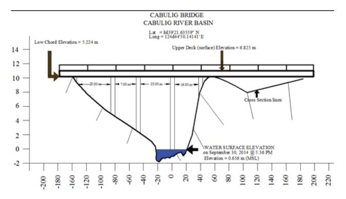
Figure 34. Cross-section diagram of Cabulig Bridge
