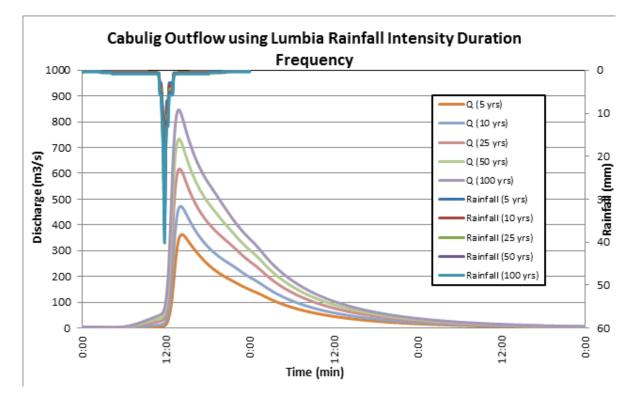
Figure 55. Outflow hydrograph at Cabulig Station generated using Lumbia RIDF simulated in HEC-HMS
