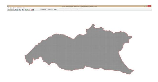
Figure 53. Screenshot of subcatchment with the computational area to be modeled in FLO-2D GDS Pro
