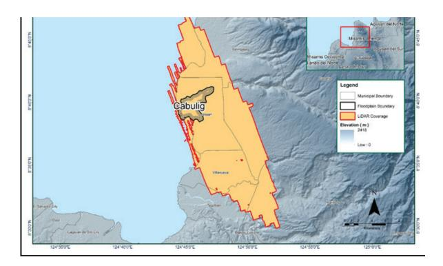
Figure 11. Boundary of the processed LiDAR data over Cabulig Floodplain
