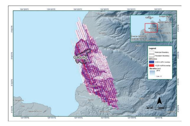
Figure 14. Elevation difference map between flight lines for Cabulig Floodplain
