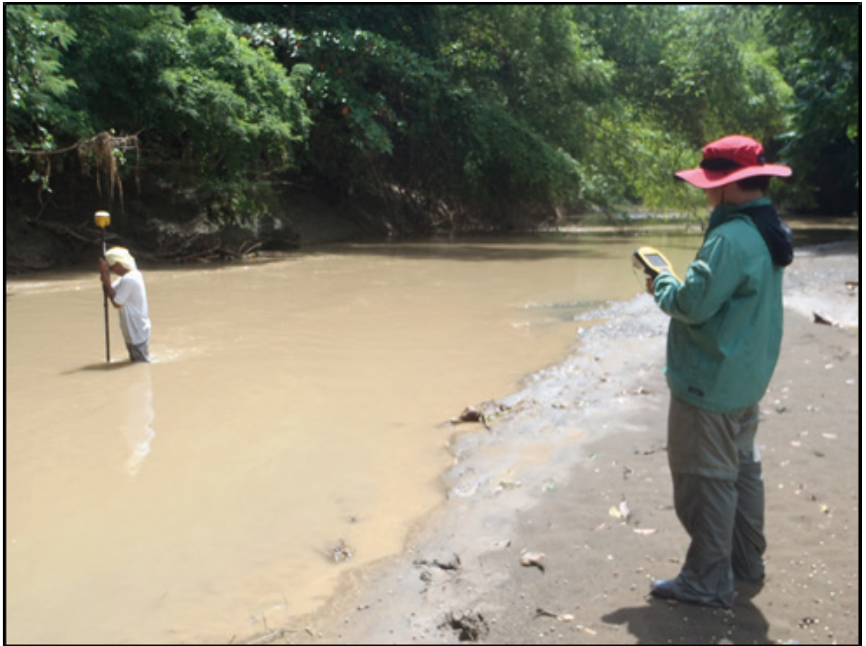
Figure 41. Manual bathymetry in the shallow portion of Alubijid River.
