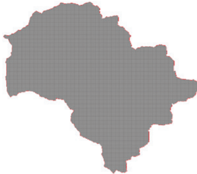
Figure 55. Screenshot of subcatchment with the computational area to be modeled in FLO-2D GDS Pro.
