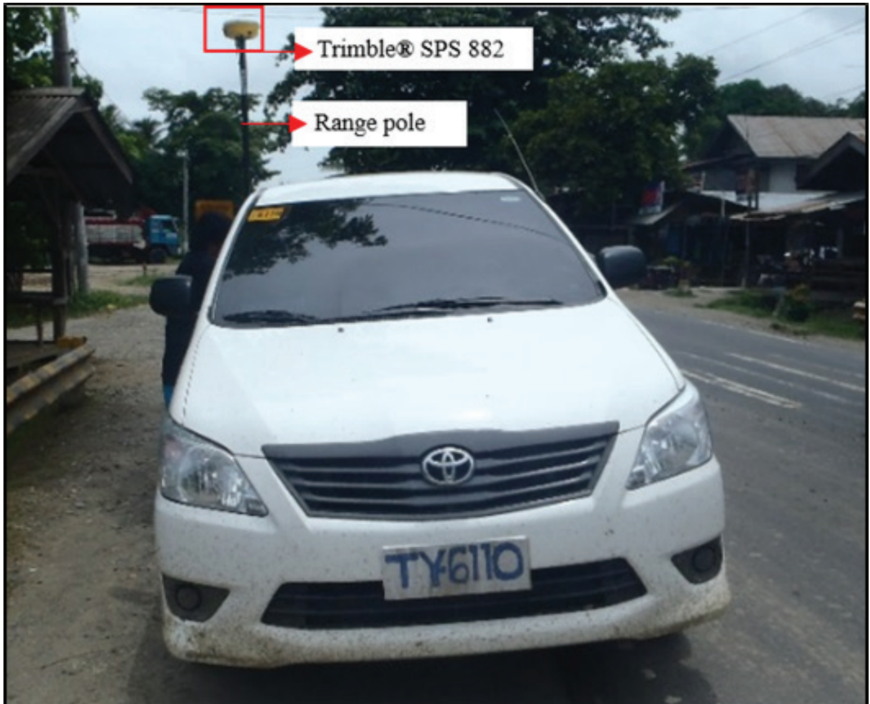
Figure 39. Trimble SPS®882 set-up in a vehicle in Alubijid River.
