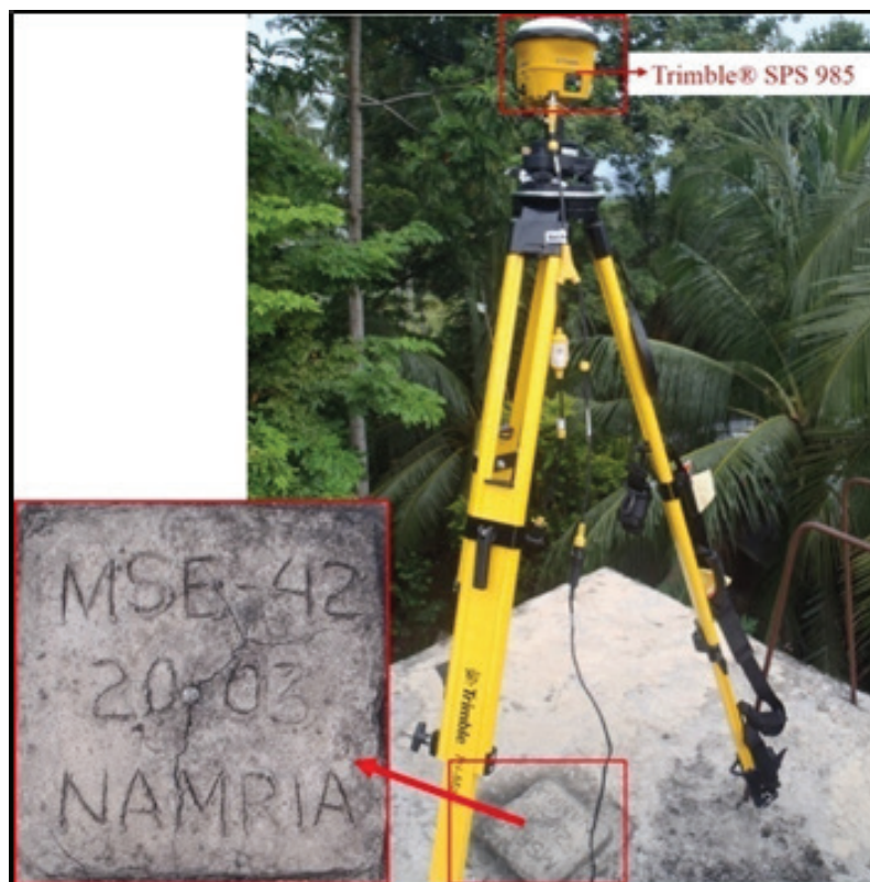
Figure 32. GNSS receiver Trimble® SPS 985 setup, at MSE-42 on the concrete water tank behind the Molocaboloc Barangay Hall, Municipality of Alubijid.
