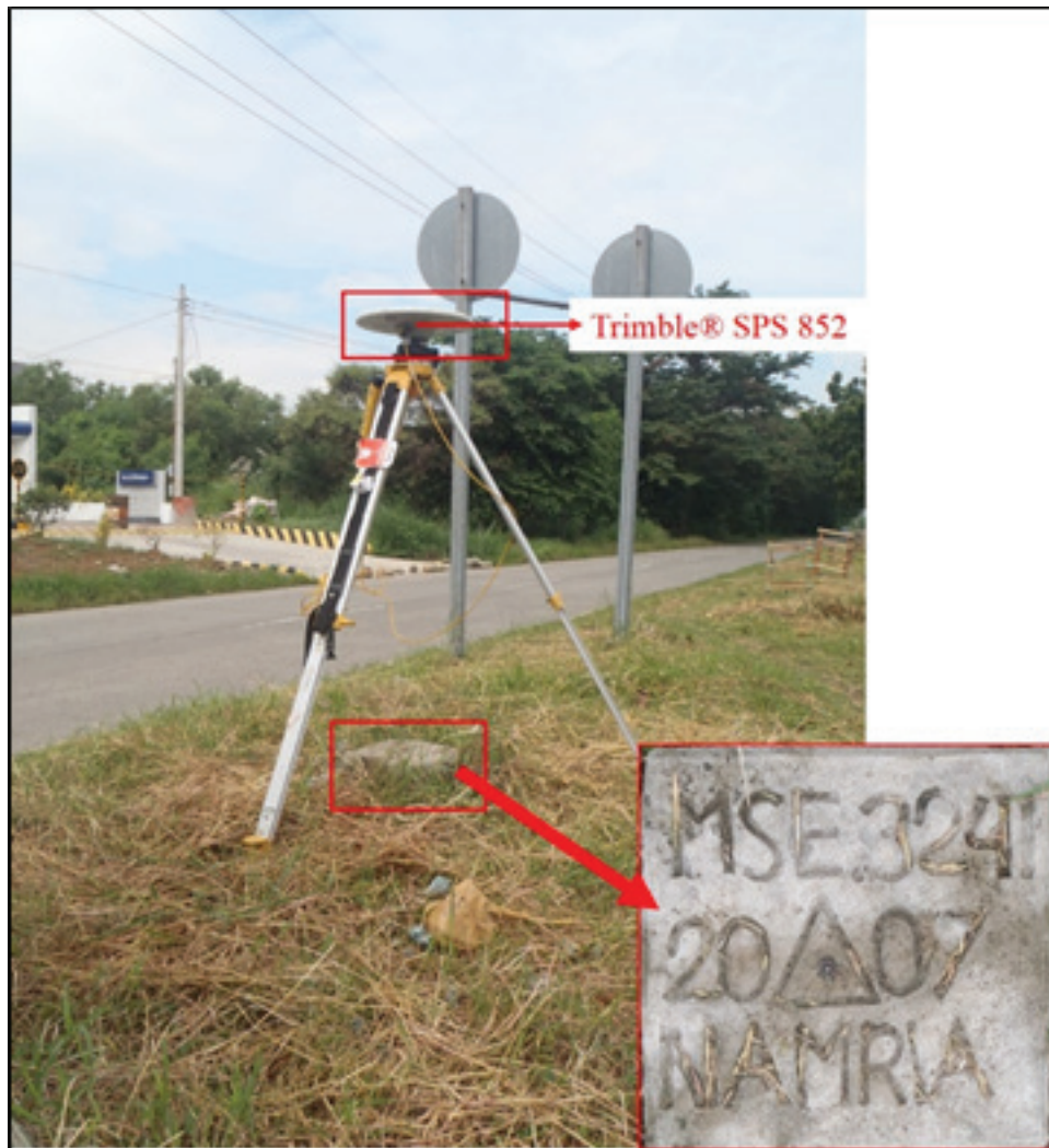
Figure 33. GNSS receiver Trimble® SPS 852 setup at MSE-3241 in Brgy. 10 (POB), Cagayan de Oro City.
