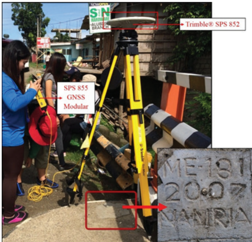
Figure 31. GNSS receiver, Trimble® SPS 852, setup at ME-181 in Alubijid Bridge, Brgy. Poblacion, Alubijid.
