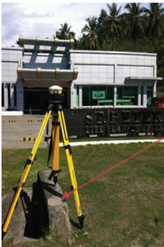
Figure 5. GPS set-up over LE-89 in front of St. Peter Life Plan of Iligan City, Lanao del Norte (a) and NAMRIA benchmark AN-44 (b) as recovered by the field team.
