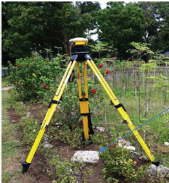
Figure 4. GPS set-up over MSE-17 inside the school grounds of Pangayawan Elementary School in Gitagum, Misamis Oriental (a) and NAMRIA reference point MSE-17 (b) as recovered by the field team.
