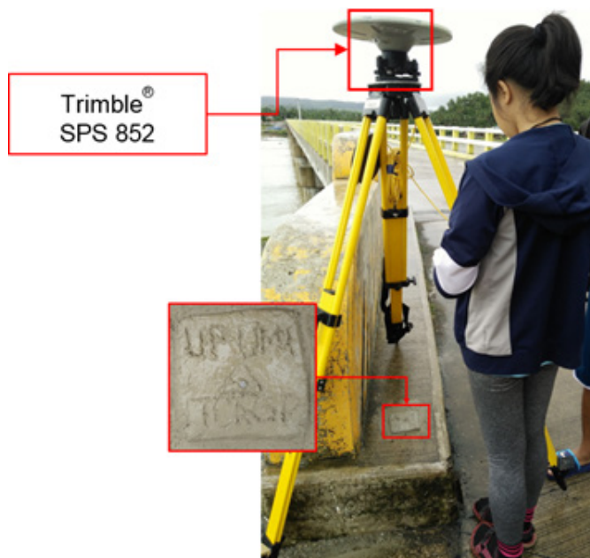
Figure 33. GNSS receiver set-up, Trimble® SPS 852, at UP-UMI, located at the deck of the Umiray Bridge in Barangay Umiray, Municipality of Dingalan, Aurora
