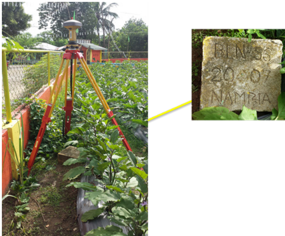
Figure 4. (a) GPS set-up over BLN-56, located within Casalat Elementary School, about 24 meters SSW of the main gate and about 0.5 meters E of the concrete fence in Barangay Casalat, San Idelfonso; and (b) NAMRIA reference point BLN-56, as recovered by the field
