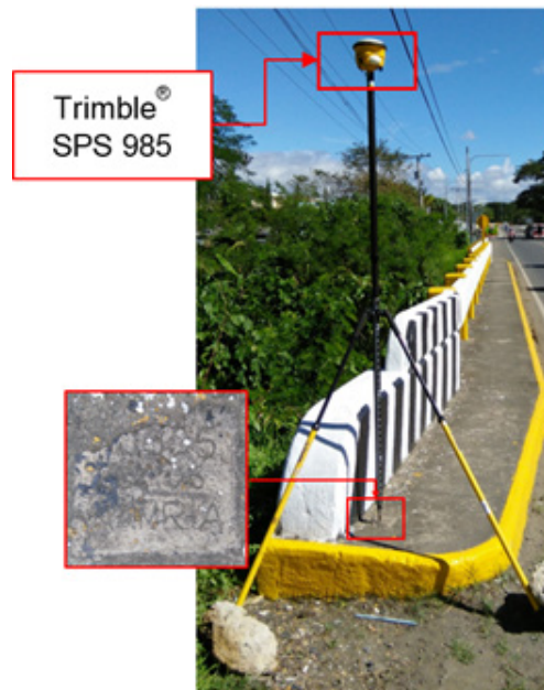
Figure 32. GNSS base set-up, Trimble® SPS 985, at NJ-305, located along the national road in Barangay Atate, Palayan City, Nueva Ecija.
