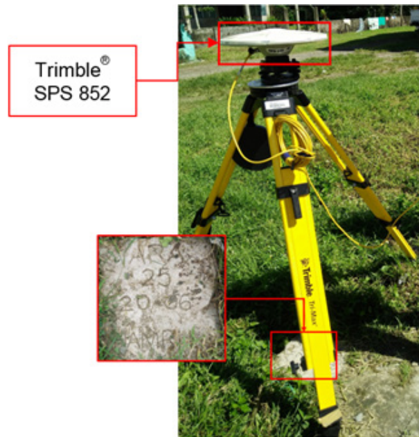
Figure 31. GNSS receiver set-up, Trimble® SPS 852, at ARA-25, located near the covered court inside the barangay complex of Barangay Ibuna, Municipality of Dingalan, Aurora.
