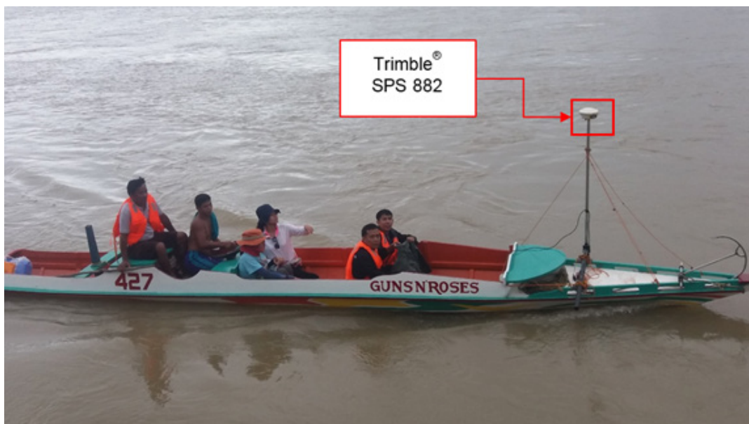
Figure 42. Bathymetric survey using a Trimble® SPS 882 in GNSS PPK survey technique in the Umiray River
