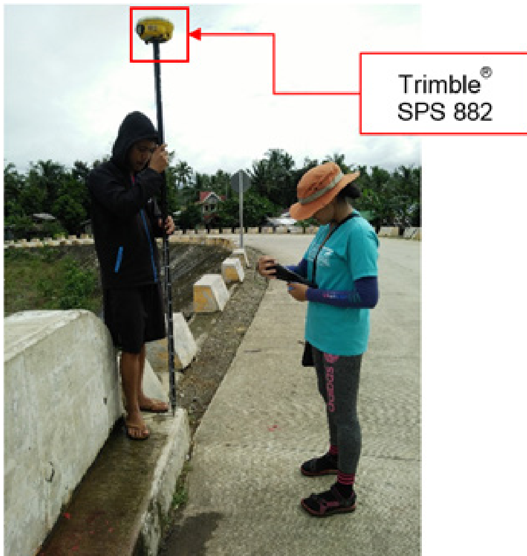
Figure 35. As-built survey of the Umiray Bridge.
