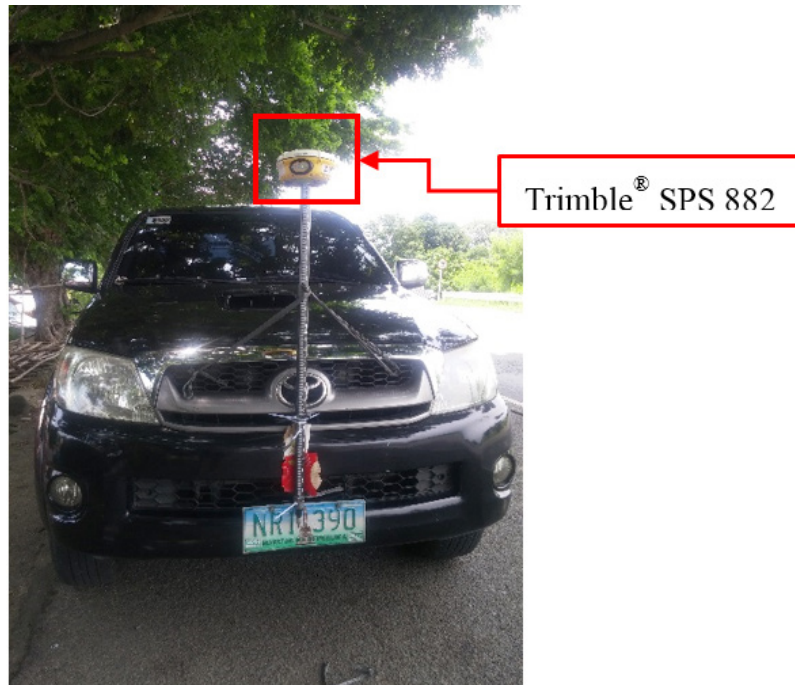
Figure 40. Validation points acquisition survey set up along MorongRiver Basin
