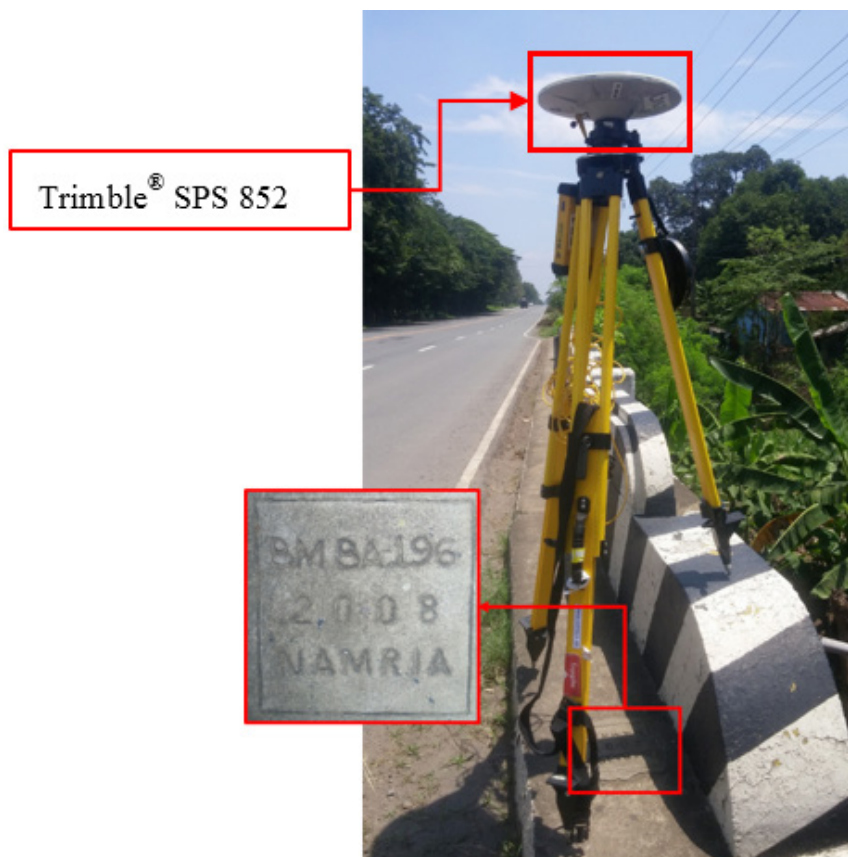
Figure 33. GNSS receiver setup, Trimble® SPS 852, at BA-196 located at the approach of CapitanganBridge in Brgy. Capitangan, Municipality of Abucay, Bataan
