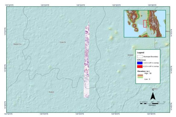
Figure 1.9.7 Elevation Difference Between flight lines
