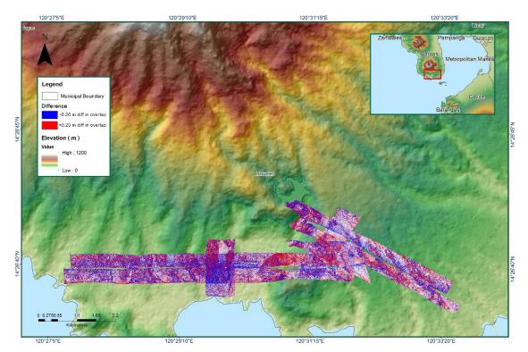
Figure 1.6.7 Elevation difference between flight lines
