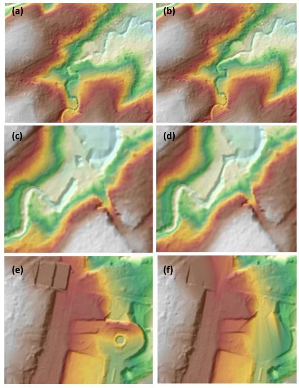
Figure 21.Portions in the DTM of Balanga floodplain – river embankments before (a) and after (b) interpolation; bridge before (c) and after (d) manual editing; and building before (e) and after (f) manual editing.
