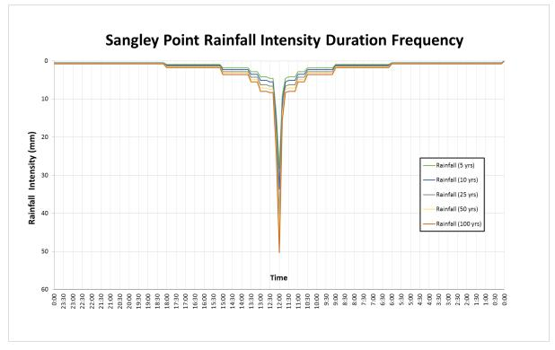
Figure 52. Synthetic storm generated for a 24-hr period rainfall for various return periods
