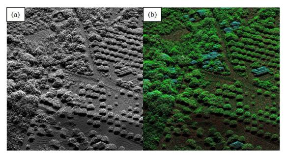
Figure 17. Point cloud before (a) and after (b) classification.
