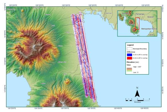
Figure 1.4.7. Elevation difference between flight line
