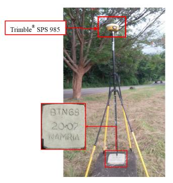
Figure 32.GNSS base set up, Trimble<sup>®</sup> SPS 882, at BTN-68, located just outside the Bataan Nuclear Power Plant along National High Way, Brgy. Nagbalayong, Municipality of Morong, Bataan
