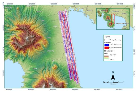
Figure 1.3.7. Elevation difference between flight lines
