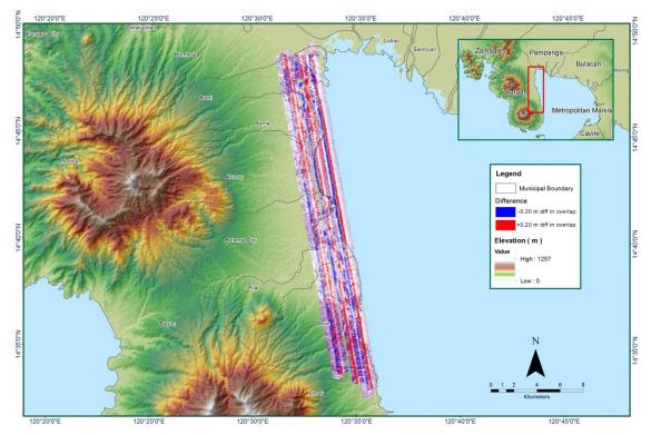
Figure 1.2.7. Elevation difference between flight lines
