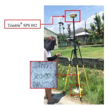
Figure 33.GNSS receiver setup, Trimble<sup>®</sup> SPS 882, at BTN-71, located at the middle of basketball court, Barangay Day Care Center and Barangay Chapel in Brgy. Apollo, Municipality of Orani, Bataan
