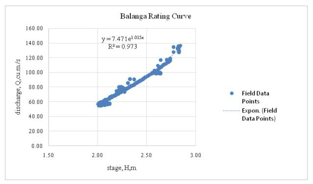
Figure 49. Rating Curve at Talisay Bridge, Balanga, Bataan
