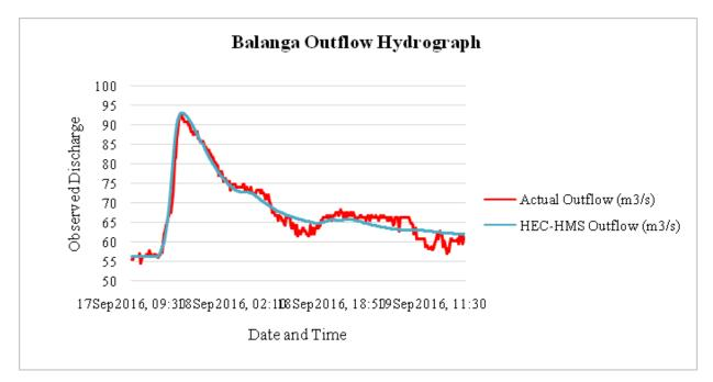
Figure 60.Outflow Hydrograph of Balanga produced by the HEC-HMS model compared with observed outflow
