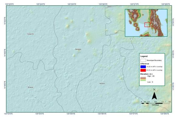
Figure 1.8.7 Elevation Difference Between flight lines
