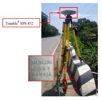
Figure 34.GNSS receiver setup, Trimble<sup>®</sup> SPS 852, at BA-196, located at the approach of Capitangan Bridge in Brgy. Capitangan, Municipality of Abucay, Bataan
