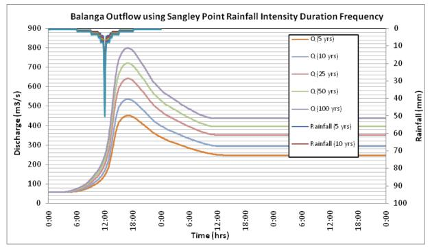
Figure 61.Outflow hydrograph at Balanga Station generated using Sangley Point RIDF simulated in HEC HMS
