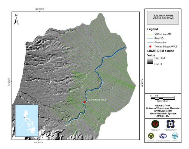
Figure 58. River cross-section of Balanga River generated through Arcmap HEC GeoRAS tool
