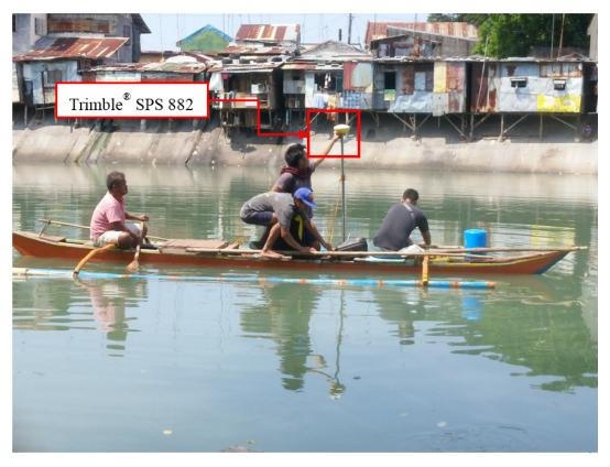
Figure 44. Bathymetric survey using Ohmex<sup>™</sup> single beam echo sounder in Talisay River
