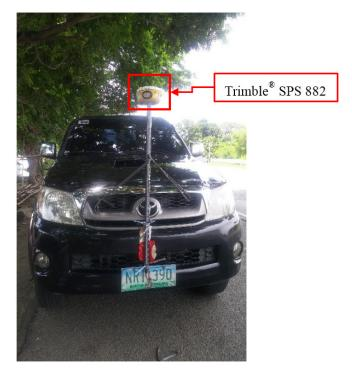
Figure 42.Validation points acquisition survey set up along Talisay River Basin
