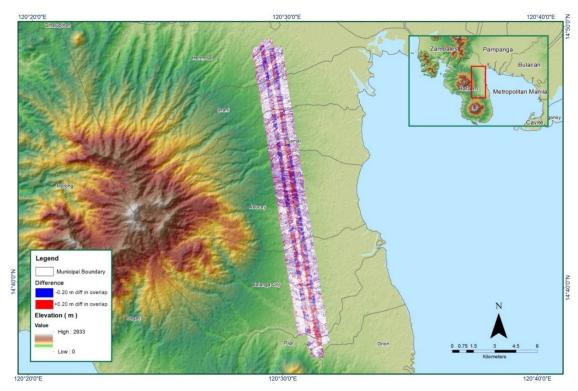
Figure 1.1.7. Elevation difference between flight lines
