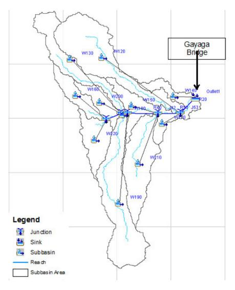
Figure 57. The Balanga river basin model generated using HEC-HMS
