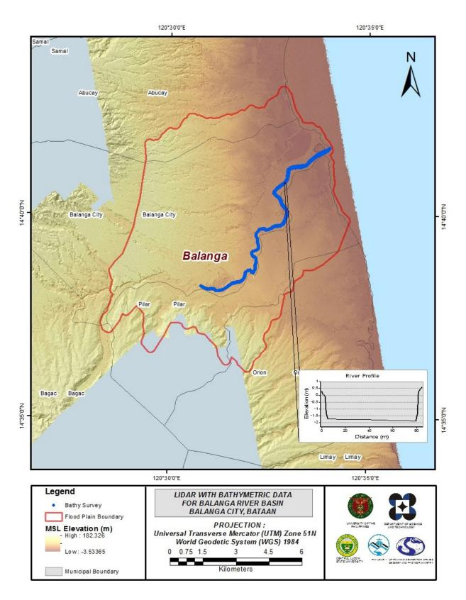
Figure 26. Map of Balanga Flood Plain with bathymetric survey points shown in blue.
