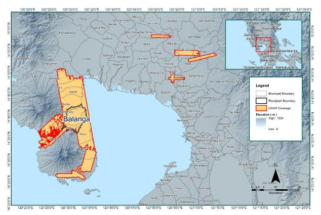
Figure 11. Boundaries of the processed LiDAR data on top of a SAR Elevation Data over Balanga Floodplain.
