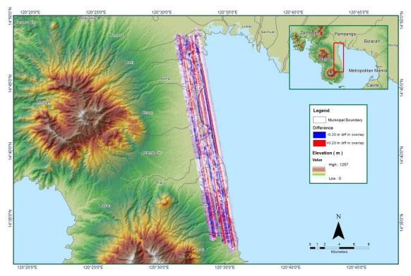
Figure 1.5.7. Elevation difference between flight lines
