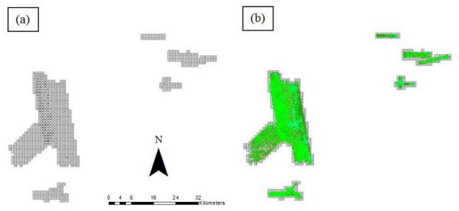
Figure 16. Tiles for Balanga floodplain (a) and classification results (b) in TerraScan.
