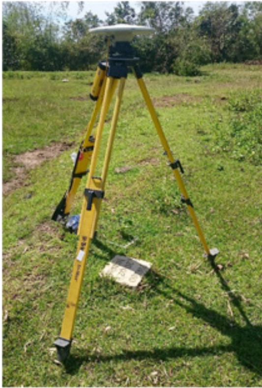
Figure 4. GPS set-up over PNG-80 located on the open ground west of the academics compound of Burgos National Highschool Brgy. Don Matias, Pangasinan (a) and NAMRIA reference point PNG-80 (b) as recovered by the field team
