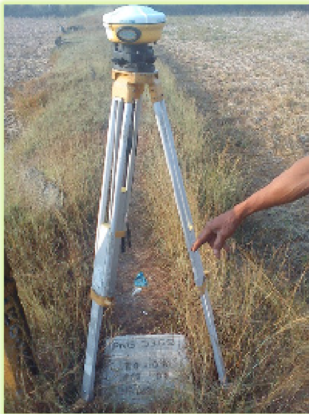
Figure 5. GPS set-up over PNG-3369 located beside DPWH kilometer post in Brgy. Banog, Pangasinan (a) and NAMRIA reference point PNG-3369 (b) as recovered by the field team
