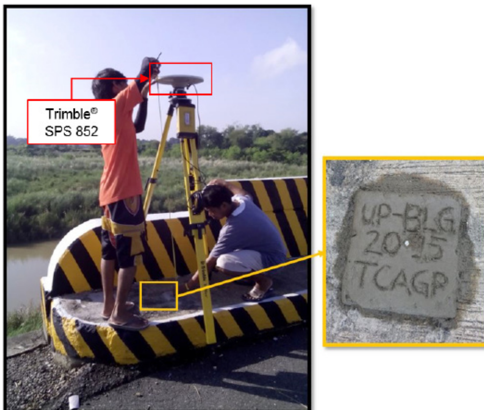
Figure 34. GNSS base receiver set-up, Trimble® SPS 852 at UP-BLG in Baloling Bridge, Municipality of Mapandan, Pangasinan
