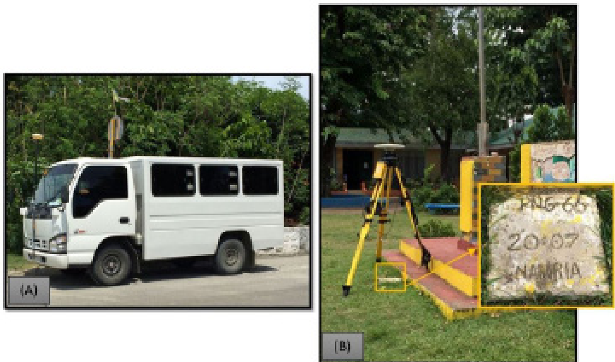
Figure 42. (A) Set-up of Trimble® SPS 882 attached to a vehicle and (B) Setting up of GNSS base station at PNG-66
