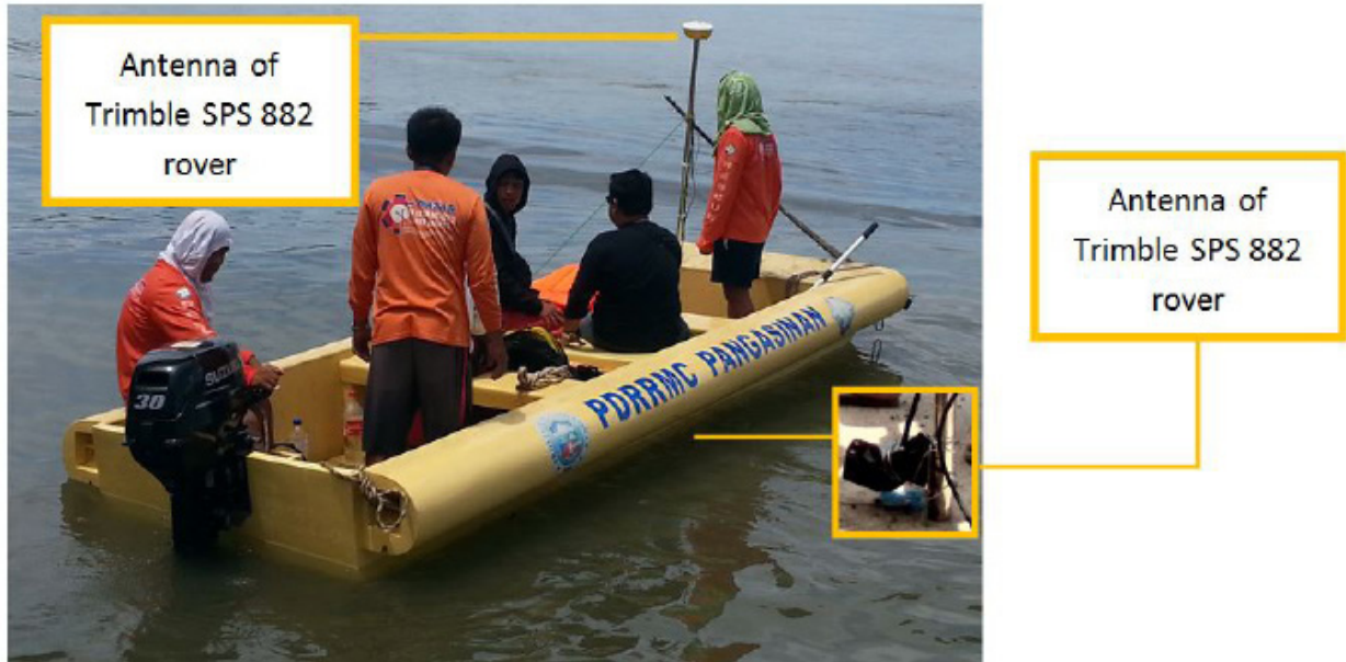
Figure 44. Bathymetric survey using OHMEX™ echo sounder
