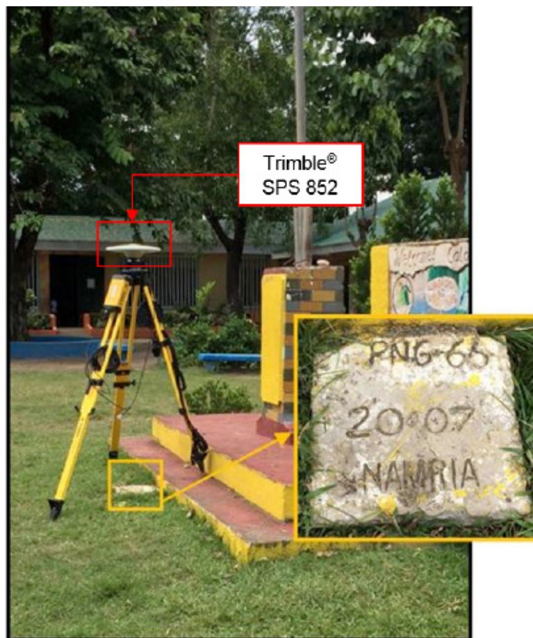
Figure 31. GNSS base receiver set-up, Trimble® SPS 852 at PNG-66 in Calamboyan Elementary School, San Carlos City, Pangasinan
