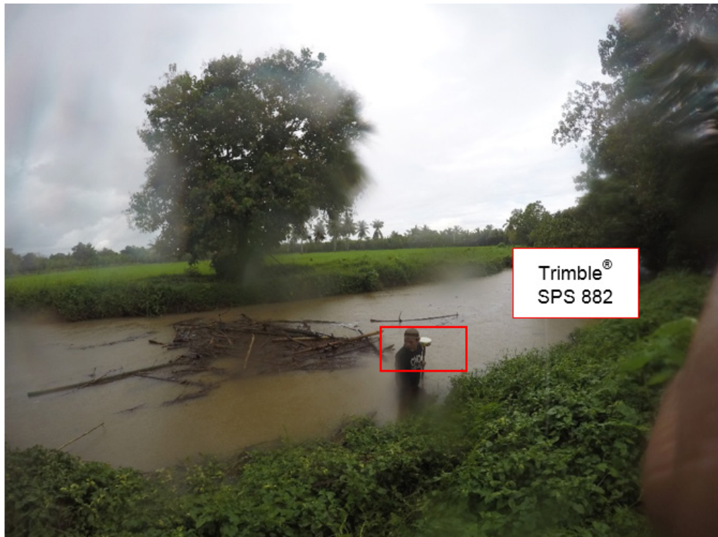
Figure 46. Bathymetric survey using PPK technique set-up in Tupilac River
