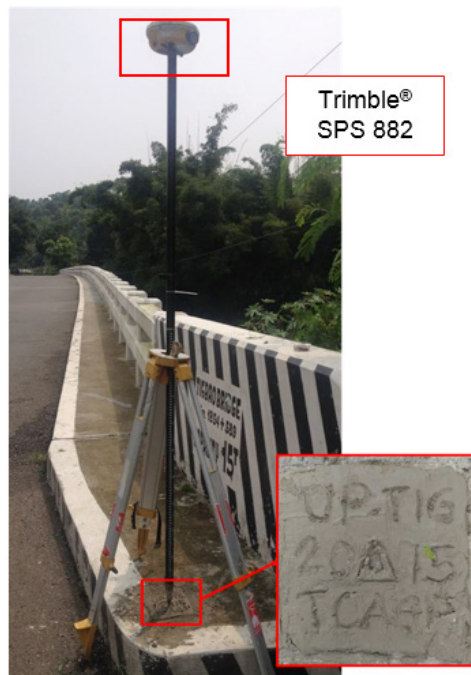
Figure 31. GNSS base set up, Trimble® SPS 882, at UP-TIG, located at the approach of Tigbao Bridge, Brgy. Tictapul, Zamboanga City, Zamboanga Del Sur
