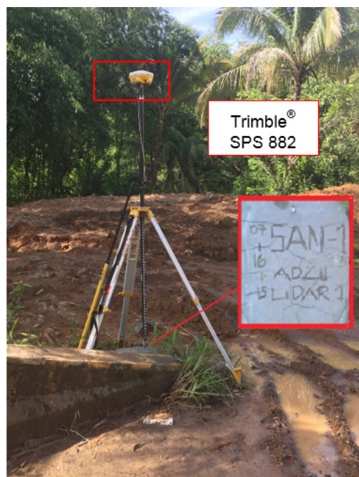
Figure 33. GNSS base set up, Trimble® SPS 882, at SAN-1, located at the approach of an unknown bridge found between Alibutdan and Diversion Rd, in Brgy. Pangi, Municipality of Ipi, Zamboanga Sibugay
