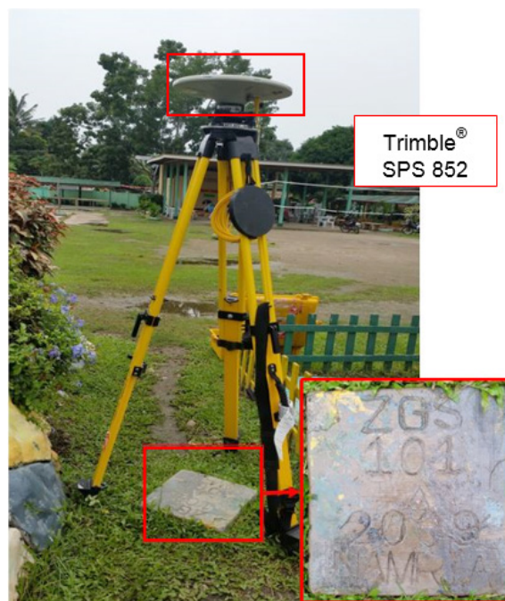
Figure 37. GNSS base set up, Trimble® SPS 852, at ZGS-101, located inside Brgy. Bolong Elementary School, Zamboanga City, Zamboanga Del Sur
