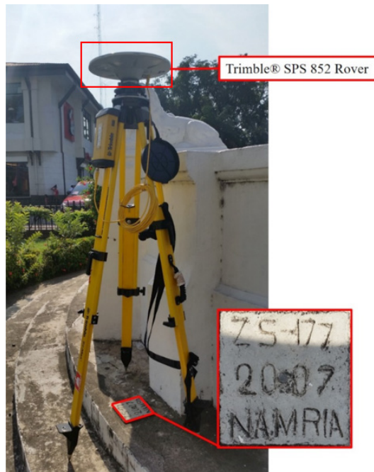
Figure 38. GNSS base set up, Trimble® SPS 852, at ZS-177, located at the stair of Rizal’s Park along the Butuan-Zamboanga National Road, Brgy Zone 4, Zamboanga City, Zamboanga Del Sur
