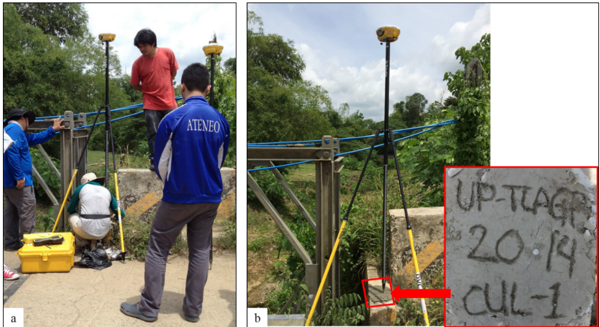
Figure 36. GNSS base receiver setup, Trimble® SPS 882 at CUL-1 along approach of Culianan Bridge in Brgy. Culianan, Zamboanga City, Zamboanga Del Sur
