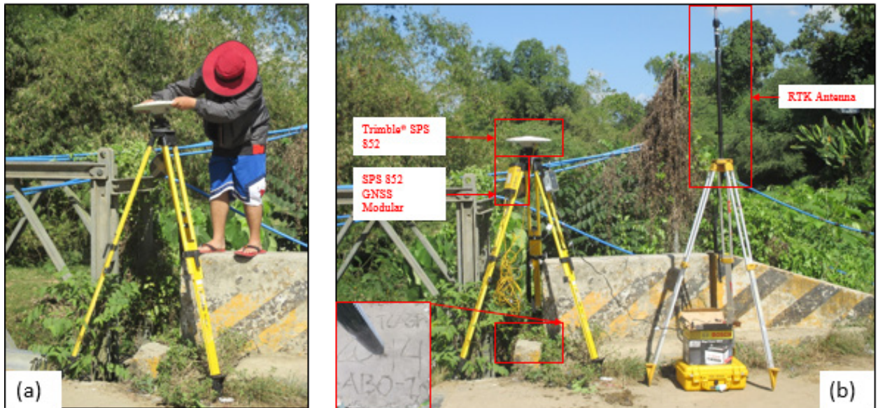
Figure 35. GNSS receiver occupation, Trimble® SPS 852 at ABO-1 located along approach of Abong Bridge, in Brgy. Dulian, Zamboanga City, Zamboanga Del Sur
