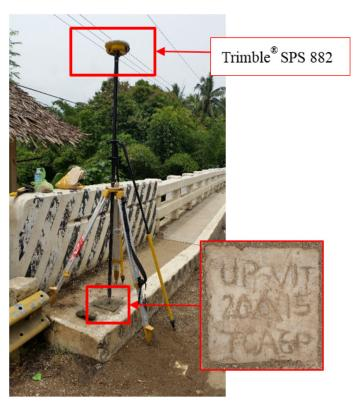
Figure 40. Trimble® SPS 882 set-up at UP-VIT located at the approach of Vitali Bridge in Brgy. Vitali, Zamboanga City
