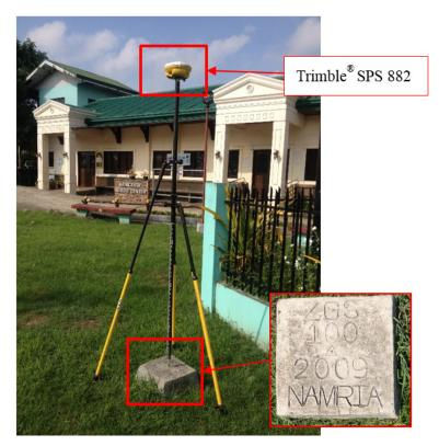
Figure 36.Trimble SPS® 882 set-up at ZGS-100 located at Manicahan Barangay Hall, Zamboanga City
