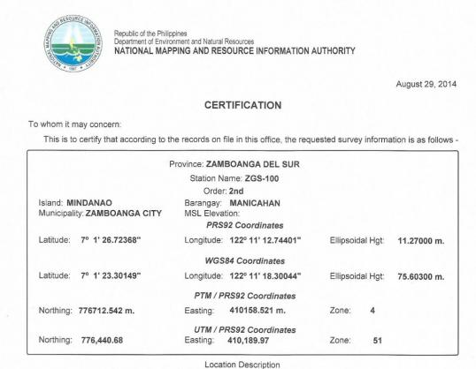
The station is marked by an 4" copper nail with its head flushed at the center of an cement putty on a concrete open canal with inscription " ZGS-100, 2009 NAMRIA".Located at Manicahan Barangay Hal 7 meters South from the flag pole 7 meters km post 1916-ZC22
