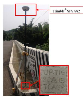
Figure 39.Trimble SPS® 882 set-up at UP-TIG located at the approach of Tigbao Bridge in Brgy. Tictapul, Zamboanga City
