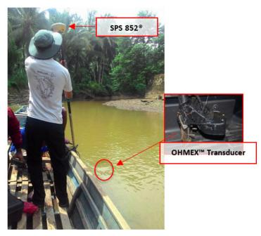
Figure 49. OHMEX<sup>™</sup> single beam echo sounder set up on a boat for Tigbao River bathymetric survey
