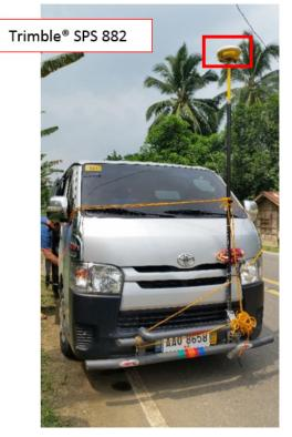
Figure 47. Trimble® SPS 882 set-up for validation points acquisition survey
