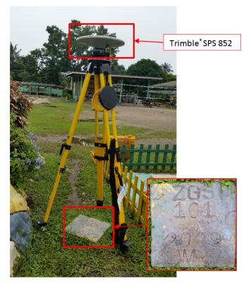
Figure 34. Trimble® SPS 852 set-up at ZGS-101 located at Bolong Elementary School, Brgy. Bolong, Zamboanga City
