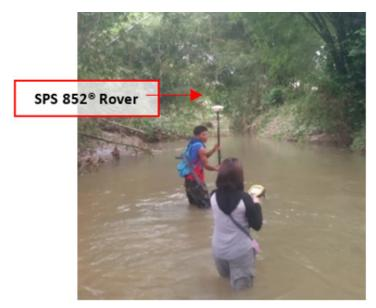
Figure 50. Manual bathymetry survey for Tigbao River
