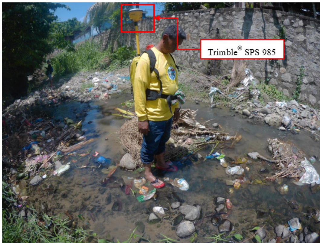
Figure 46. Bathymetric survey using Trimble® SPS 985 in GNSS PPK survey technique in Townsville River
