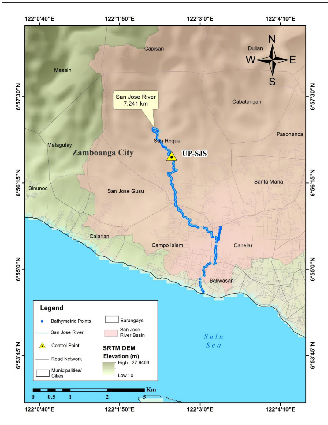
Figure 48. Bathymetric survey of San Jose River
