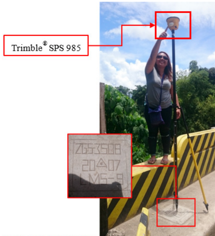
Figure 34. GNSS base set-up, Trimble® SPS 985, at ZGS-99 located beside a seawall at Airforce Beach, Brgy. Sinunoc, Zamboanga City, Zamboanga Del Sur
