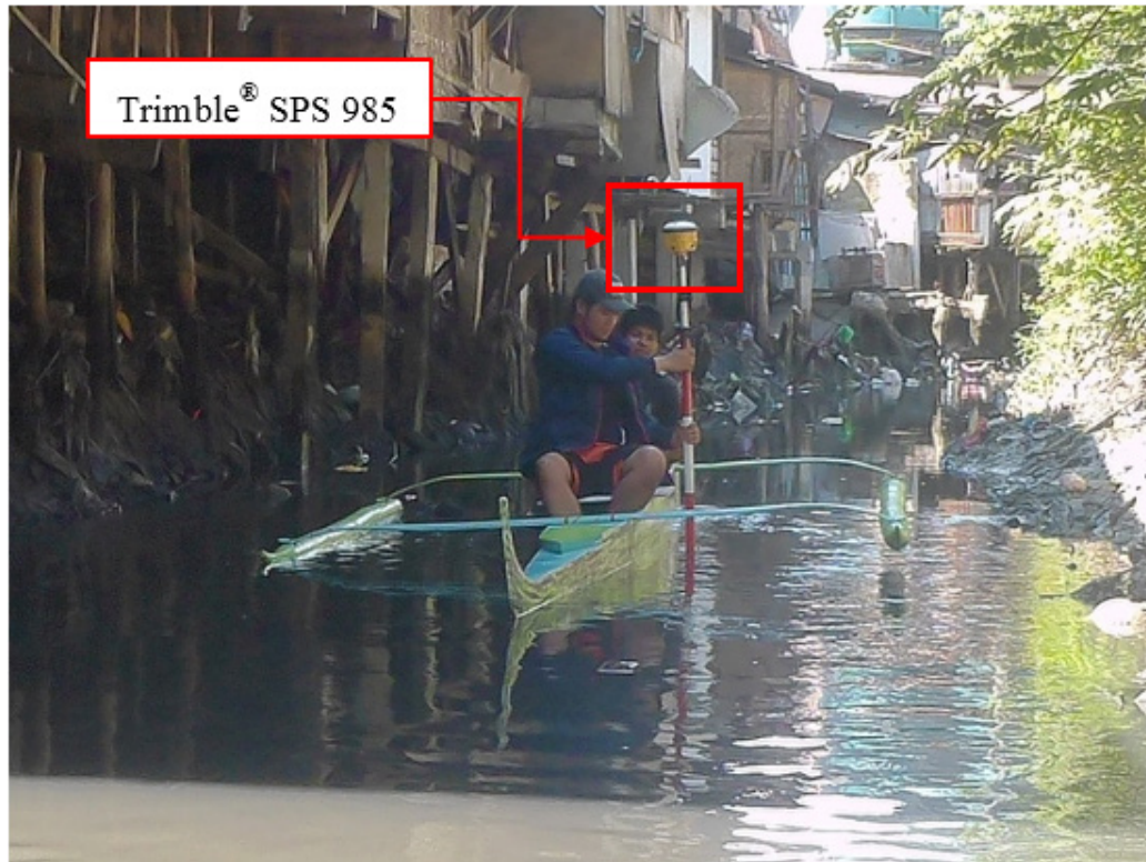
Figure 45. Bathymetric survey using OHMEX™ single beam echo sounder in San Jose River
