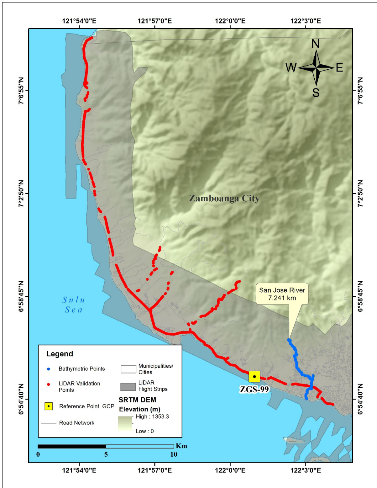
Figure 44. Validation point acquisition survey of San Jose River Basin
