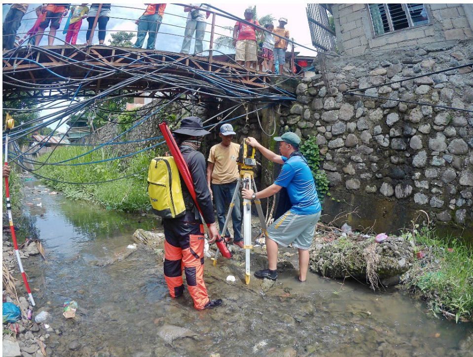
Figure 47. Bathymetric Survey using Total Station
