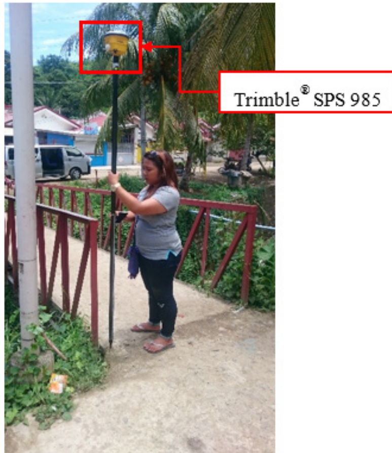
Figure 38. Bridge As-Built Survey using PPK Technique.
