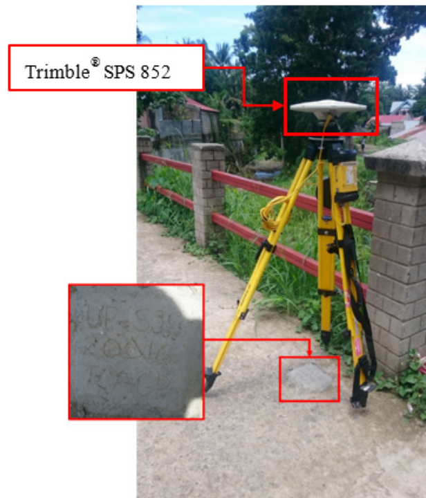
Figure 36. GNSS receiver set-up, Trimble® SPS 852, at UP-SJS located at the approach Townsville Bridge, Brgy. San Roque, Zamboanga City, Zamboanga Del Sur
