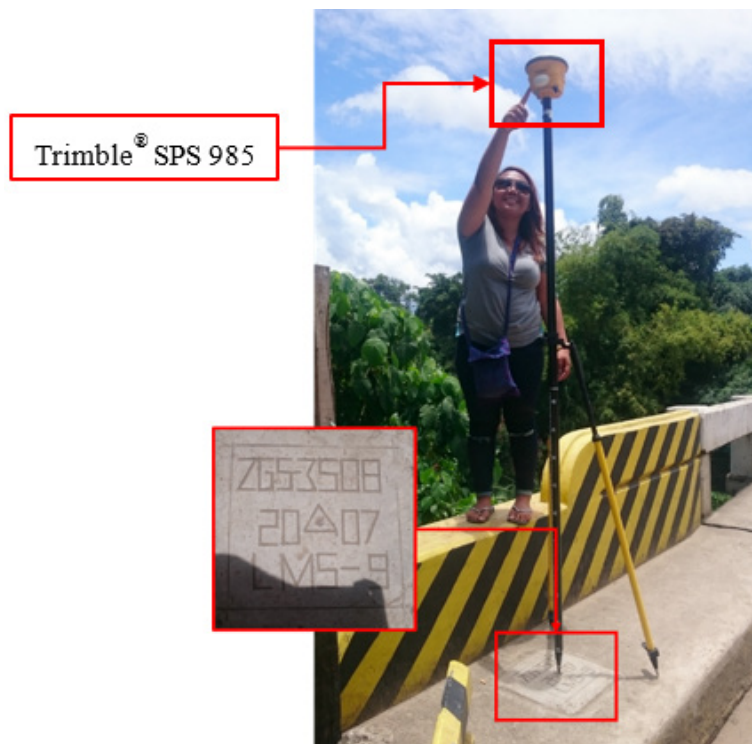
Figure 35. GNSS receiver set-up, Trimble® SPS 985, at ZGS-3508 located at the approach of Tumaga Bridge, Brgy. Tumaga, Zamboanga City, Zamboanga Del Sur
