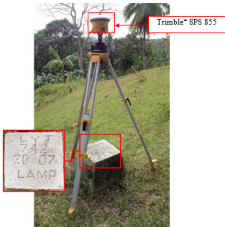
Figure 32. GNSS base set up, Trimble ® SPS 855, at LYT-742, located near a chapel and basketball court in Brgy. Tambis, Municipality of Hilongos, Leyte
