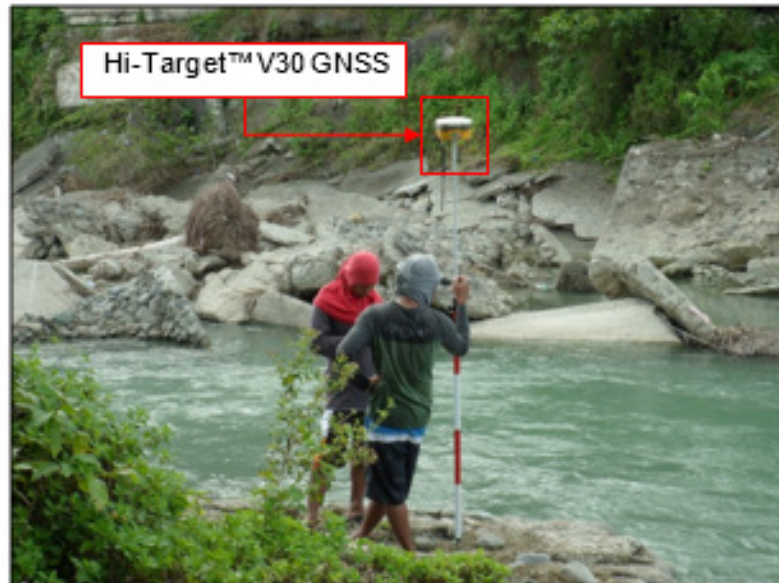
Figure 43. Manual bathymetric survey using a Hi-Target™ V30 GNSS in Salug River
