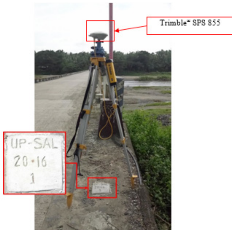
Figure 34. GNSS receiver set up, Trimble® SPS 855, at UP-SAL, located at Salug Bridge approach in Brgy. Imelda Marcos, Hilongos, Leyte
