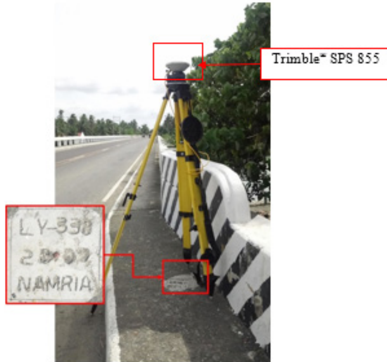
Figure 33. GNSS receiver set up, Trimble® SPS 855, at LY-338, located at the approach of Salug Birdge along Sta. Indang-Hilongos Road in Brgy. San Juan, Municipality of Hilongos, Leyte
