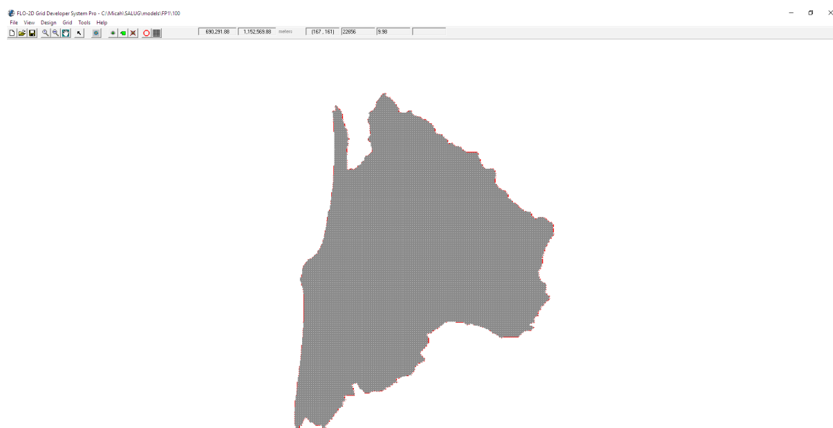
Figure 59. Screenshot of subcatchment with the computational area to be modeled in FLO-2D GDS Pro
