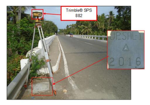
Figure 34. GNSS receiver set up, Trimble® SPS 882, UP\_SAL-1 located at the side of Ipil-Dipolog Highway near Salug Bridge in Brgy. La Libertad, Municipality of Gutalac, Province of Zamboanga del Norte
