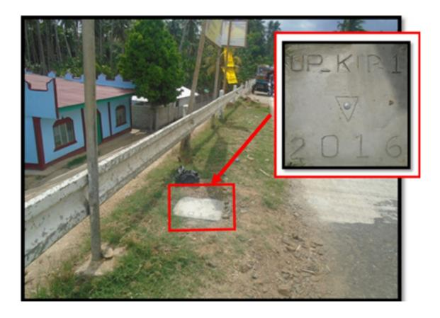
Figure 31. UP\_KIP-1 located at the approach of Kipit Bridge in Brgy. Kipit, Municipality of Labason, Province of Zamboanga del Norte
