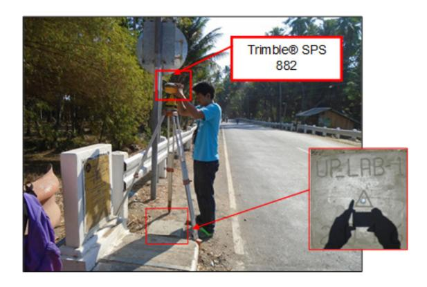
Figure 32. GNSS receiver set up, Trimble® SPS 882, at UP\_LAB-1 at Labason Bridge in Brgy. Antonio, Municipality of Labason, Province of Zamboanga del Norte
