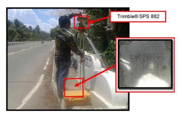
Figure 30. GNSS rover, Trimble® SPS 882, at ZN-143, an established control point, located at the right side walk going to Brgy. Rizon direction of Polandok Bridge in Brgy.Ramon Magsaysay, Salug, Province of Zamboanga del Norte
