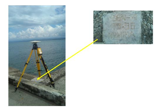
Figure 5. GPS set-up over ZGN-4 at Barangay Lamao, Liloy, Zamboanga del Norte (a) and NAMRIA reference point ZGN-4 (b) as recovered by the field team.
