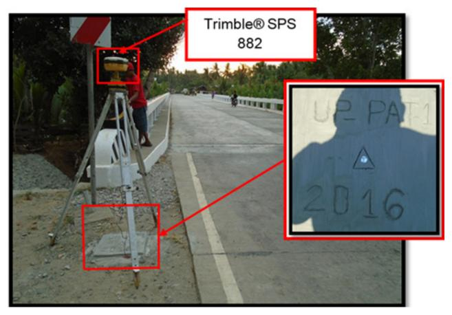
Figure 33.GNSS receiver set up, Trimble SPS 882, UP\_PAT-1 at the side of Labason-Liloy Road near Patawag Bridge in Brgy. Patawag, Municipality of Labason, Province of Zamboanga del Norte
