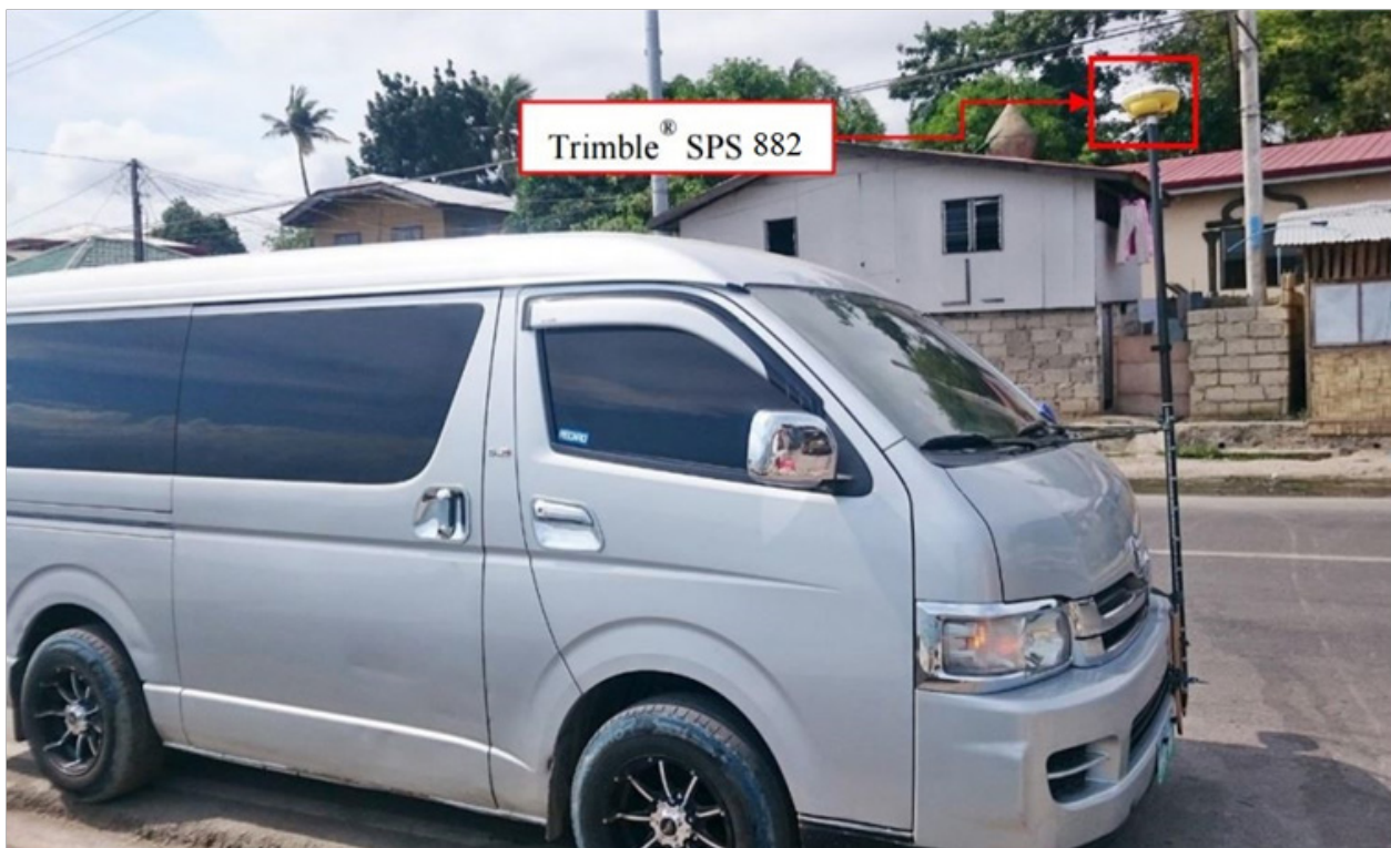
Figure 43. Validation points acquisition survey set-up for Polandok River
