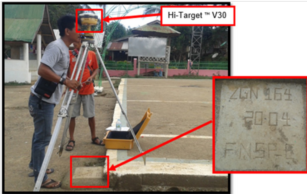
Figure 31. GNSS rover, Hi-Target™ V30, ZGN-164, situated inside the barangay hall compound beside basketball court in Brgy. Caracol, Salug, Province of Zamboanga del Norte
