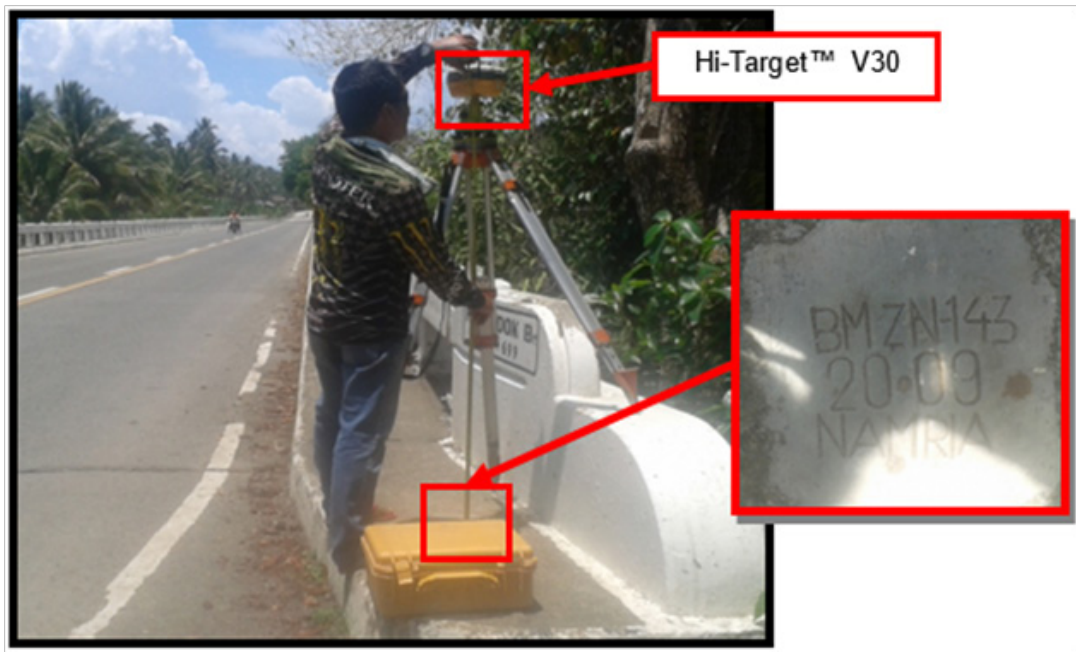
Figure 32. GNSS rover, Hi-Target™ V30, at ZN-143, an established control point, located at the right side walk going to Brgy. Rizon direction of Palandok Bridge in Brgy. Ramon Magsaysay, Salug, Province of Zamboanga del Norte
