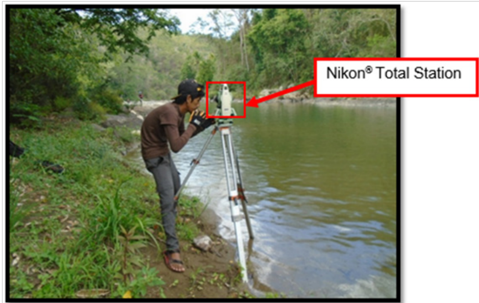
Figure 45. Manual bathymetric survey at Polandok River using Nikon® Total Station
