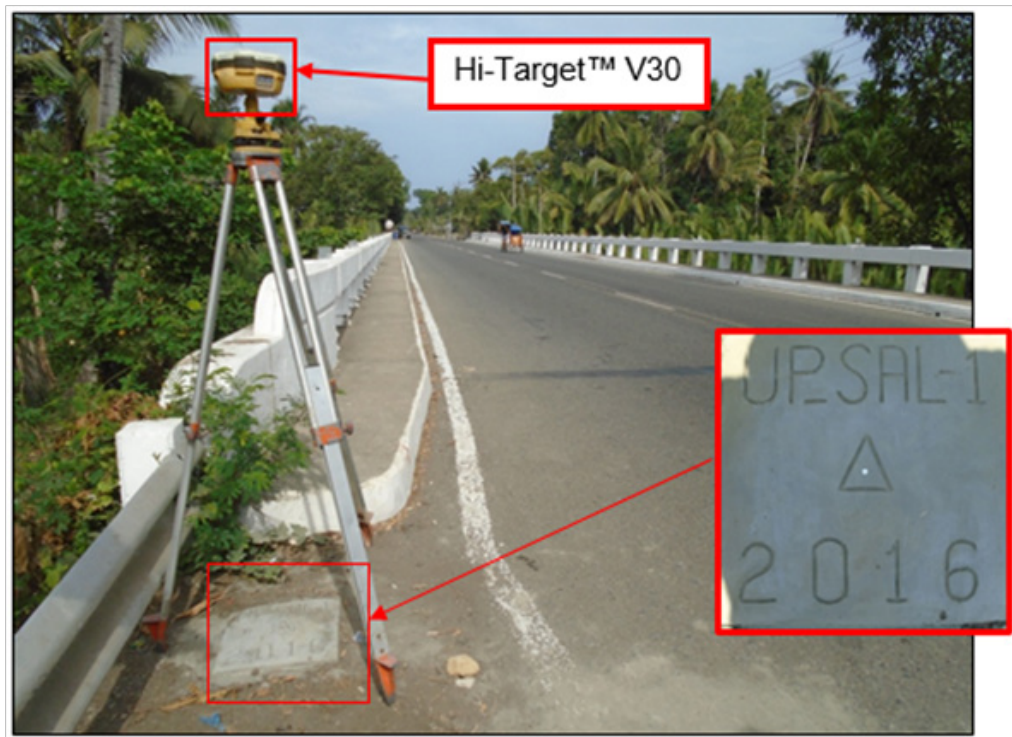
Figure 36. GNSS receiver set up, Hi-Target™ V30, UP_SAL-1 located at the side of Ipil-Dipolog Highway near Salug Bridge in Brgy. La Libertad, Municipality of Gutalac, Province of Zamboanga del Norte
