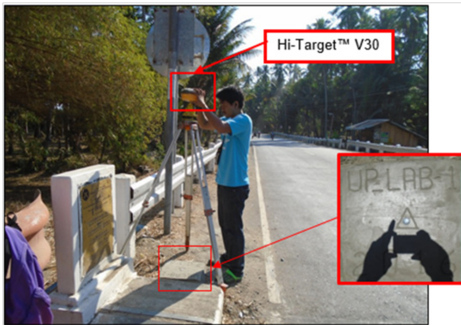
Figure 34. Figure C-6 GNSS receiver set up, Hi-Target™ V30, at UP_LAB-1 at Labason Bridge in Brgy. Antonio, Municipality of Labason, Province of Zamboanga del Norte
