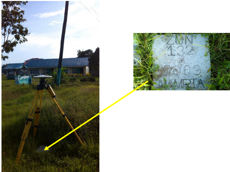
Figure 5. GPS set-up over ZGN-132 at Barangay Mandih, Zambonaga del Norte (a) and NAMRIA reference point ZGN-132 (b) as recovered by the field team.
