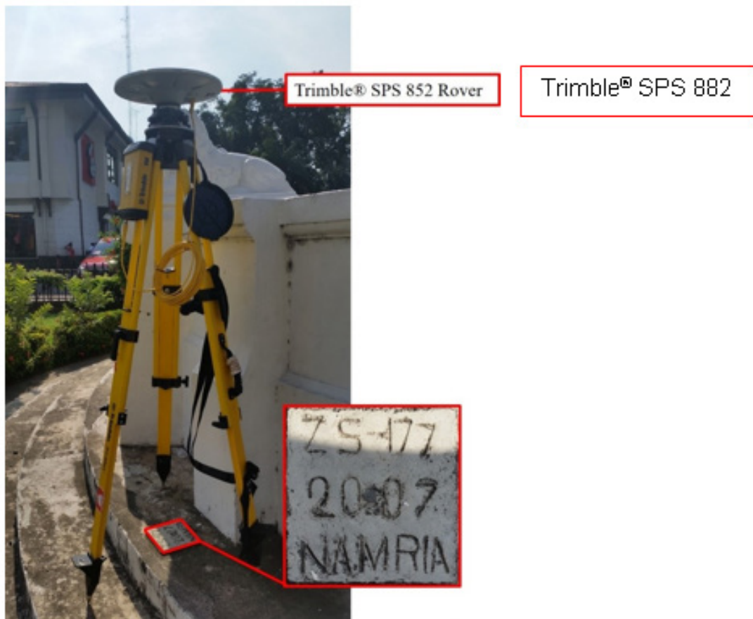
Figure 34. GNSS base set up, Trimble® SPS 882, at ZS-177, located in Brgy. Poblacion, Zamboanga City, Province of Zamboanga del Sur.
