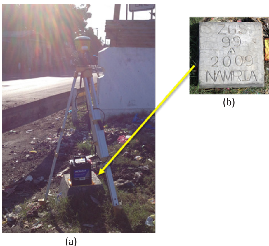
Figure 5. GPS set-up over ZGS-99 beside the seawall in Calarian, Zamboanga City (a) and NAMRIA reference point ZGS-99 (b) as recovered by the field team.
