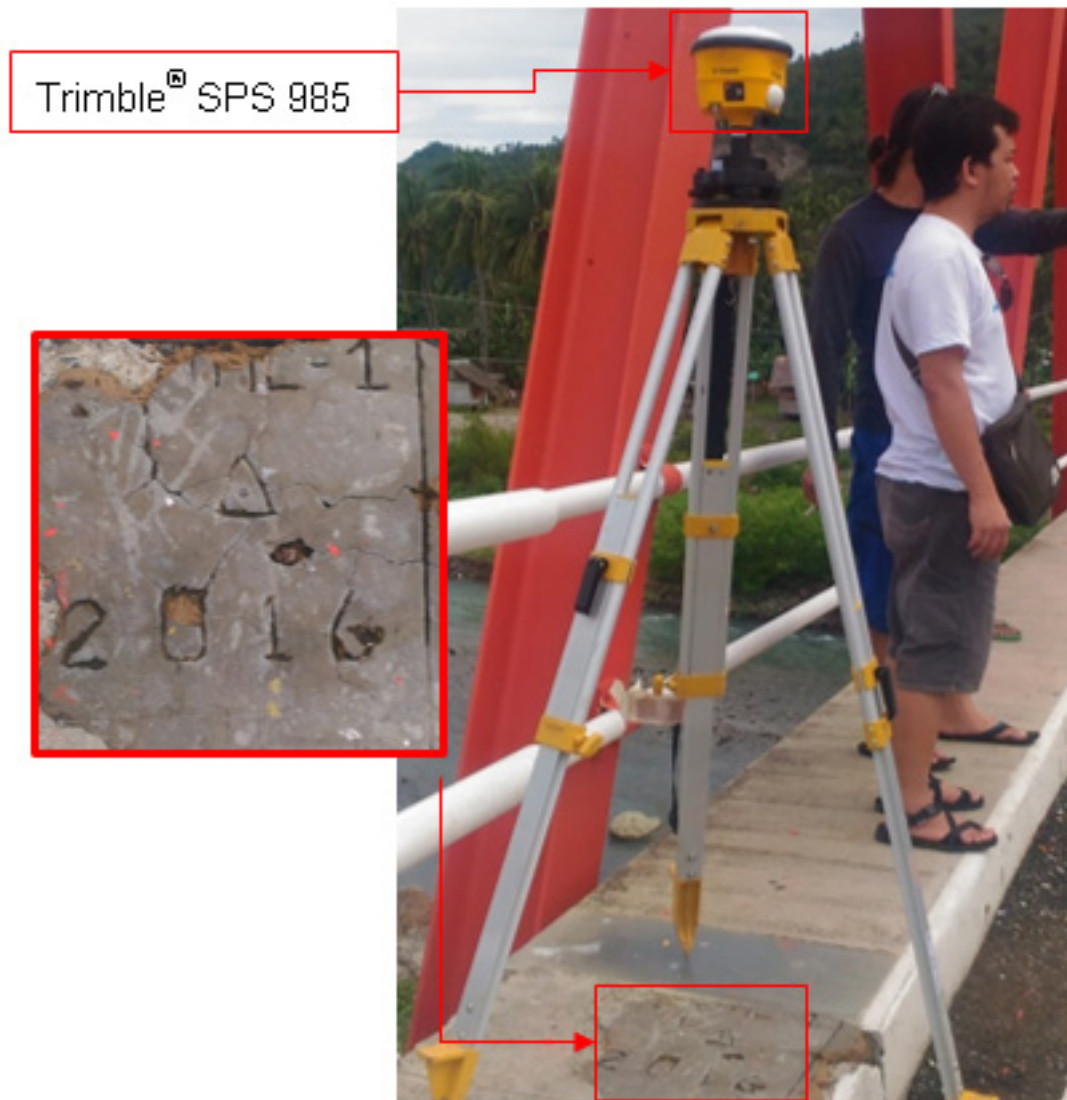
Figure 35. GNSS receiver set up, Trimble® SPS 985, at UP_mal-1, located at the approach of Limpapa Bridge foot walk in Brgy. Limpapa, Sibuco, Province of Zamboanga Del Norte.
