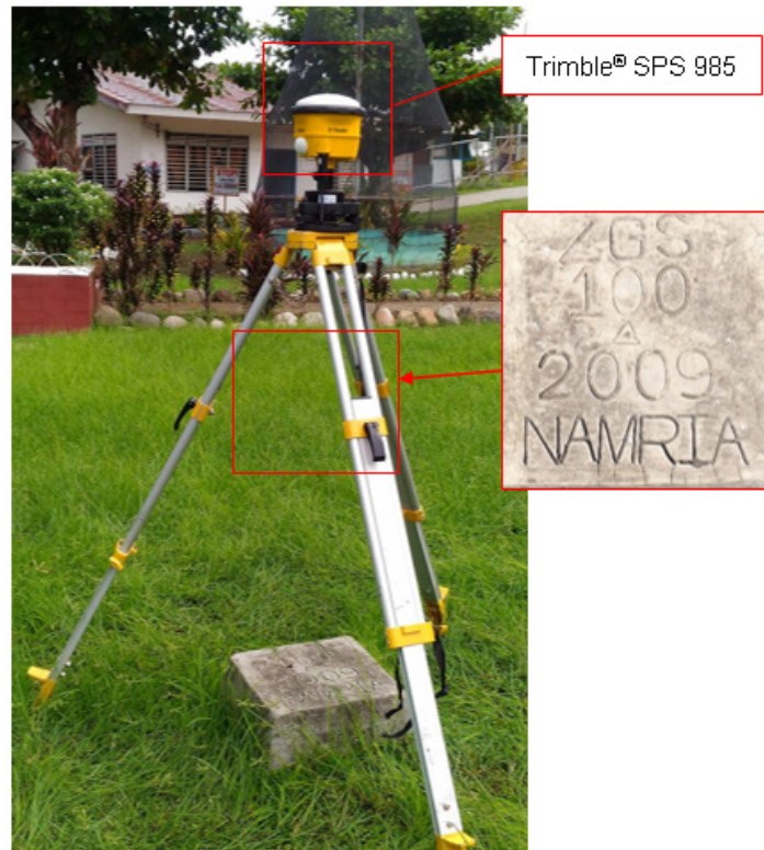
Figure 33. GNSS receiver set up, Trimble® SPS 985, at ZGS-100, located at Brgy. Manicahan, Zamboanga City, Province of Zamboanga del Sur.
