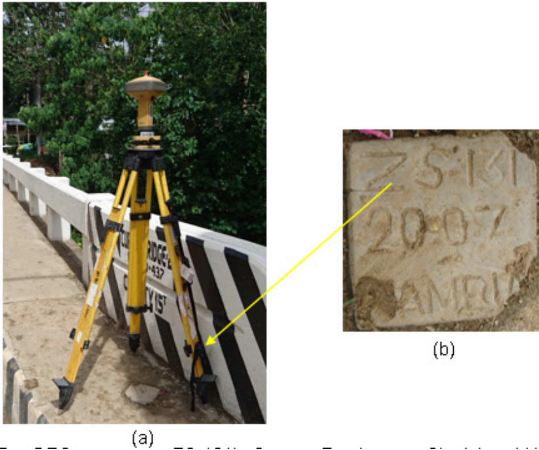
Figure 7. GPS set-up over ZS-131 in Curuan, Zamboanga City (a) and NAMRIA reference point ZS-131 (b) as recovered by the field team.
