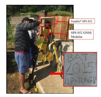
Figure 31. GNSS receiver, Trimble<sup>®</sup> SPS 852 setup at control point BAT, at Batu Bridge in Brgy. Batu, Municipality of Siay, Zamboanga Sibugay along the PAN-Philippine National Highway
