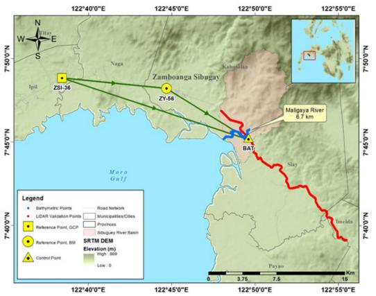
*Figure 27. Extent of the bathymetric survey (in blue line) in Batu River and the LiDAR data validation survey (in red).*
