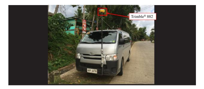
Figure 37. Trimble<sup>®</sup> SPS882 set-up for validation points acquisition survey for Maligaya River
