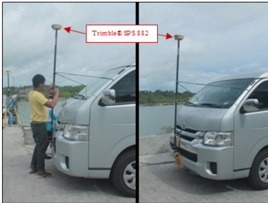
Figure 45. Validation points acquisition survey setup.
