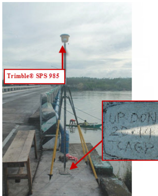
Figure 38. Trimble® SPS 985 setup at UP-DON, Dankalan Bridge, Brgy. Dankalan, Donsol, Sorsogon
