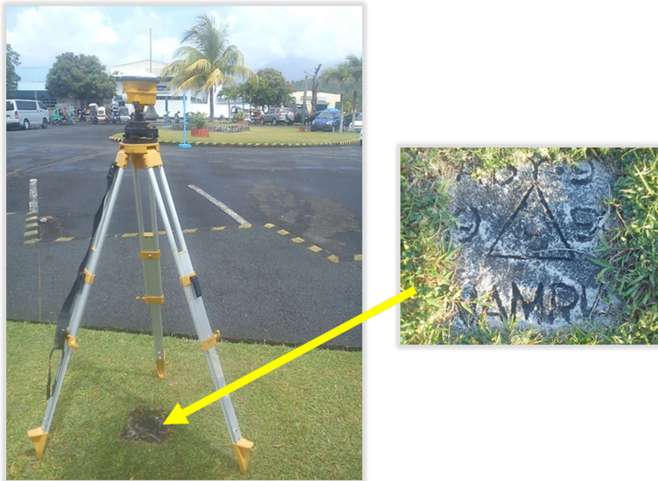
Figure 7. GPS set-up over ABY-9 inside Legaspi Airport Compound 52.0 meters SE of Legaspi Airport Flagpole, 35 meters NE of Legaspi Airport Welcome Post 3.30 meters NW of Lamp (a) and NAMRIA reference point ABY-9 (b) as recovered by the field team.
