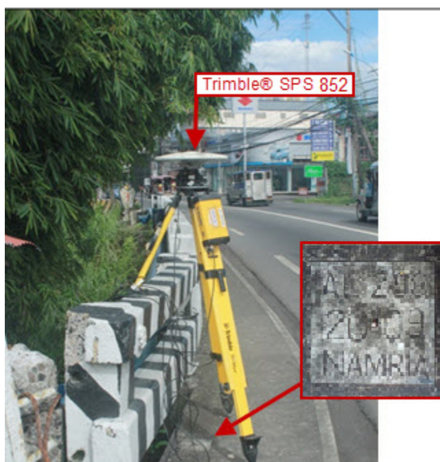
Figure 36. Trimble® SPS 852 setup at AL-298, Sagpon Bridge Brgy. Sagpon, Legazpi City, Albay
