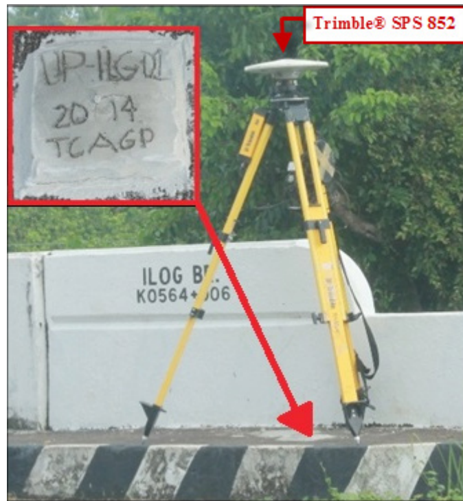
Figure 39. Trimble® SPS 852 setup at UP-ILG01 at the approach of Ilog Bridge, Brgy. Gura, Donsol, Sorsogon
