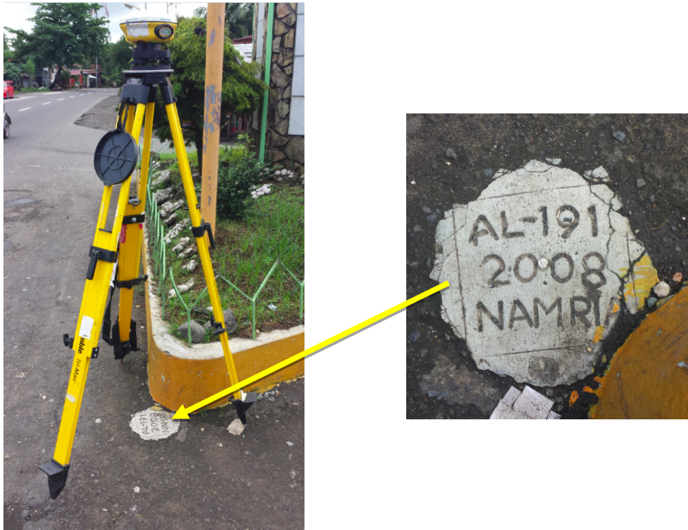
Figure 9. GPS set-up over AL-191 along the Albay-Sorsogon National road at the edge of the center island at about 5 meters south of the centerline of the road (a) and NAMRIA benchmark AL-191 (b) as recovered by the field team.
