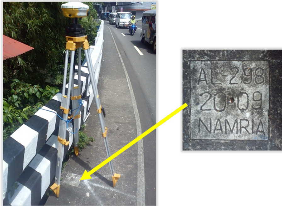
Figure 8. GPS set-up over AL-289 at the south west end of Sagpon Bridge at KM 528+166 and about 4.8 meters SW of the centerline of the road, along the Legazpi-Daraga national road (a) and NAMRIA benchmark AL-289 (b) as recovered by the field team.
