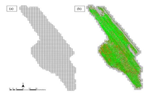
Figure 16. Tiles for Nauco Aguada floodplain (a) and classification results (b) in TerraScan.
