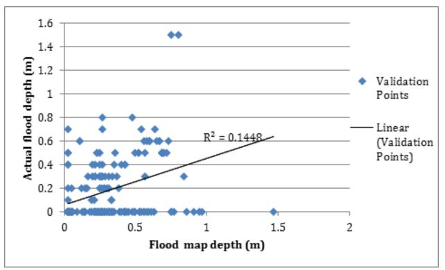
Figure 87. Flood map depth versus actual flood depth.
