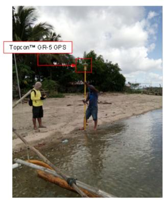
Figure 37. Cross-section survey at the mouth of Nauco Aguada River.
