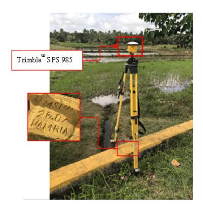
Figure 33. GNSS receiver setup, Trimble® SPS 985, at MS-141, located in Brgy. San Vicente, Municipality of Cawayan, Masbate.
