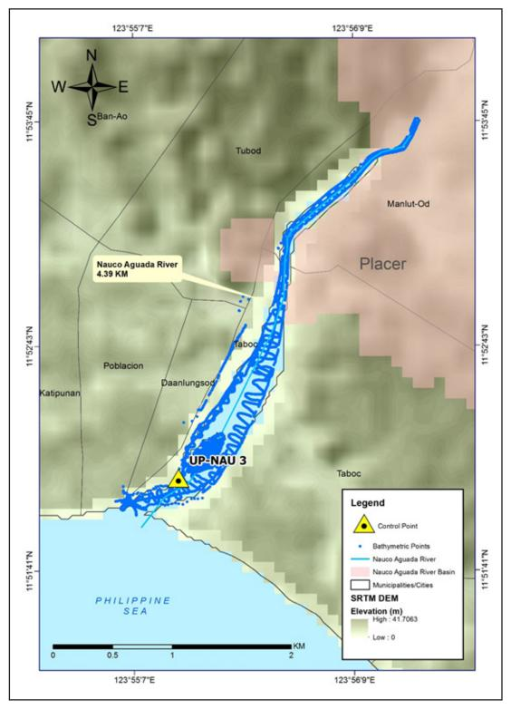
Figure 47. The extent of the Nauco Aguada River Bathymetry Survey.
