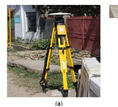
Figure 3. GPS set-up over MST-40 (a) as recovered in Buenavista Bridge in Brgy. Buenavista, municipality of Uson, Masbate; and NAMRIA reference point MST-40 (b) as recovered by the field team.
