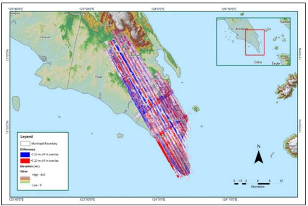
Figure A-8.7. Elevation difference between flight lines
