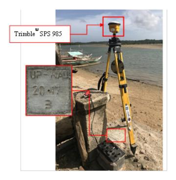
Figure 36. GNSS receiver setup, Trimble® SPS 985, at UP-NAU3, located in Brgy. Taboc, Municipality of Placer, Masbate.
