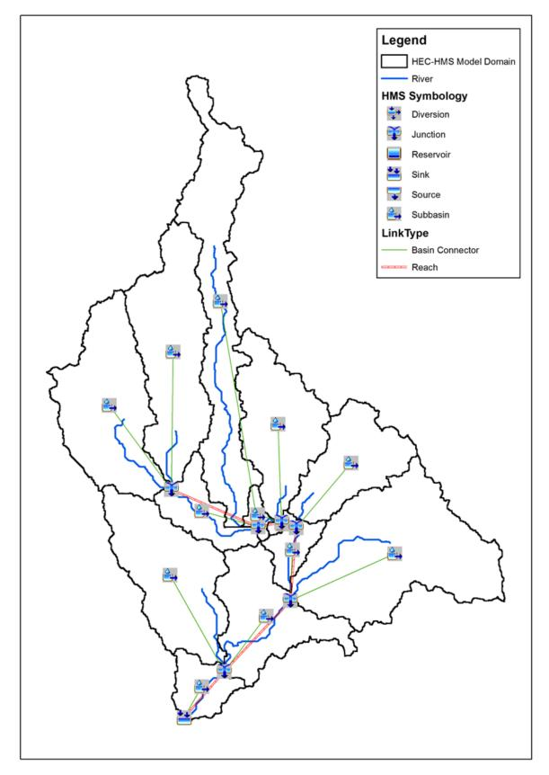
Figure 59. The Nauco Aguada river basin model generated using HEC-HMS.
