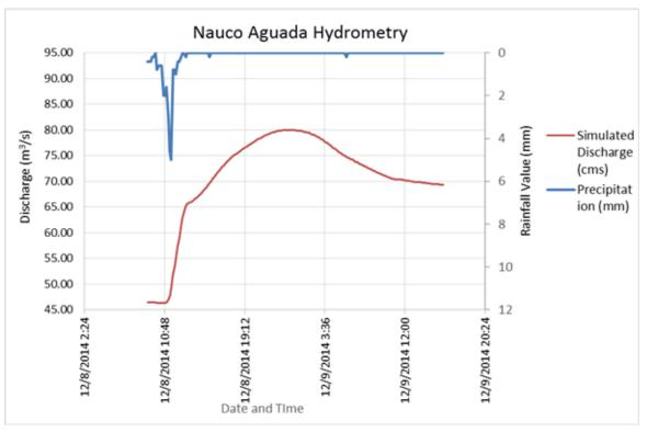
Figure 52. Rainfall and outflow data at the Nauco Aguada Bridge of the Nauco Aguada River Basin, which was used for modeling.
