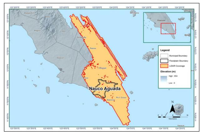
Figure 11. Boundaries of the processed LiDAR data over the Nauco Aguada Floodplain.
