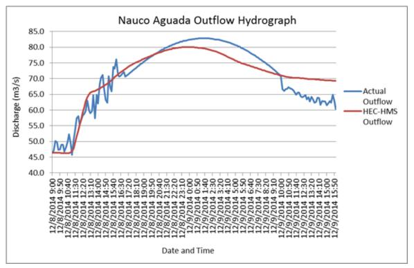
Figure 62. Outflow Hydrograph of Nauco Aguada produced by the HEC-HMS model compared with observed outflow.
