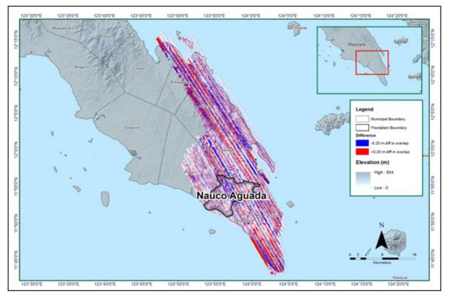
Figure 14. Elevation difference Map between flight lines for the Nauco Aguada Floodplain Survey.
