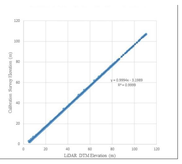
Figure 24. Correlation plot between calibration survey points and LiDAR data.
