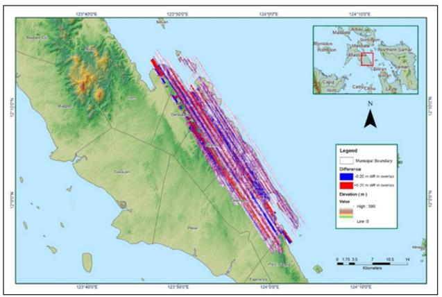
Figure A-8.21. Elevation difference between flight lines
