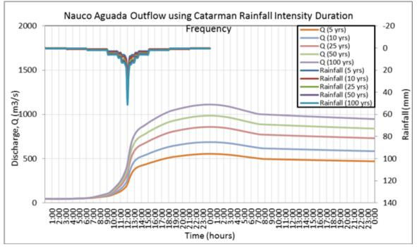
Figure 63. The Outflow hydrograph at the Nauco Aguada Station, generated using the Romblon RIDF simulated in HEC-HMS.
