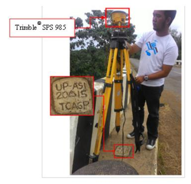
Figure 32. GNSS receiver setup, Trimble® SPS 985, at UP-ASI, located Brgy. Cayabon, Municipality of Milagros, Masbate.
