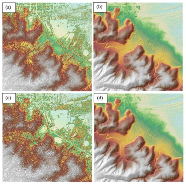
Figure 18. The production of last return DSM (a) and DTM (b), first return DSM (c) and secondary DTM (d) in some portion of Nauco Aguada floodplain.
