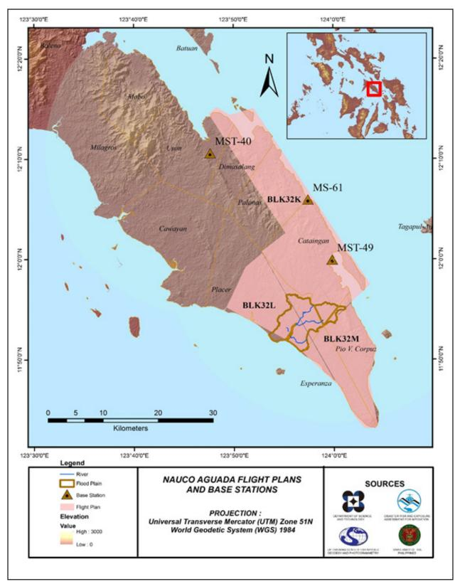
Figure 2. Flight Plan and base stations used for the Nauco Aguada Floodplain survey using Pegasus sensor.
