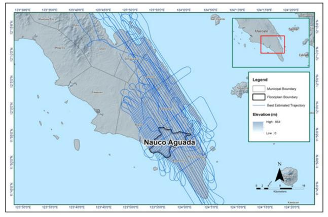
Figure 10. Best Estimated Trajectory of the LiDAR missions conducted over the Nauco Aguada Floodplain.
