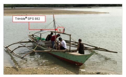
Figure 45. Gathering of random bathymetric points along Nauco Aguada River conducted by the DVBC.
