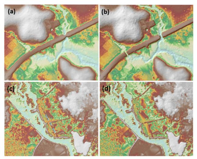
Figure 21. Portions in the DTM of the Nauco Aguada Floodplain – a bridge before (a) and after (b) manual editing; a paddy filed before (c) and after (d) data retrieval.
