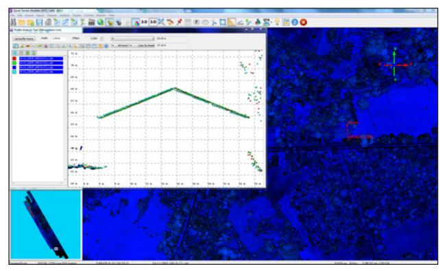
Figure 15. Quality checking for Nauco Aguada flight 1291P using the Profile Tool of QT Modeler.
