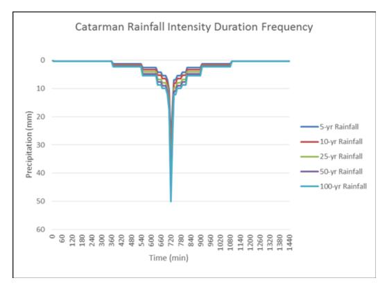
Figure 54. The synthetic storm generated for a 24-hour period rainfall for various return periods.
