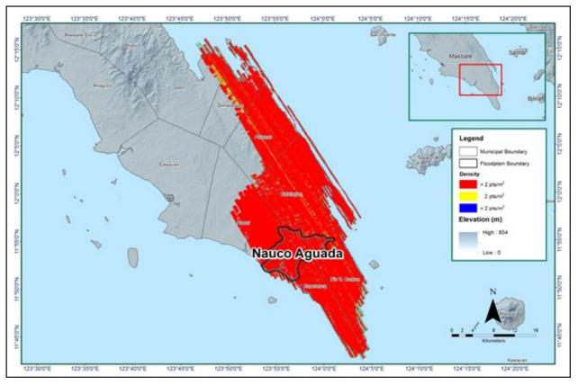
Figure 13. Pulse density map of the merged LiDAR data for Nauco Aguada floodplain.
