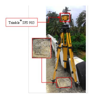
Figure 34. GNSS receiver setup, Trimble® SPS 985, at MST-41, located in Brgy. Gaid, Municipality of Dimasalang, Masbate.
