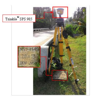
Figure 31. GNSS base set up, Trimble® SPS 985, at MST-4549, located in Brgy. Canjunday, Municipality of Baleno, Masbate.
