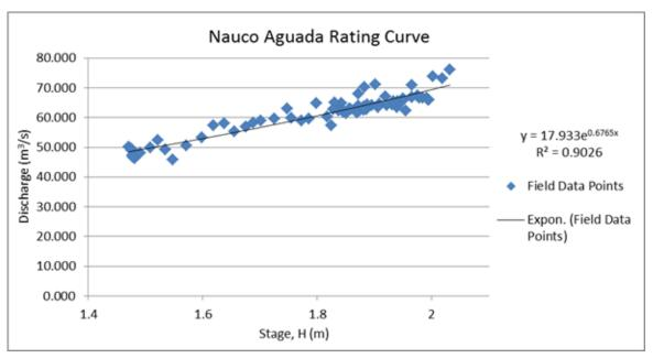
Figure 51. The rating curve of Nauco Aguada Bridge in Nauco Aguada, Masbate.
