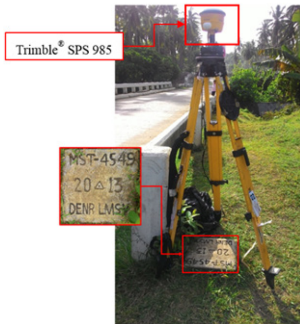
Figure 35. GNSS base set up, Trimble® SPS 985, at MST-4549, located in Brgy. Canjunday, Municipality of Baleno, Masbate.
