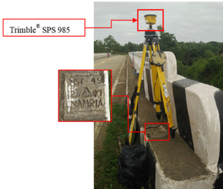
Figure 37. GNSS receiver setup, Trimble® SPS 985, at MST-45, located in Brgy. Villahermosa, Municipality of Cawayan, Masbate
