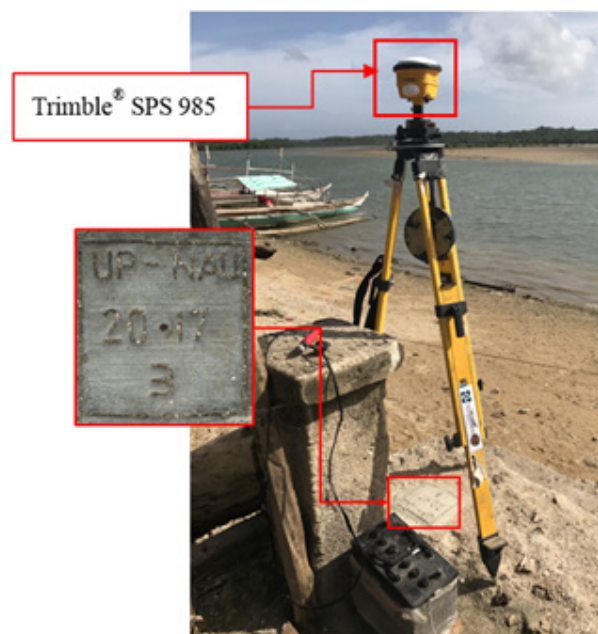
Figure 40. GNSS receiver setup, Trimble® SPS 985, at UP-NAU3, located in Brgy. Taboc, Municipality of Placer, Masbate
