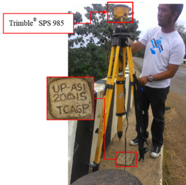
Figure 39. GNSS receiver setup, Trimble® SPS 985, at UP-ASI, located Brgy. Cayabon, Municipality of Milagros, Masbate
