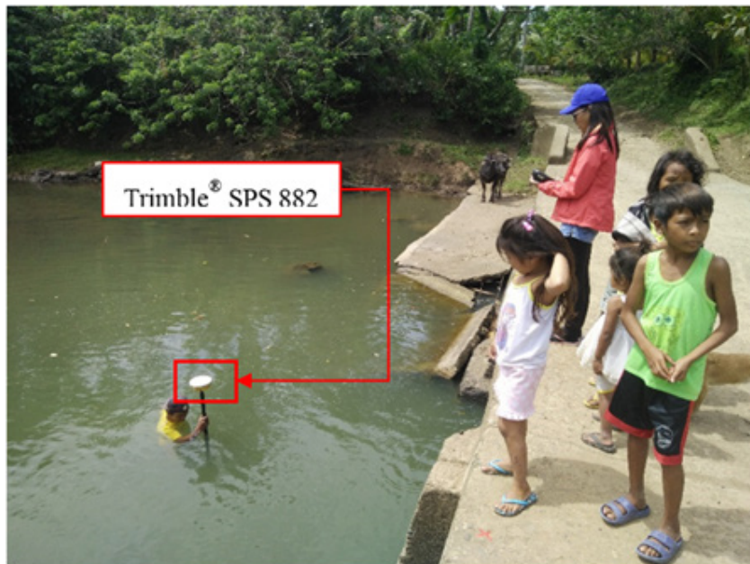
Figure 42. Bridge As-Built Survey using PPK Technique
