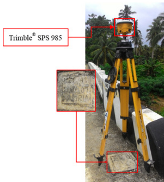
Figure 36. GNSS receiver setup, Trimble® SPS 985, at MST-41, located in Brgy. Gaid, Municipality of Dimasalang, Masbate
