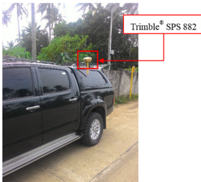
Figure 47. Validation points acquisition survey set up along Malbug River Basin
