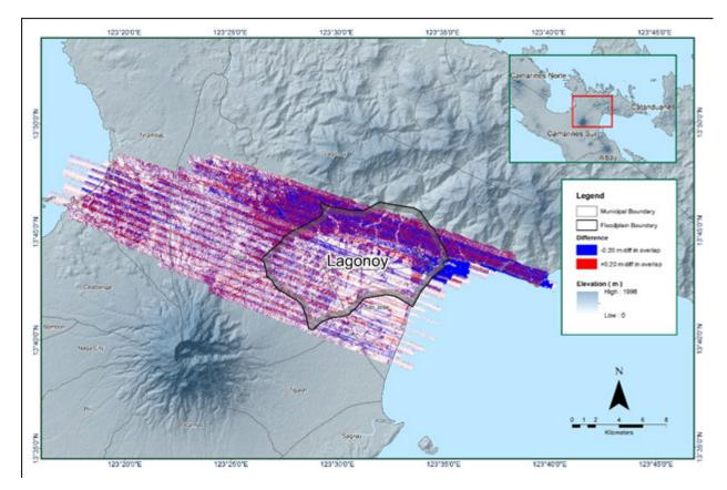
Figure 14. Elevation difference map between flight lines for Lagonoy Floodplain.
