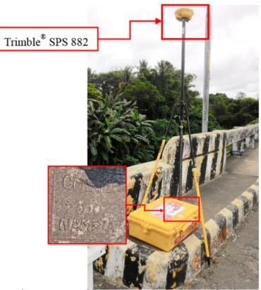
Figure 29. GNSS base set up, Trimble® SPS 882, at CMS-110, situated at the approach of Culasi Bridge in Brgy. Taytay, Municipality of Goa, Camarines Sur
