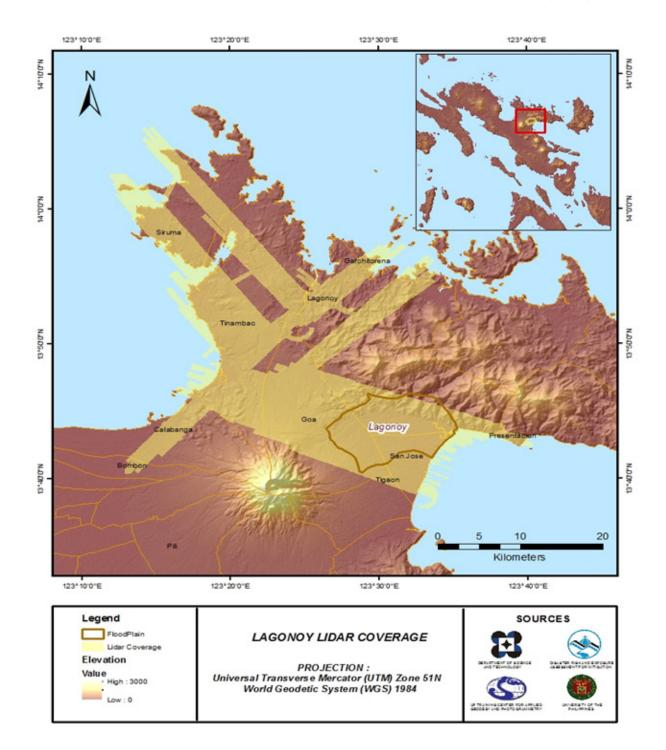
Figure 6. Actual LiDAR survey coverage for Lagonoy Floodplain
