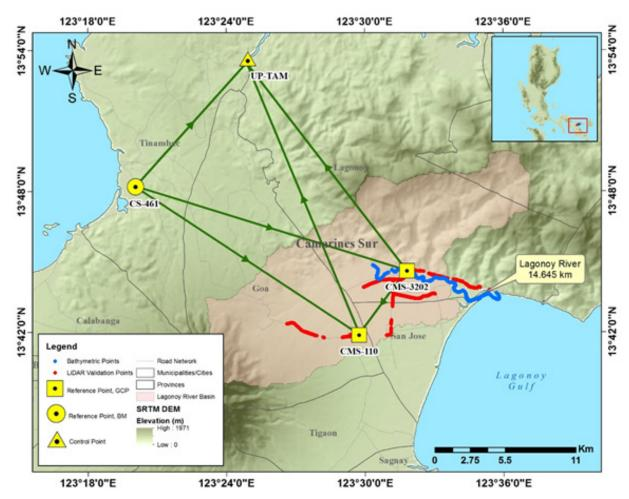
Figure 27. Extent of the bathymetric survey (in blue line) in Lagonoy River and the LiDAR data validation survey (red)
