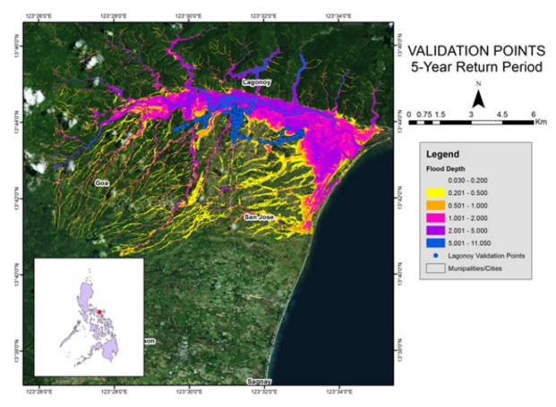
Figure 93. Flood validation points for Lagonoy Floodplain
