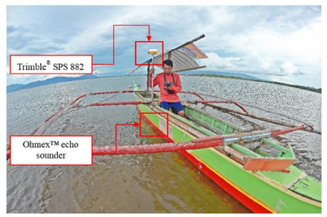
Figure 40. Bathymetric survey using Ohmex™ single beam echo sounder in Lagonoy River
