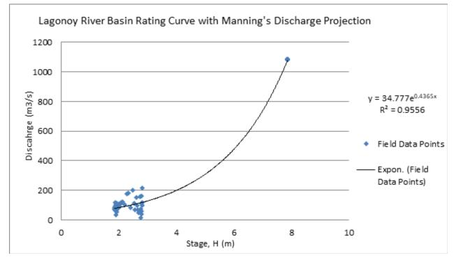
Figure 46. The rating curve of Lagonoy Bridge in Lagonoy, Camarines Sur
