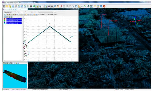
Figure 15. Quality checking for Lagonoy Flight 23290P using the Profile Tool of QT Modeler.
