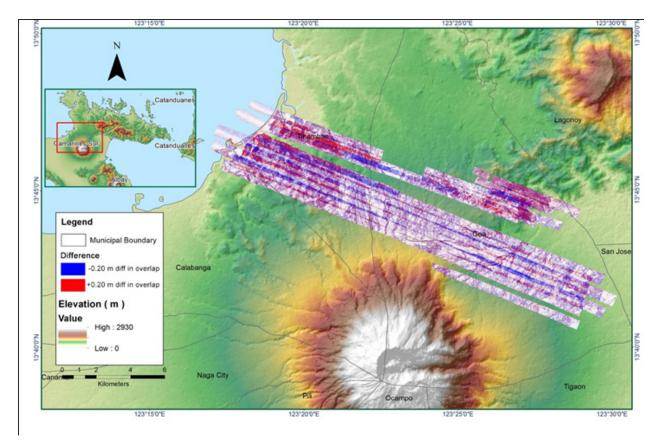
Figure A-8.21. Elevation difference between flight lines
