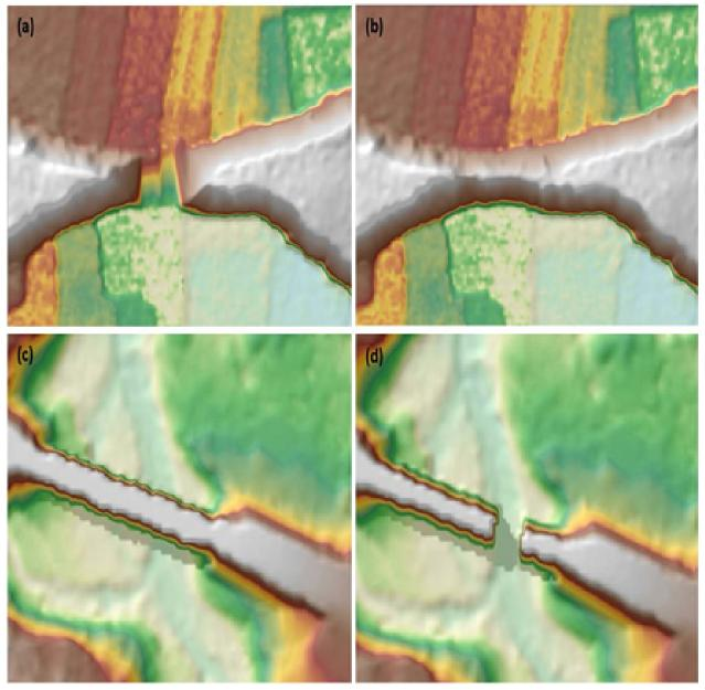
Figure 19. Portions in the DTM of Lagonoy Floodplain – a paddy field before (a) and after (b) data retrieval; and a bridge before (c) and after (d) manual editing.
