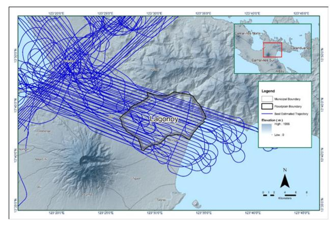
Figure 10. Best Estimated Trajectory of the LiDAR missions conducted over the Lagonoy Floodplain.
