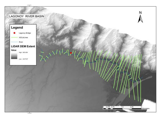
Figure 55. River cross-section of Lagonoy River generated through Arcmap HEC GeoRAS tool
