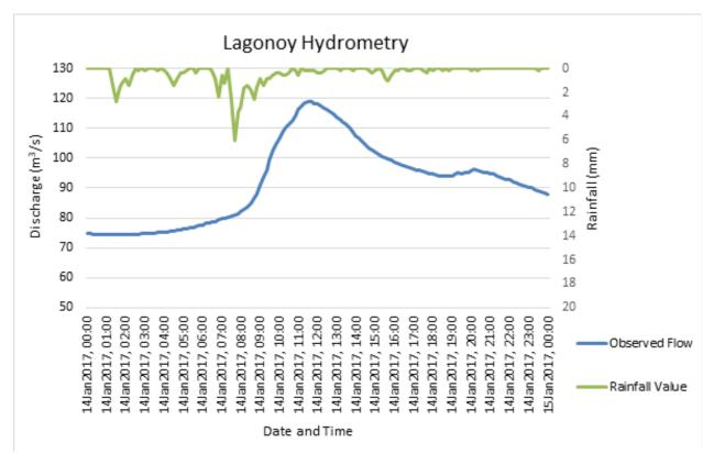
Figure 47. Rainfall and outflow data of the Lagonoy River Basin, which was used for modeling
