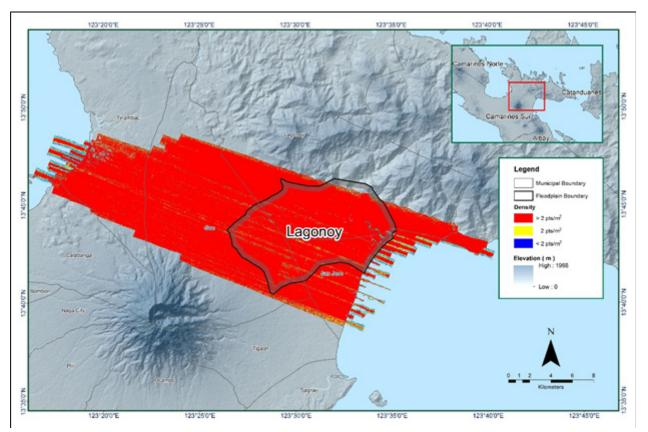
Figure 13. Pulse density map of merged LiDAR data for Lagonoy Floodplain.
