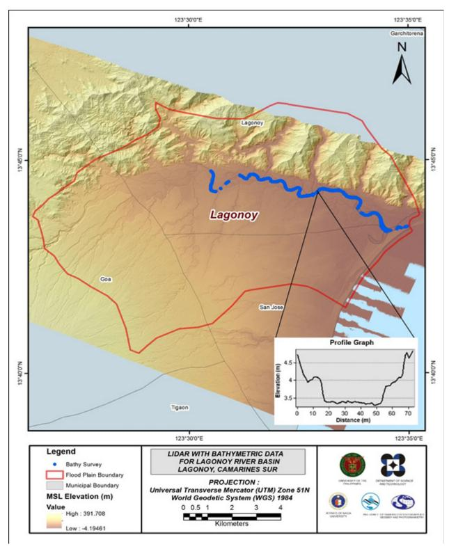
Figure 24. Map of Lagonoy Floodplain with bathymetric survey points shown in blue.
