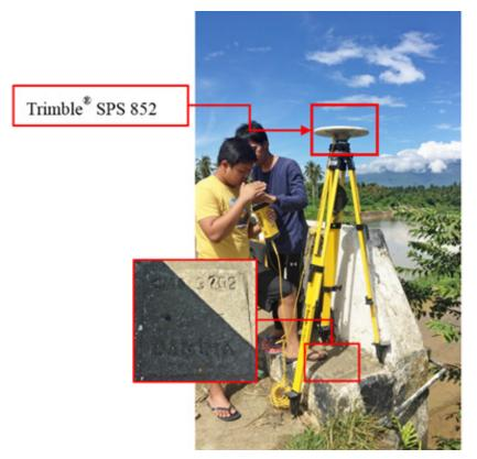
Figure 31. GNSS receiver setup, Trimble® SPS 852, at CMS-3202, located at the approach of Lagonoy Bridge in Brgy. Ginorangan, Municipality of Lagonoy, Camarines Sur
