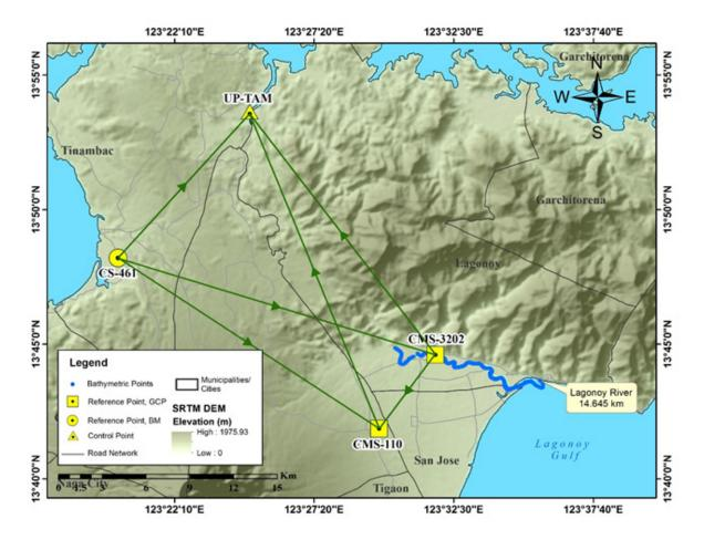
Figure 28. GNSS Network of Lagonoy River Basin Survey
