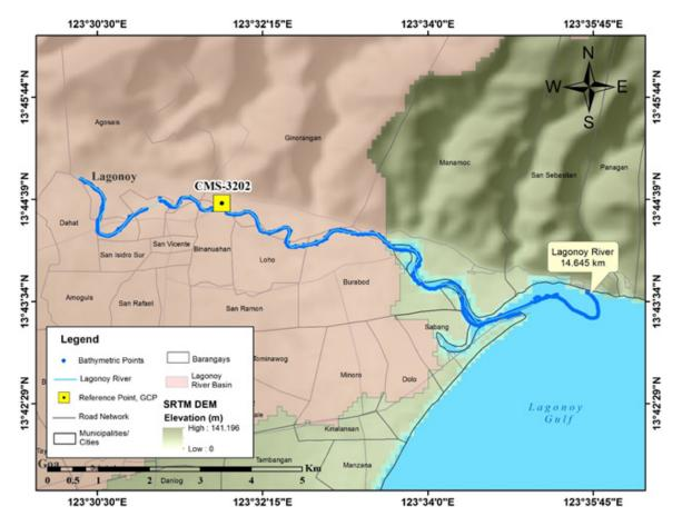
Figure 42. Bathymetric Survey of Lagonoy River
