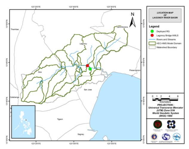
Figure 44. The location map of Lagonoy HEC-HMS model used for calibration
