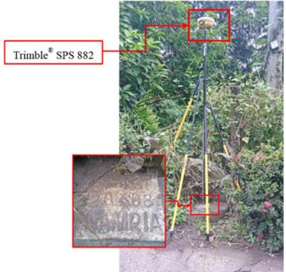
Figure 30. GNSS receiver setup, Trimble® SPS 882, at CS-461, located at the approach of a bridge in Brgy. Balaobalite, Municipality of Tinambac, Camarines Sur
