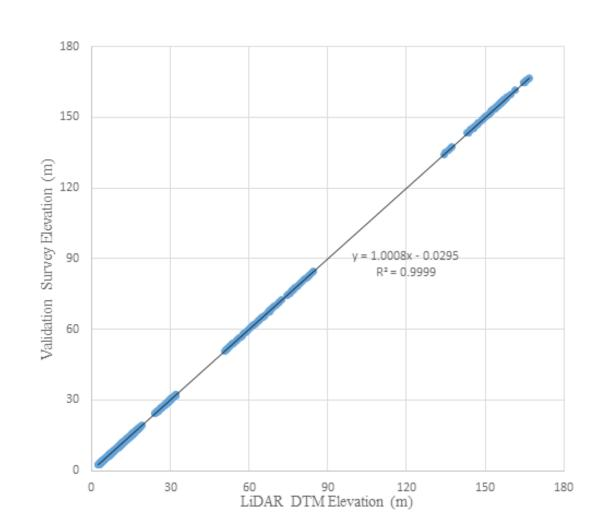
Figure 23. Correlation plot between validation survey points and LiDAR data.
