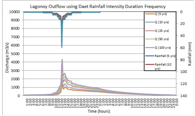
Figure 58. The Outflow hydrograph at the Lagonoy Basin, generated using the simulated rain events for 24-hour period for Daet station
