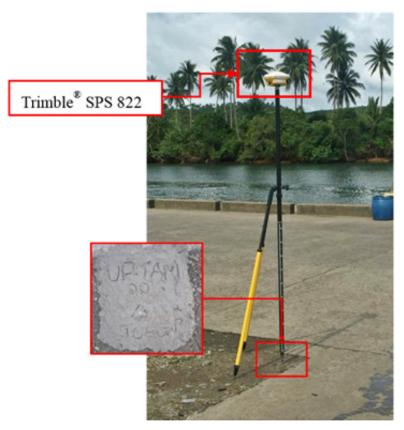
Figure 32. GNSS receiver setup, Trimble® SPS 822, at UP-TAM, located at Tamban Port, Brgy. Tamban, Municipality of Tinambac, Camarines Sur
