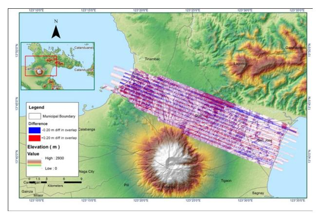
Figure A-8.7. Elevation difference between flight lines
