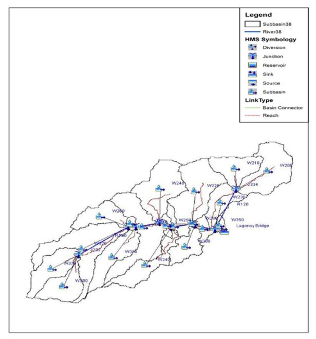
Figure 54. The Lagonoy River Basin model generated using HEC-HMS
