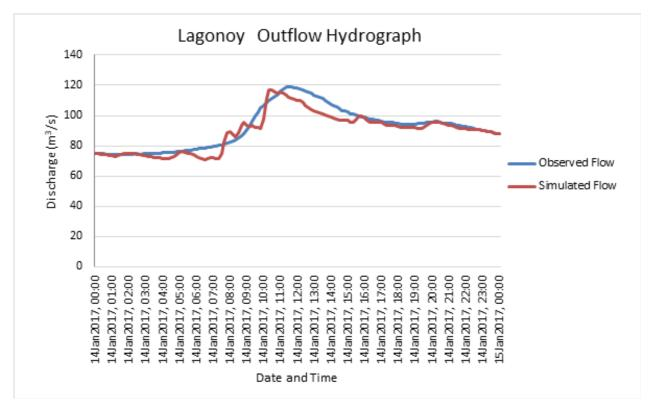
Figure 57. Outflow hydrograph of Lagonoy River Basin produced by the HEC-HMS model compared with observed outflow
