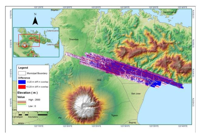
Figure A-8.28 Elevation difference between flight lines
