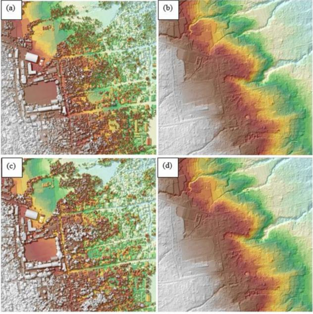
Figure 18. The Production of last return DSM (a) and DTM (b), first return DSM (c) and secondary DTM (d) in some portion of Lagonoy Floodplain.
