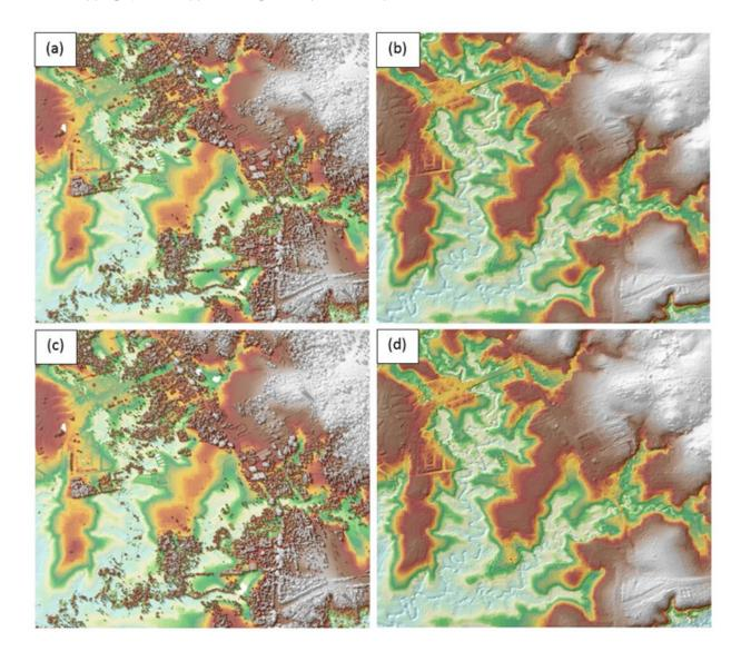
Figure 21. The Production of last return DSM (a) and DTM (b), first return DSM (c), and secondary DTM (d) in some portion of Daraga Floodplain.
