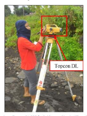
Figure 38. Leveling using a Topcon DL 500 for bridge marking in Kilicao Bridge, Daraga, Albay
