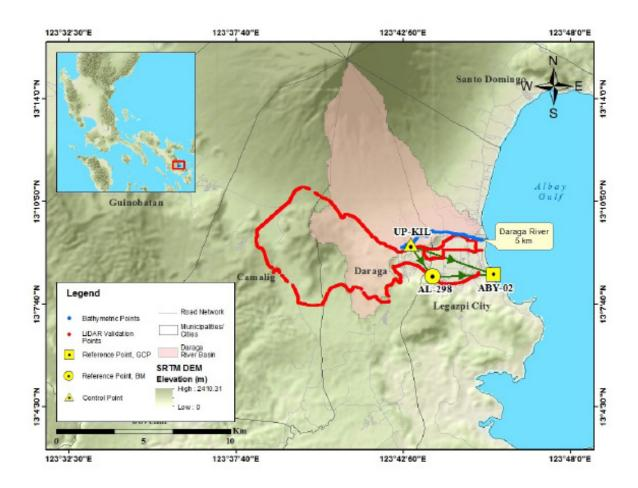
Figure 32. Extent of the bathymetric survey (in blue line) in Daraga River and the LiDAR data validation survey (red).
