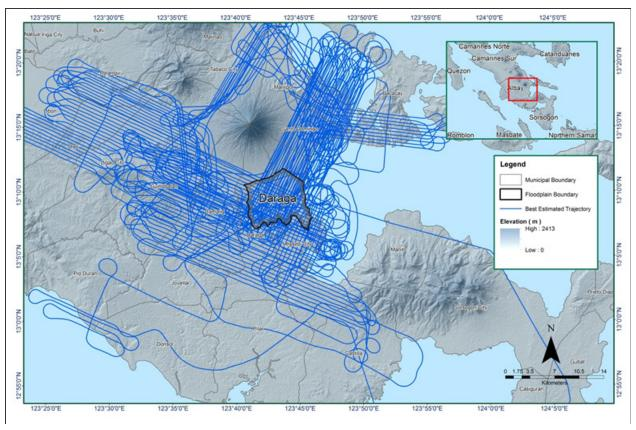
Figure 13. Best Estimated Trajectory of the LiDAR missions conducted over the Daraga Floodplain.
