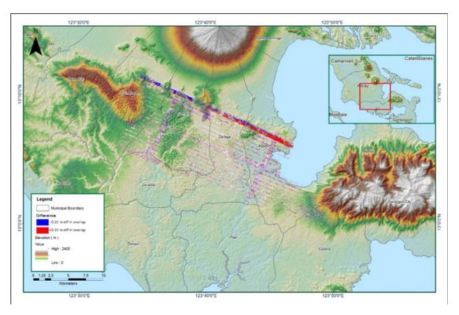
Figure A-8.7. Elevation difference between flight lines
