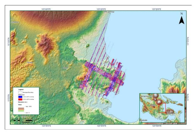
Figure A-8.28. Elevation difference between flight lines
