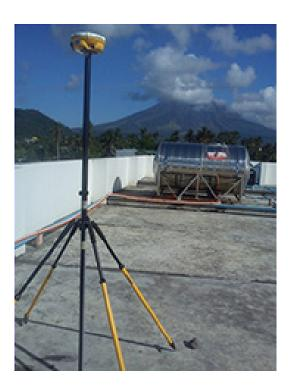
Figure 7. GPS set-up over LPH-01 located at the rooftop of La Piazza Hotel and Convention Center along Tahao Road, Legazpi, Albay.
