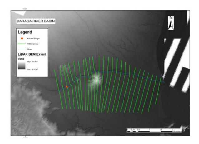
Figure 58. River cross-section of Daraga River generated through Arcmap HEC GeoRAS tool
