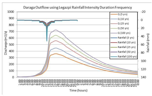
Figure 61. The Outflow hydrograph at the Daraga Station, generated using the simulated rain events for 24-hour period for Legazpi station
