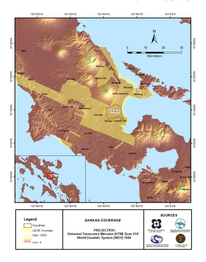
Figure 9. Actual LiDAR survey coverage for Daraga Floodplain.
