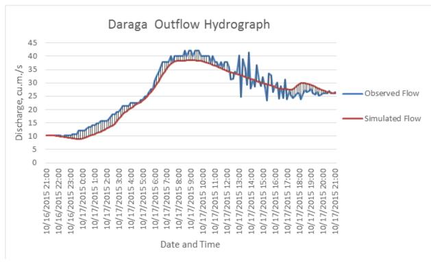
Figure 60. Outflow hydrograph of Daraga produced by the HEC-HMS model compared with observed outflow
