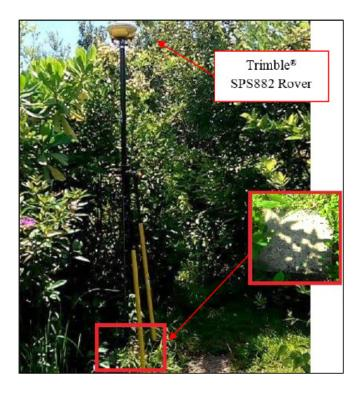
Figure 34. GNSS receiver, Trimble® SPS882 set-up at ABY-2 in Victory Village, Legazpi City, Albay
