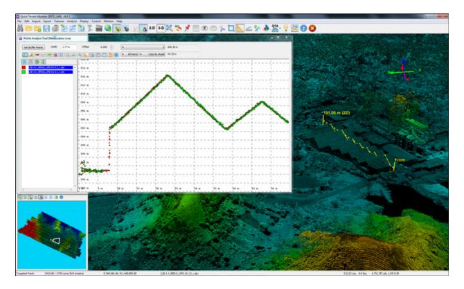
Figure 18. Quality checking for Daraga Flight 3891G using the Profile Tool of QT Modeler.
