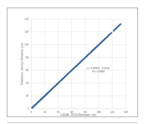
Figure 28. Correlation plot between validation survey points and LiDAR data.
