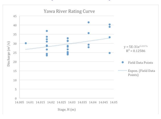
Figure 49. The rating curve of Kilicao Bridge in Daraga, Albay
