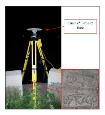
Figure 36. GNSS base, Trimble® SPS852 base set-up at UP-KIL in Kilicao Bridge in Daraga, Albay
