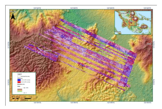
Figure A-8.42. Elevation difference between flight lines
