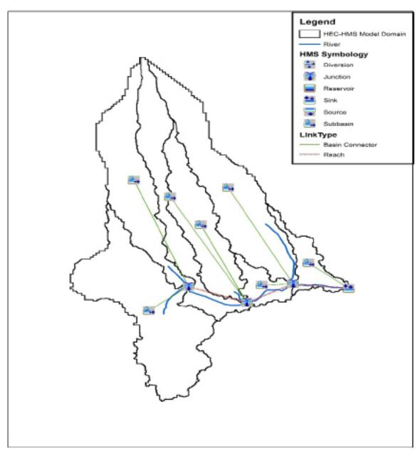
Figure 57. The Daraga River Basin model generated in HEC-HMS
