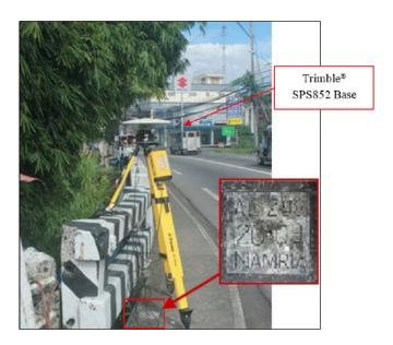
Figure 35. GNSS base receiver Trimble® SPS852 at AL-298 in Sagpon Bridge, Legazpi City, Albay
