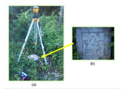
Figure 3. a) GPS set-up over ABY-92 beside the baseline of the basketball court at about 19 m from the barangay hall, and b) NAMRIA reference point ABY-92 as recovered by the field team.
