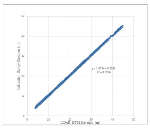
Figure 27. Correlation plot between calibration survey points and LiDAR data.
