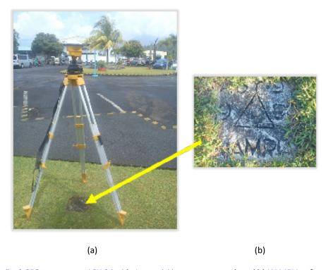
Figure 5. a) GPS set-up over ABY-9 inside Legaspi Airport compound, and b) NAMRIA reference point ABY-9 as recovered by the field team.
