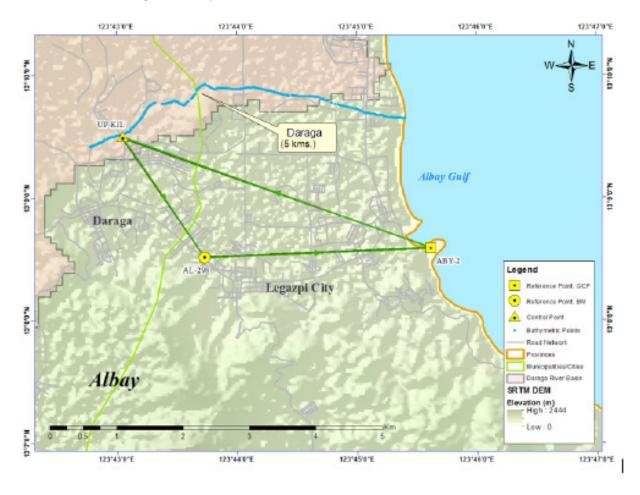
Figure 33. GNSS Network of Daraga River Basin Survey
