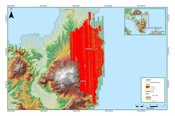
Figure 1.11.6. Density map of merged LiDAR data
