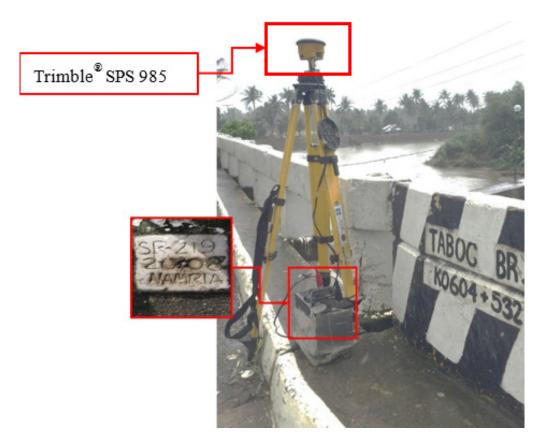
Figure 35. GNSS receiver setup, Trimble® SPS 985, at SR-219, located along the approach of Taboc Bridge in Brgy. Taboc, Municipality of Juban, Sorsogon
