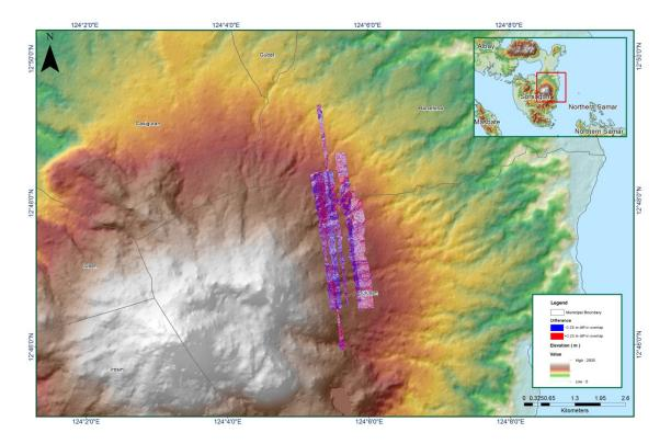
Figure 1.9.7. Elevation difference between flight lines
