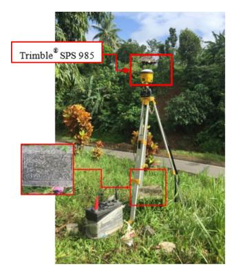
Figure 33. GNSS base set up, Trimble® SPS 985, at SRG-27, located in front of the Barangay Hall in Brgy. Bulabog, Sorsogon City, Sorsogon.
