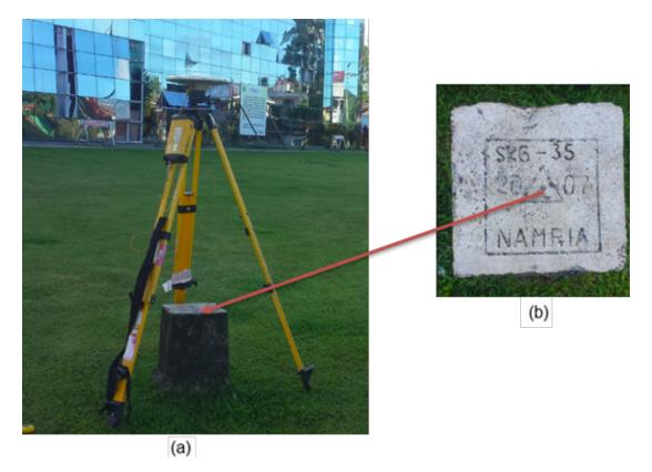
Figure 3. GPS set-up over SRG-35 as recovered in front of Casiguran Municipal Hall from the concrete fence and 13 meters from the flagpole (a) and NAMRIA reference point SRG-35 (b) as recovered by the field team.
