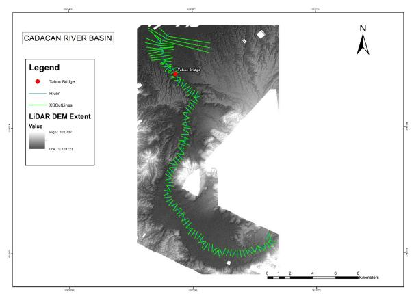
Figure 61. River cross-section of Cadacan River generated through Arcmap HEC GeoRAS tool
