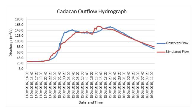
Figure 63. Outflow hydrograph of Cadacan River Basin produced by the HEC-HMS model compared with observed outflow
