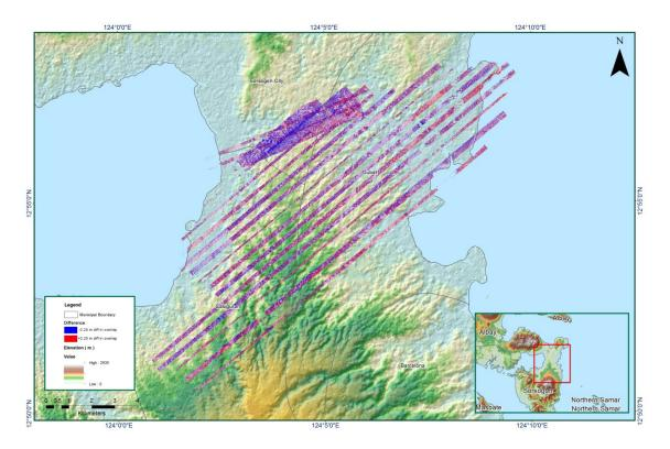
Figure 1.13.7. Elevation difference between flight lines
