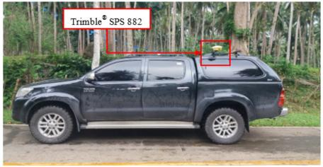
Figure 43. Validation points acquisition survey set up along Cadacan River Basin
