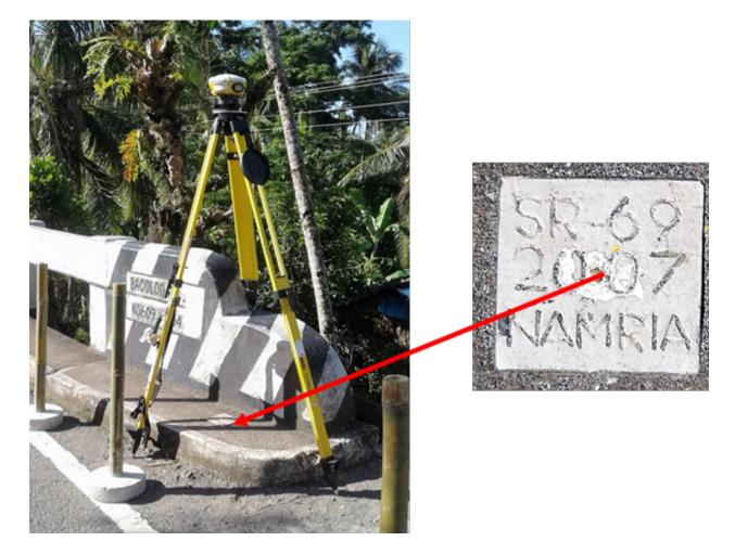
Figure 6. GPS set-up over SR-69 along Legazpi-Matnog National Road, at about 62 meters south east of KM Post 609 (a) and NAMRIA reference point SR-69 (b) as recovered by the field team.
