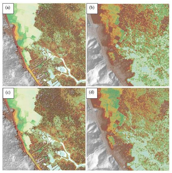
Figure 20. The production of last return DSM (a) and DTM (b), first return DSM (c) and secondary DTM (d) in some portion of Cadacan floodplain.
