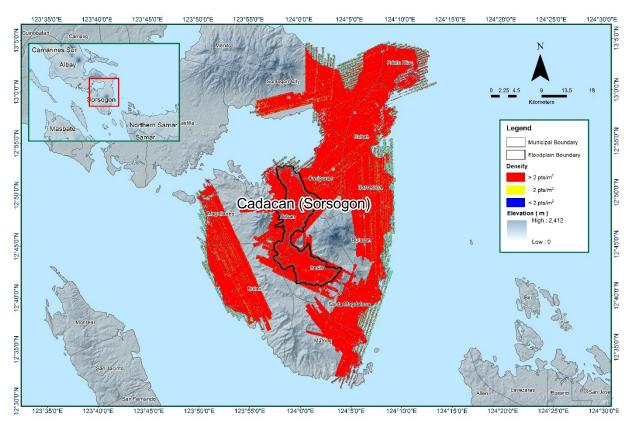
Figure 15. Pulse density map of merged LiDAR data for Cadacan floodplain.
