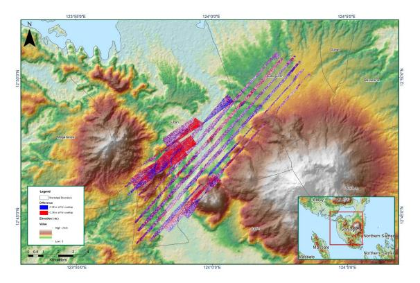
Figure 1.17.7. Elevation difference between flight lines
