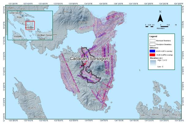
Figure 16. Elevation difference map between flight lines for Cadacan floodplain.
