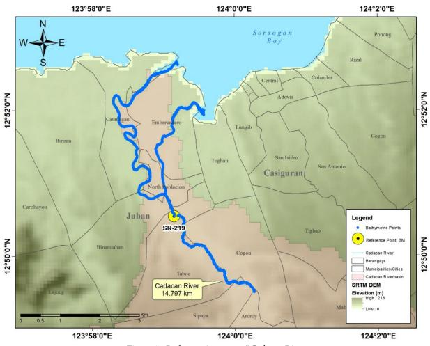
Figure 47. Bathymetric survey of Cadacan River
