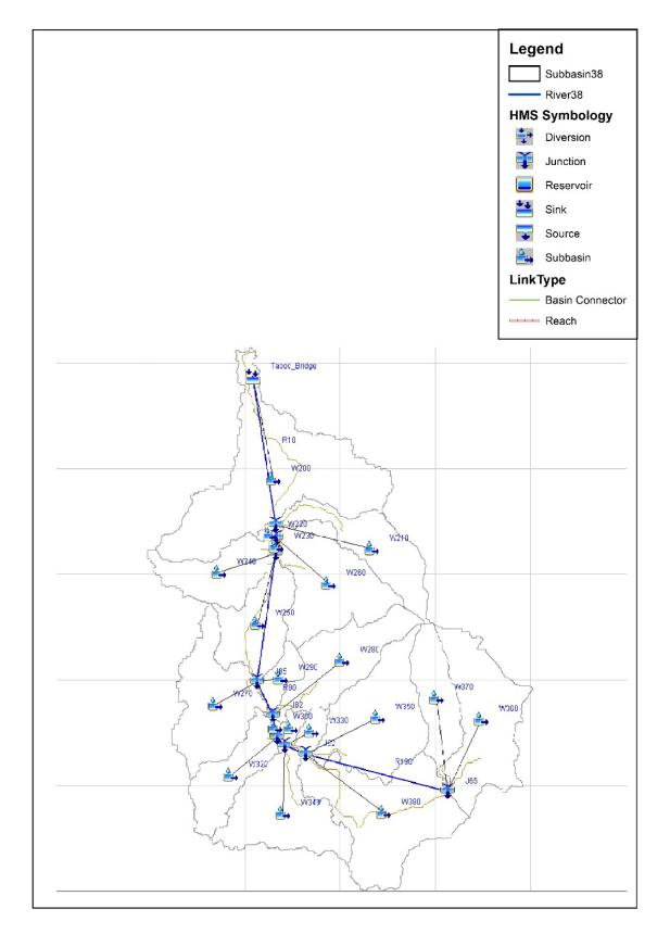
Figure 60. The Cadacan river basin model generated using HEC-HMS
