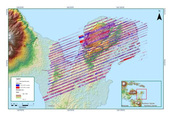
Figure 1.10.7. Elevation difference between flight lines
