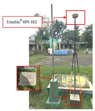
Figure 36. GNSS receiver setup, Trimble® SPS 882, at SRG-32, located inside Banuyo Elementary School in Brgy. Banuyo, Municipality of Pilar, Sorsogon.
