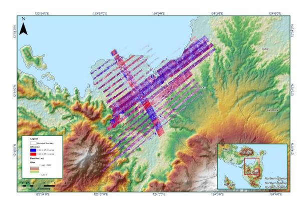
Figure 1.3.7. Elevation difference between flight lines
