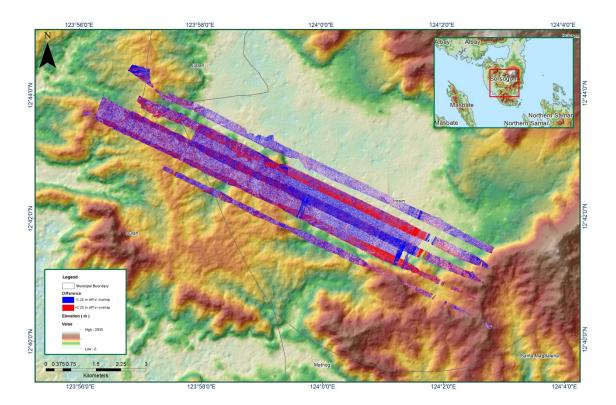
Figure 1.15.7. Elevation difference between flight lines
