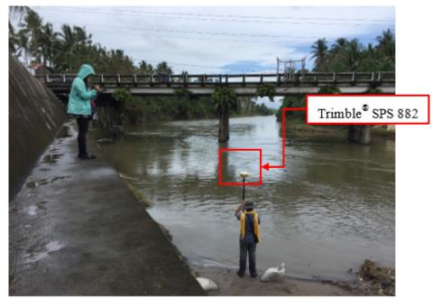
Figure 38. Bridge As-Built Survey using PPK Technique.
