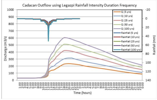
Figure 64. The outflow hydrograph at the Cadacan River Basin, generated using the simulated rain events for 24-hour period for Legazpi station
