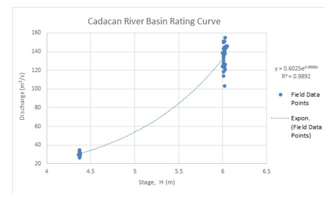
Figure 52. The rating curve of Taboc Bridge in Cadacan, Sorsogon
