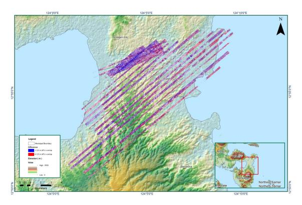
Figure 1.12.7. Elevation difference between flight lines
