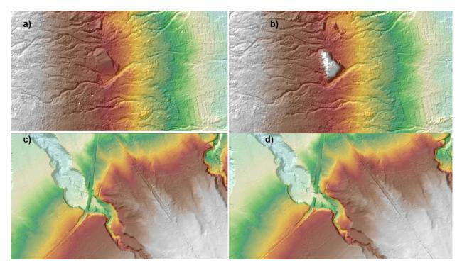
Figure 23. Portions in the DTM of Cadacan floodplain – a hilltop before (a) and after (b) data retrieval; a bridge before (c) and after (d) manual editing
