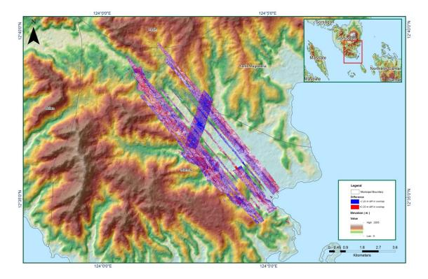
Figure 1.7.7. Elevation difference between flight lines
