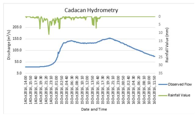
Figure 53. Rainfall and outflow data of the Cadacan River Basin, which was used for modeling
