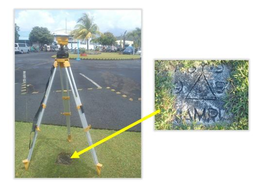
Figure 4. GPS set-up over ABY-9 inside Legaspi Airport Compound 52.0 meters SE of Legaspi Airport Flagpole, 35 meters NE of Legaspi Airport Welcome Post 3.30 meters NW of Lamp (a) and NAMRIA reference point ABY-9 (b) as recovered by the field team.
