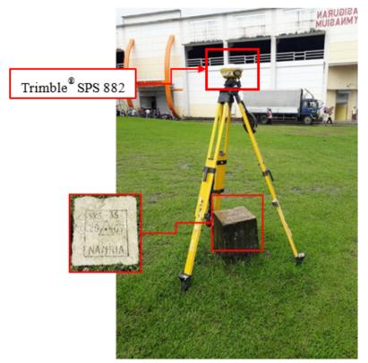
Figure 34. GNSS receiver setup, Trimble® SPS 882, at SRG-35, located in front of the Casiguran Municipall Hall in Brgy. Central, Municipality of Casiguran, Sorsogon.
