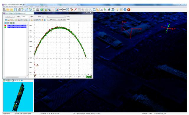
Figure 17. Quality checking for a Cadacan flight 3887G using the Profile Tool of QT Modeler.
