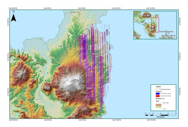
Figure 1.11.7. Elevation difference between flight lines
