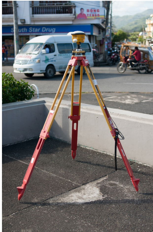
Figure 5. GPS set-up over established control point VIRAC-E0 at Barangay Palta Small, Virac Catanduanes.
