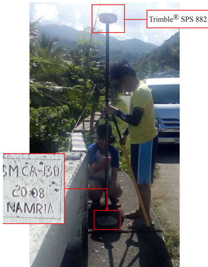
Figure 32. GNSS base set up, Trimble® SPS 882, at CA-130, located at the end of pathwalk in Brgy. Balatohan, Municipality of San Miguel, Catanduanes
