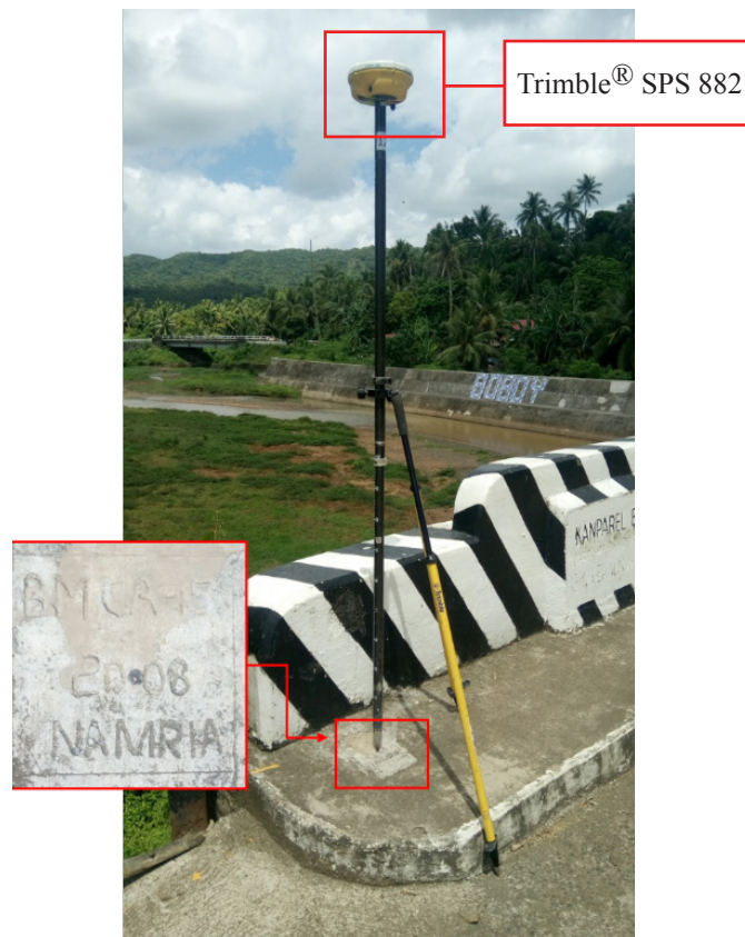
Figure 33. GNSS base set up, Trimble® SPS 882, at CA-15, is located at the approach of the left side of Kanparel Bridge in Brgy. Santa Maria, Municipality of Panganiban, Catanduanes
