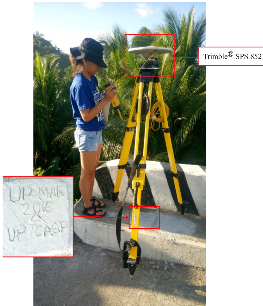
Figure 36. GNSS base set up, Trimble® SPS 852, at UP-MAR, located at the approach of the right side of Marcos Bridge in Brgy. Bigaa, Municipality of Virac, Catanduanes
