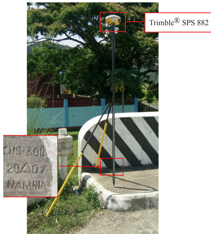
Figure 34. GNSS base set up, Trimble® SPS 882, at CNS-3018, located at the approach of Pilot Bridge along Catanduanes Circumferential Road in Brgy. San Isidro, Municipality of Viga, Catanduanes
