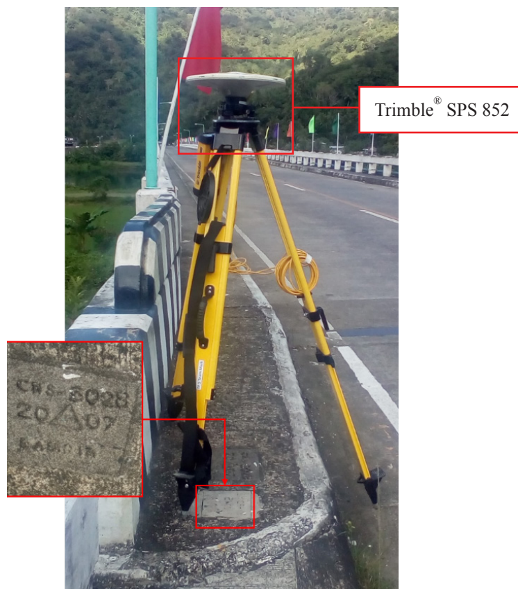
Figure 35. GNSS base set up, Trimble® SPS 852, at CNS-3028, located at the approach of Bato Bridge along Catanduanes Circumferential Road in Brgy. Tilis, Municipality of Bato, Province of Catanduanes
