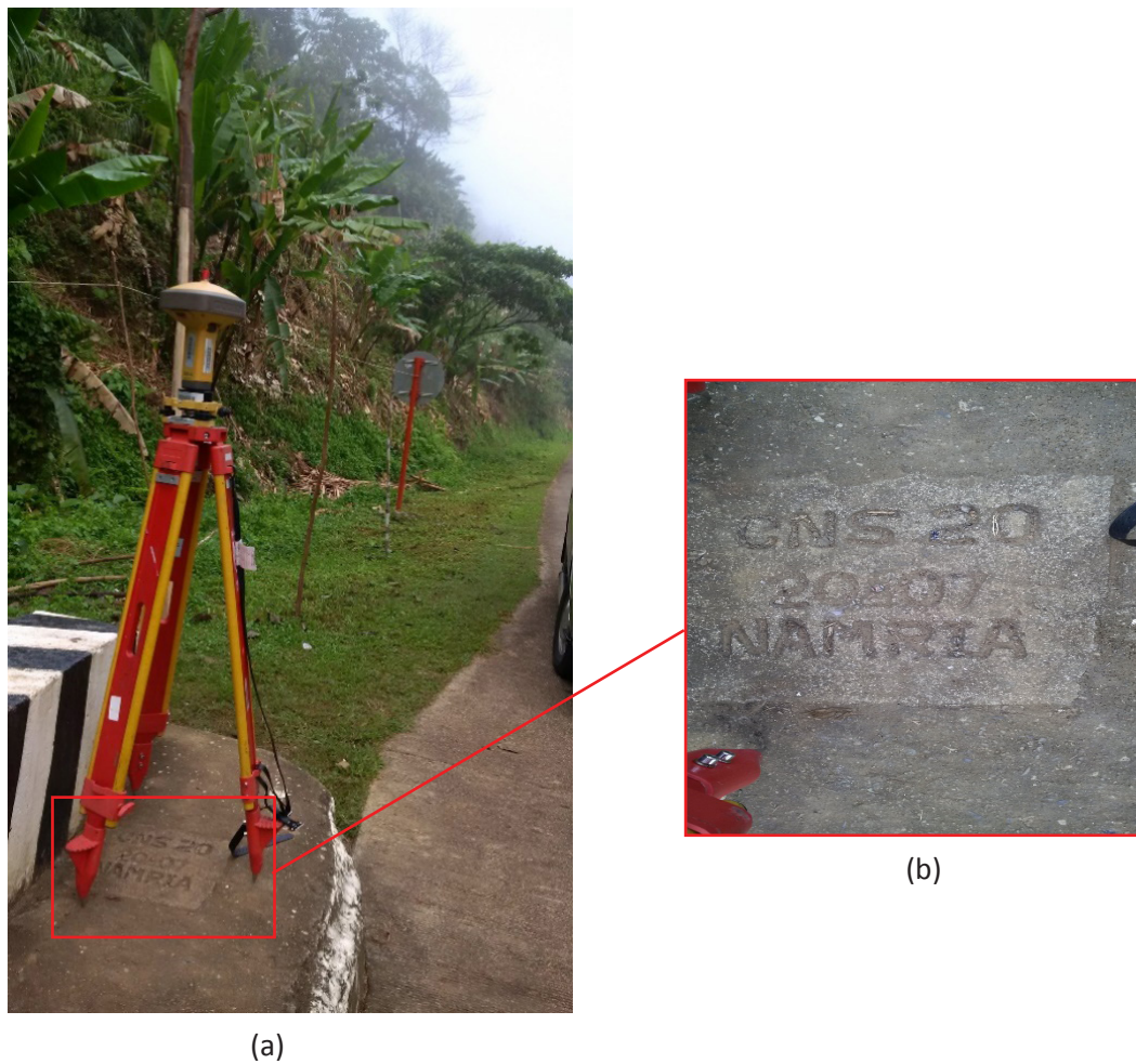
Figure 4. GPS set-up over CNS-20 located at Malmag bridge along circumferential road at Barangay Pagsangahan (a) and NAMRIA reference point CNS-20 (b) as recovered by the field team.
