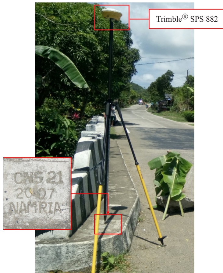
Figure 31. GNSS base set up, Trimble® SPS 882, at CNS-21, located at Palta Bridge in Brgy. Palta Small, Municipality of Virac, Catanduanes
