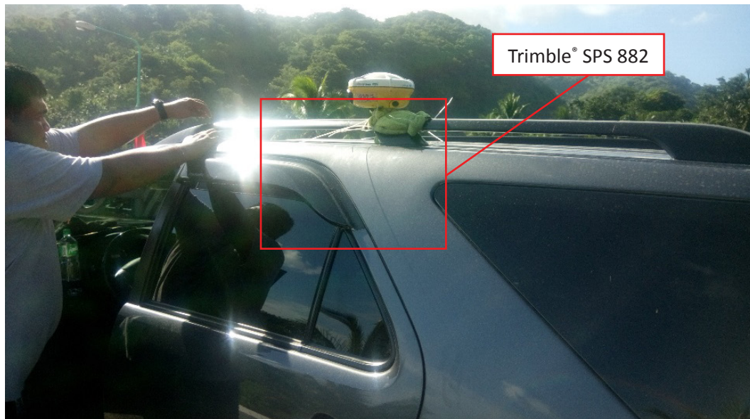
Figure 41. Validation points acquisition survey set up
