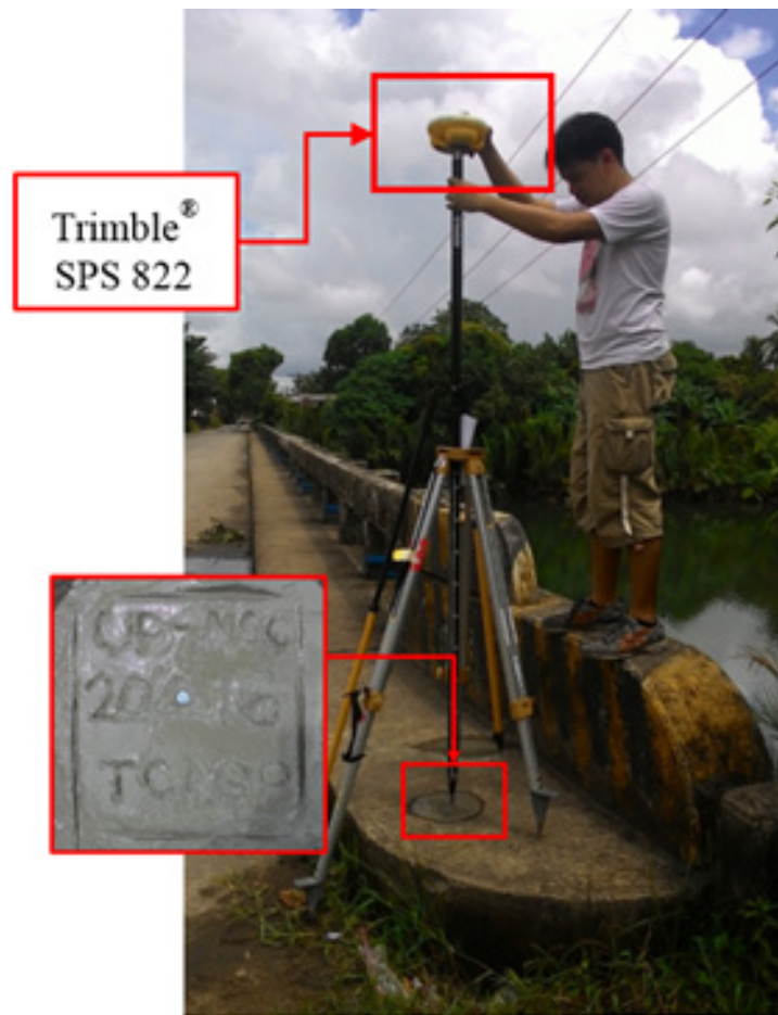
Figure 35. GNSS receiver setup, Trimble® SPS 822, at UP-MOC, located at the approach of Mocong Bridge in Brgy. Mocong, Municipality of Basud, Camarines Norte
