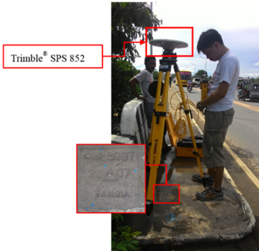
Figure 34. GNSS receiver setup, Trimble® SPS 852, at CMN-3087, located at the approach of Labo Bridge in Brgy. Bakiad, Municipality of Labo, Camarines Norte
