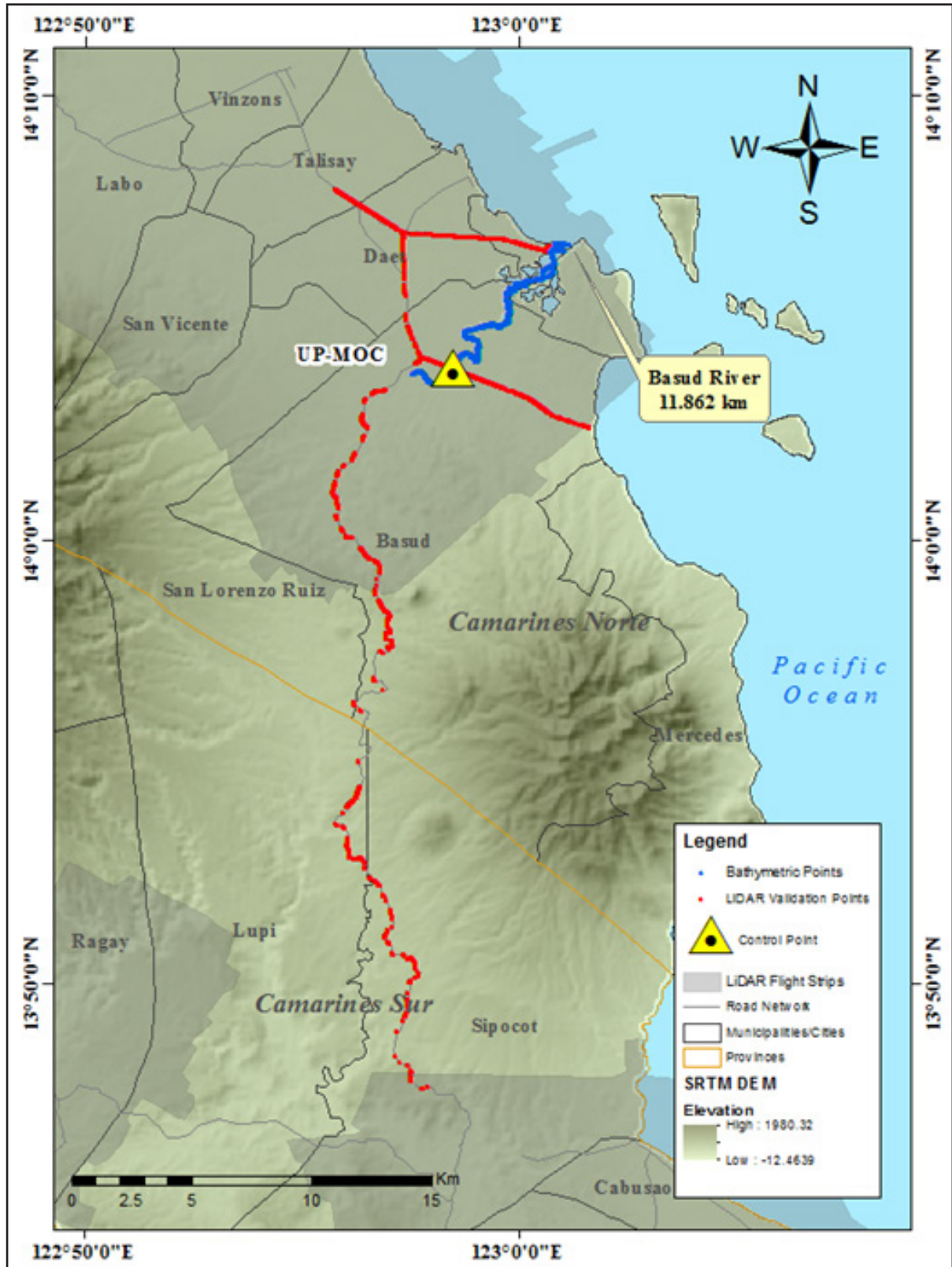
Figure 43. Validation point acquisition survey of Basud River basin
