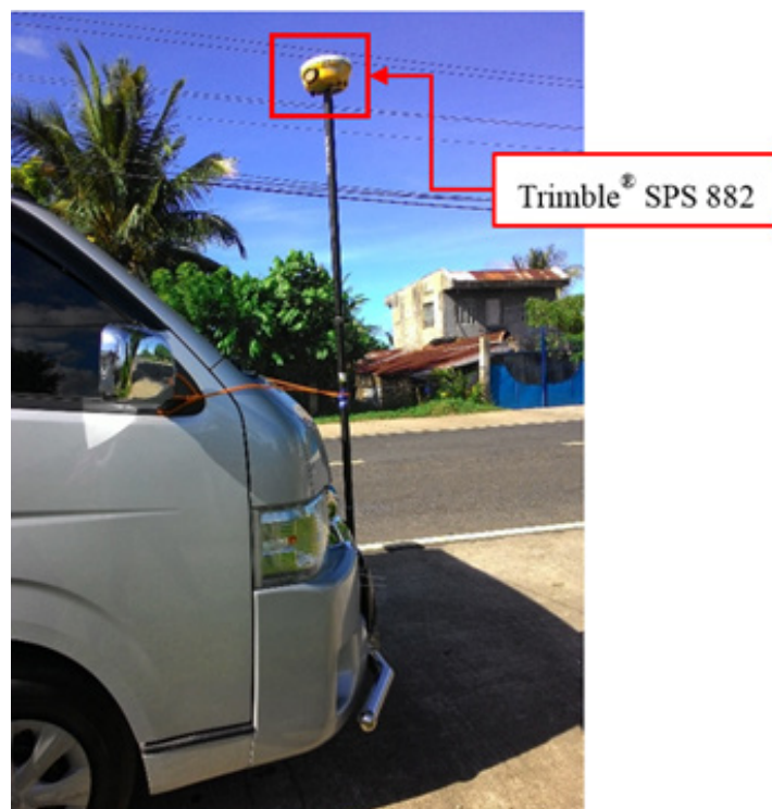
Figure 49. The validation point acquisition survey setup using a GNSS receiver fixed in a van along the Silaga River Basin
