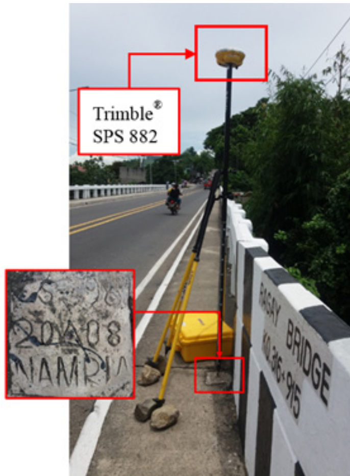
Figure 33. GNSS receiver setup, Trimble® SPS 882, at CS-398, located at the approach of Ragay Bridge in Brgy. Pangitayan, Municipality of Ragay, Camarines Sur
