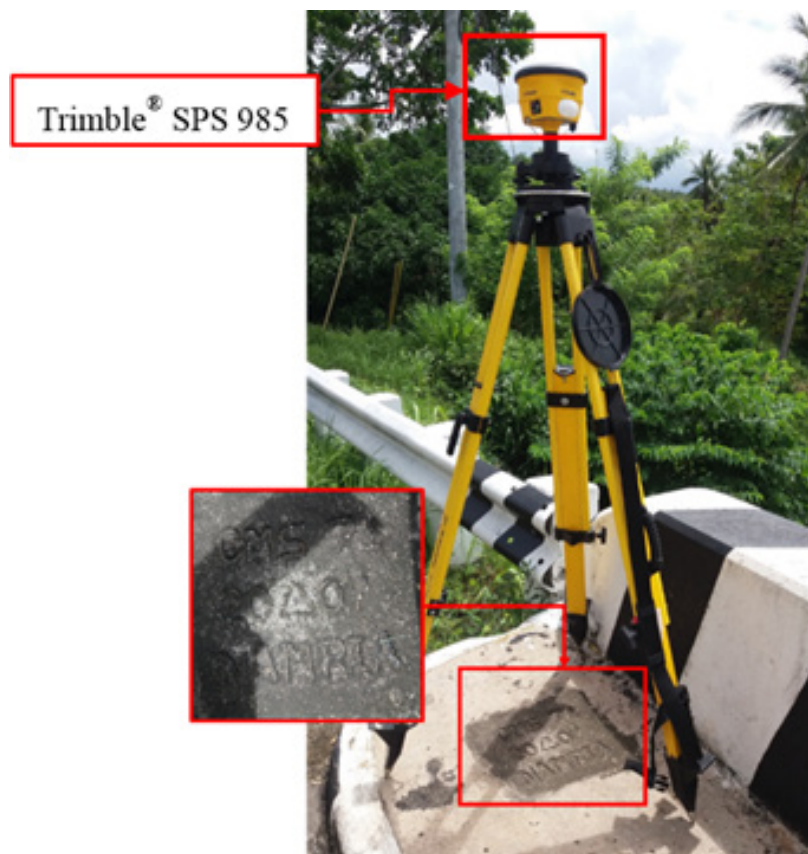
Figure 32. GNSS base set up, Trimble® SPS 985, at CMS-71, situated at the approach of Kilbay Bridge in Brgy. Cabasag, Municipality of Del Gallego, Camarines Sur
