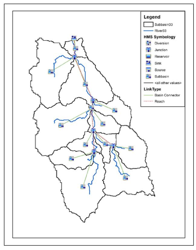
Figure 64. The Baleno river basin model generated using HEC-HMS
