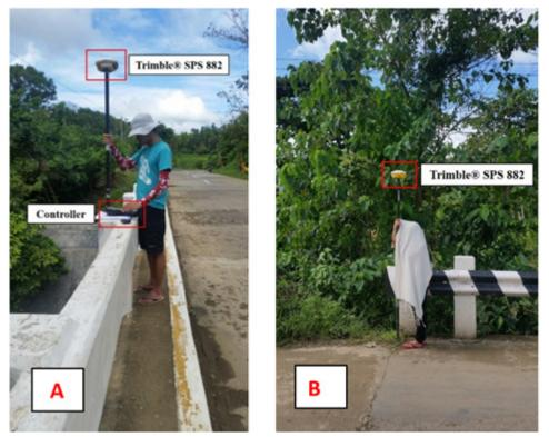
Figure 39. Setup during the Bridge As-built measurement in A) Cancahorao and B) Gangao Bridge
