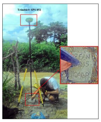
Figure 38. GNSS receiver setup, Trimble® SPS 882, at UP-GAN, located on the top of a riprap near Gangao Bridge, along Central Nautical Highway, Brgy. Gangao, Baleno, Masbate
