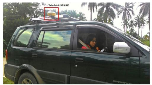
Figure 47. Validation points acquisition survey setup: A Trimble® SPS 882, mounted on top of the vehicle
