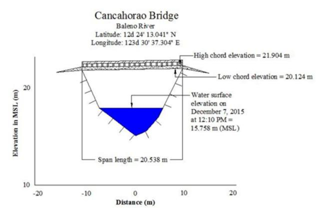
Figure 41. Cancahorao Bridge cross-section diagram
