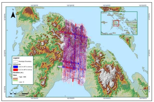
Figure A-8.7. Elevation difference between flight lines
