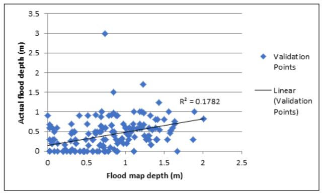
Figure 83. Flood map depth vs. Actual flood depth
