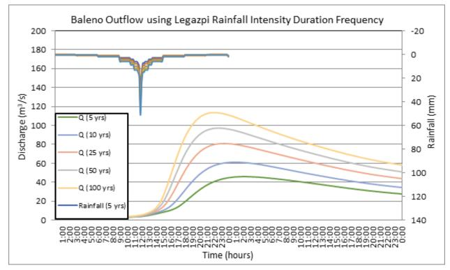
Figure 68. The outflow hydrograph at the Baleno River Basin, generated using the simulated events for 24-hour period for Legazpi station
