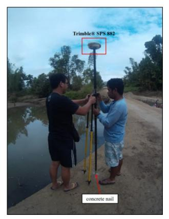
Figure 36. Trimble® SPS 882 setup at UP-ALA, located at Alas Bridge in Brgy. Alas, Mandaon, Masbate
