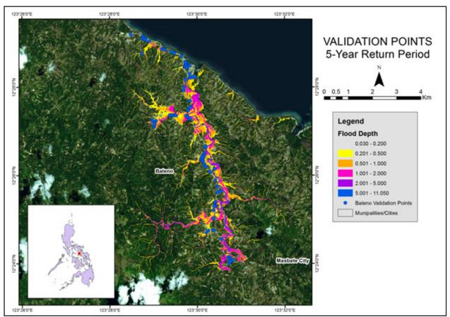
Figure 82. The validation points for the 5-Year flood depth map of the Baleno flood plain
