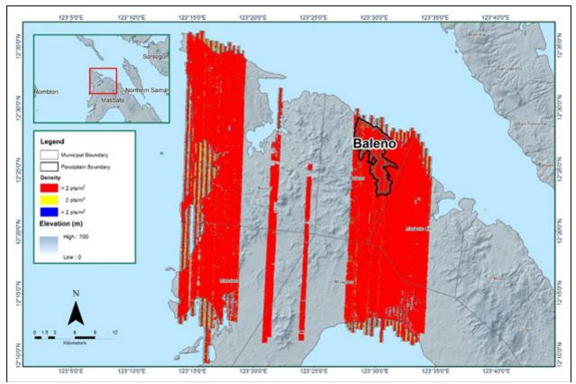
Figure 15. Pulse density map of merged LiDAR data for Baleno floodplain.
