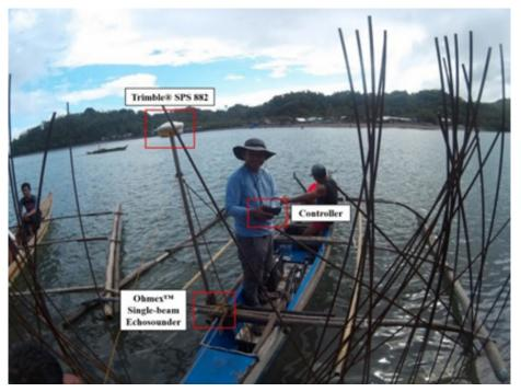
Figure 50. Setup of Trimble® SPS 882 receiver and Ohmex<sup>™</sup> single-beam echosounder in a boat for the bathymetric survey in Baleno River
