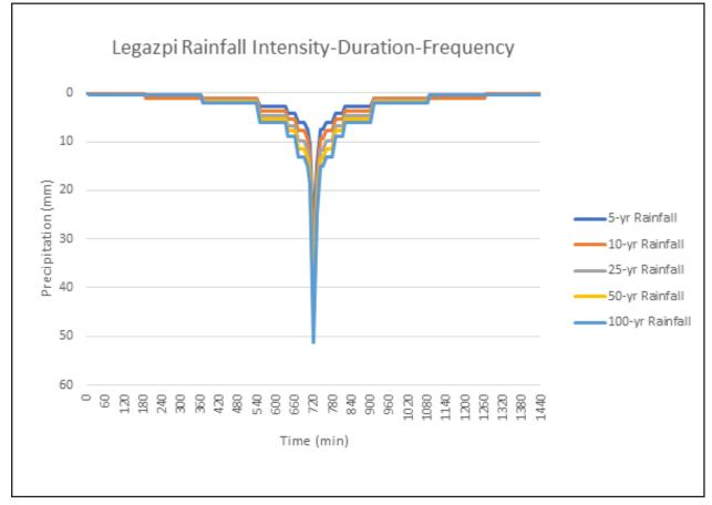
Figure 59. The synthetic storm generated for a 24-hour period rainfall for various return periods
