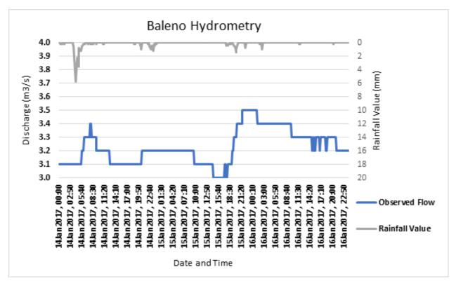
Figure 57. Rainfall and outflow data of the Baleno River Basin, which was used for modeling
