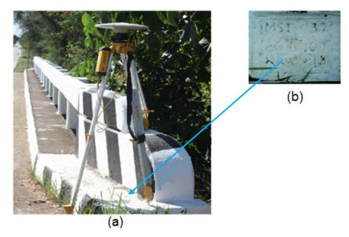
Figure 4. GPS set-up over MST-31 in Boracay Bridge, Barangay Bangad, municipality of Milagros, Masbate (a) and NAMRIA reference point MST-31 (b) as recovered by the field team.
