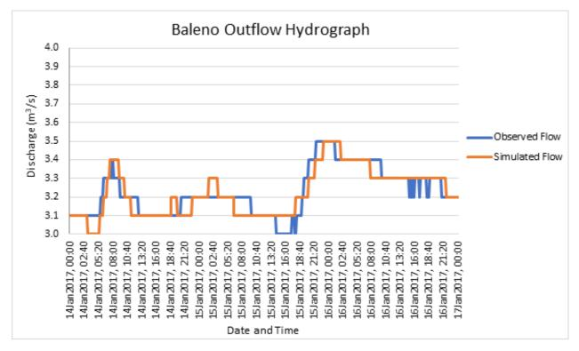
Figure 67. Outflow hydrograph of Baleno River Basin produced by the HEC-HMS model compared with observed outflow
