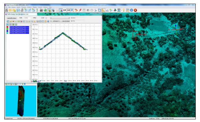
Figure 17. Quality checking for a Baleno flight 1307P using the Profile Tool of QT Modeler.
