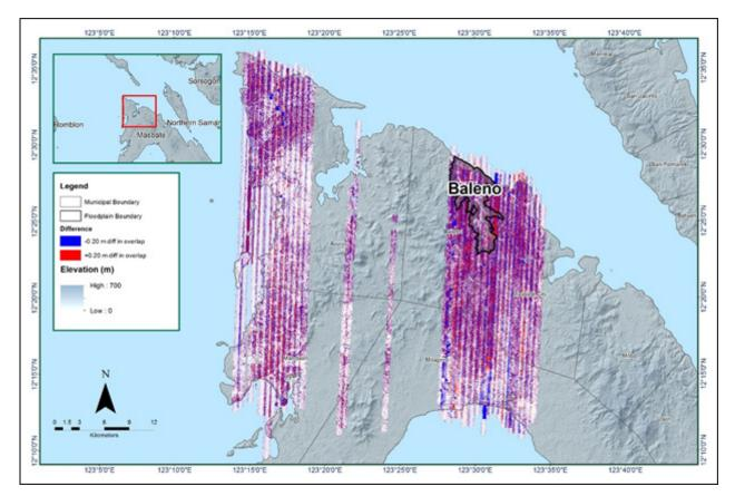
Figure 16. Elevation difference map between flight lines for Baleno floodplain.
