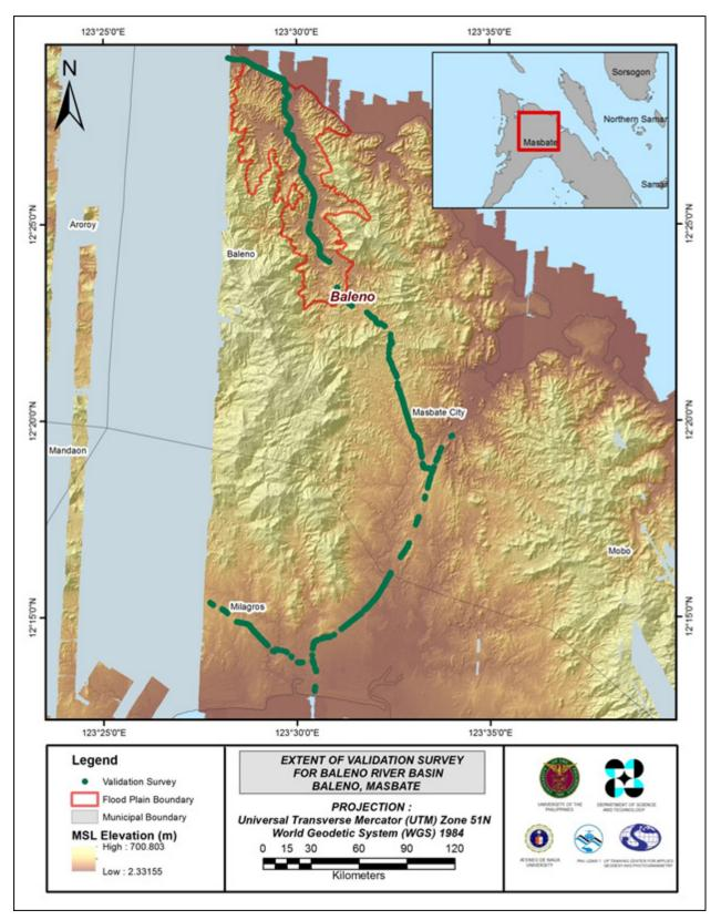
Figure 25. Map of Baleno Flood Plain with validation survey points in green.
