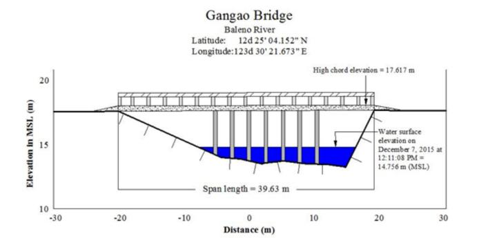
Figure 43. Bridge as-built and cross-sectional diagram of Baleno River at Gangao Bridge, Brgy. Gangao, Municipality of Baleno, Masbate
