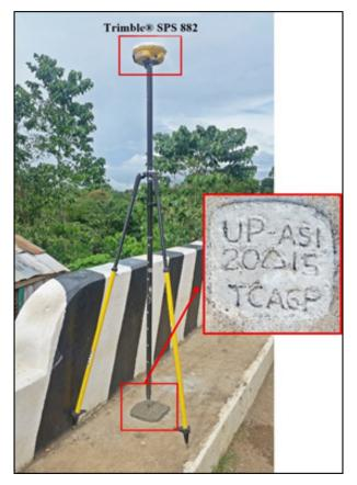
Figure 37. GNSS receiver setup, Trimble® SPS 882, at UP-ASI, at Asid Bridge, along Central Nautical Highway, Brgy. Asid, Masbate City
