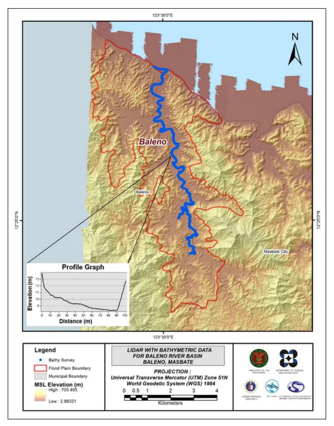
Figure 28. Map of Baleno Flood Plain with bathymetric survey points shown in blue.
