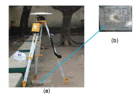
Figure 5. GPS set-up over MST-32 inside the compound of the Milagros Municipal Hall, Masbate (a) and NAMRIA reference point MST-32 (b) as recovered by the field team.
