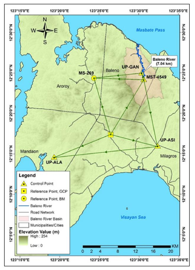
Figure 32. GNSS Network occupied in Baleno River Basin field survey
