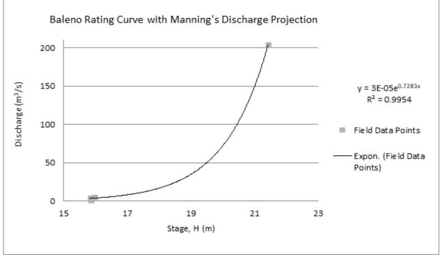
Figure 56. The rating curve of Cancahorao Bridge in Baleno, Masbate
