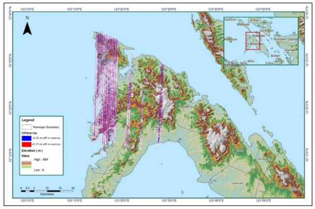
Figure A-8.14. Elevation difference between flight lines
