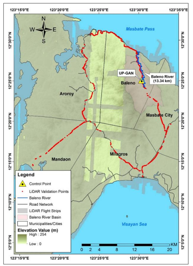
Figure 48. Points gathered during the LiDAR Ground Validation Survey for Baleno River Basin
